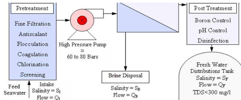
Fig. 2. A typical reverse osmosis seawater desalination plant scheme showing input/output and different stages of treatment. Note that boron control involves a second RO stage (BWRO), which also produces brine with a low TDS (< 3000 mg/l).
