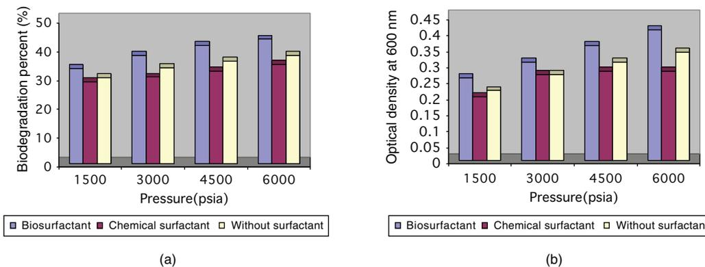
Fig. 8. Effect of pressure on (a) percentage of biodegradation and (b) growth of the strain ERCPP1-1 ( $T = 40\text{ }^{\circ}\text{C}$ , salinity =  $0.1\%$ ,  $\text{pH} = 7.0$ , heavy crude oil concentration =  $0.5\%$ , rotation =  $150\text{ rpm}$ ).
