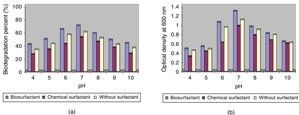
Fig. 6. Effect of pH on (a) percentage of biodegradation and (b) growth of the strain ERCPPI-1 ( $T = 40^\circ\text{C}$ , salinity = 0.1%,  $P = 14.7$  psia, heavy crude oil concentration = 0.5%, rotation = 150 rpm).
