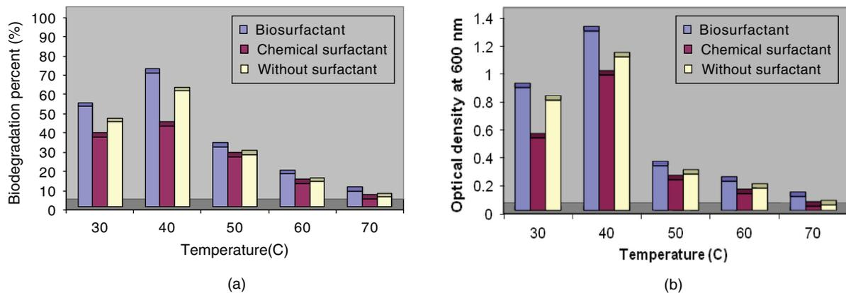
Fig. 5. Effect of temperature on (a) percentage of biodegradation and (b) growth of the strain ERCPPI-1 (pH = 7.0, salinity = 0.1%,  $P = 14.7$  psia, heavy crude oil concentration = 0.5%, rotation = 150 rpm).
