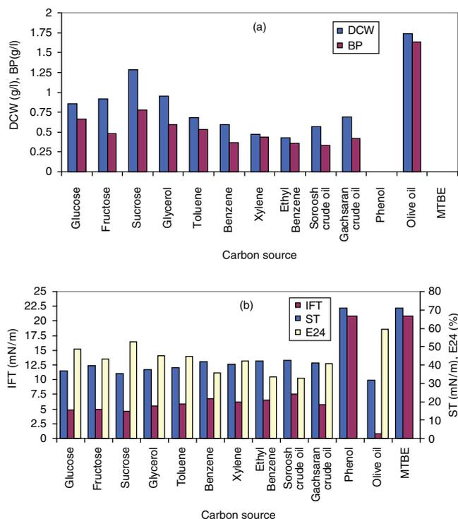
Fig. 3. Effect of various carbon sources on (a) growth and biosurfactant production of the strain ERCPPI-1, (b) surface activity of biosurfactant produced by strain ERCPPI-1 ( $T = 40$  °C, salinity=0.1%,  $P = 14.7$  psia, pH = 7.0, carbon source concentration = 1.0%, rotation = 150 rpm).
