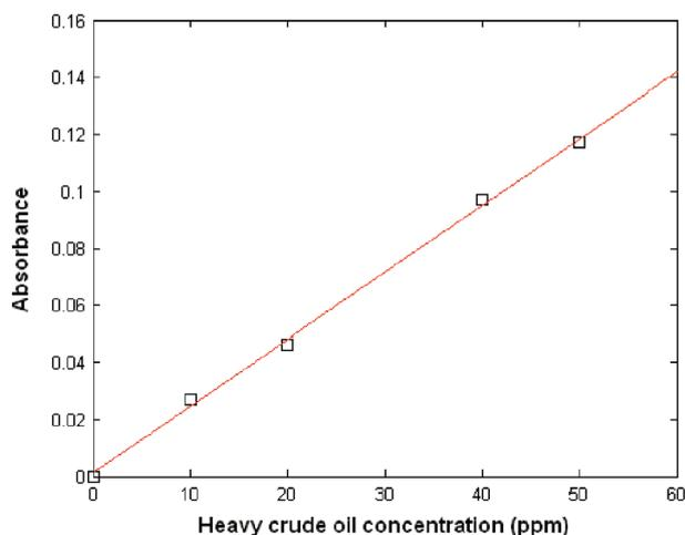
Fig. 1. Calibration curve for determining petroleum hydrocarbon content.
