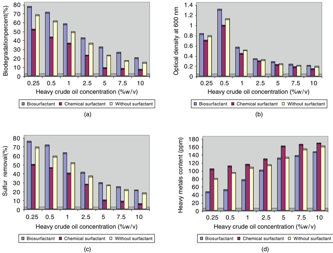
Fig. 4. Effect of heavy crude oil concentration on (a) percentage of biodegradation and (b) growth of the strain ERCPPI-1, (c) percentage of sulfur removal and (d) heavy metals content of Soroosh heavy crude oil ( $T = 40\text{ }^{\circ}\text{C}$ , salinity = 0.1%,  $P = 14.7$  psia, pH = 7.0, rotation = 150 rpm).
