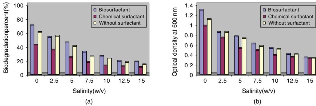
Fig. 7. Effect of salinity on (a) percentage of biodegradation and (b) growth of the strain ERCPP1-1 ( $T = 40\text{ }^{\circ}\text{C}$ ,  $\text{pH} = 7.0$ ,  $P = 14.7\text{ psia}$ , heavy crude oil concentration =  $0.5\%$ , rotation =  $150\text{ rpm}$ ).
