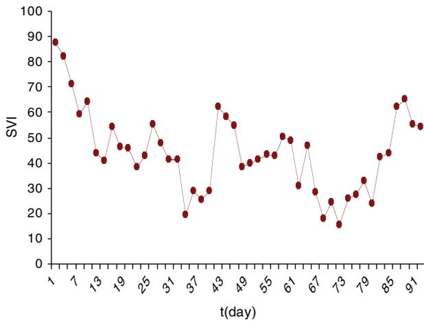
Fig. 3. Temporal variation of SVI in bioreactor during the experiment.
