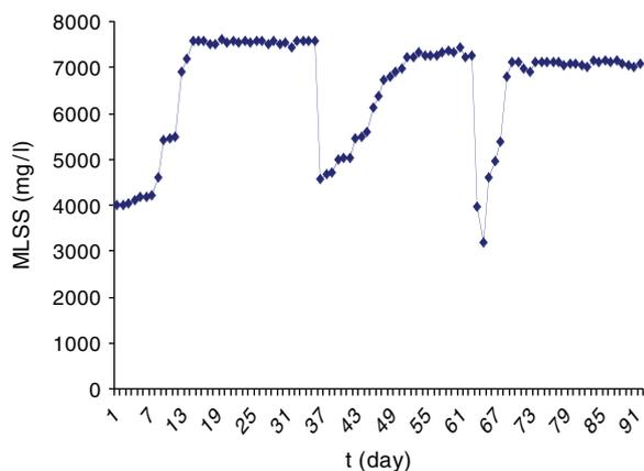
Fig. 1. Profile of MLSS in bioreactor during the experiment.
