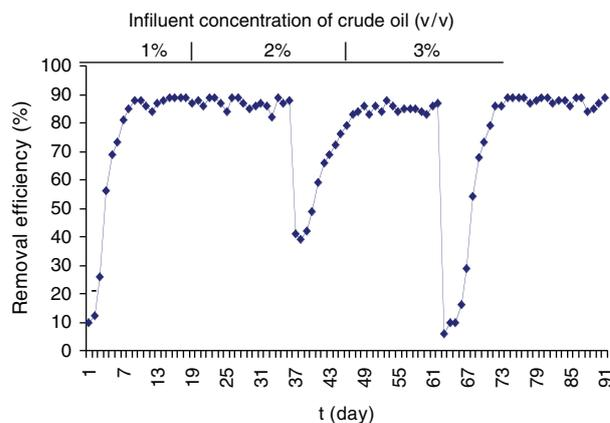
Fig. 2. Profile of crude oil removal efficiencies during the experiment.
