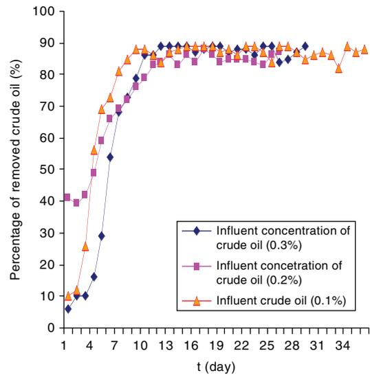
Fig. 4. Relationship between incubation time and removal percentage of crude oil at different concentrations of crude oil.
