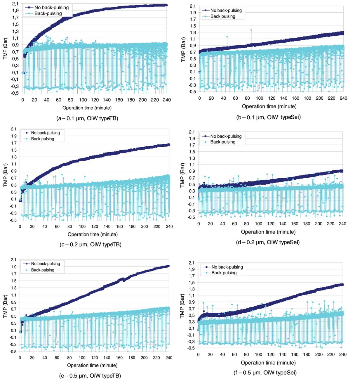
Fig. 6. *a,b,c,d,e,f*: Effect of different oil types (TB, Sei) with concentration 350 ppm on different membrane pore sizes with surfactant (450 ppm), without particles, with and without back-pulsing at flux  $500 \text{ l.m}^{-2}.\text{hr}^{-1}$ .
