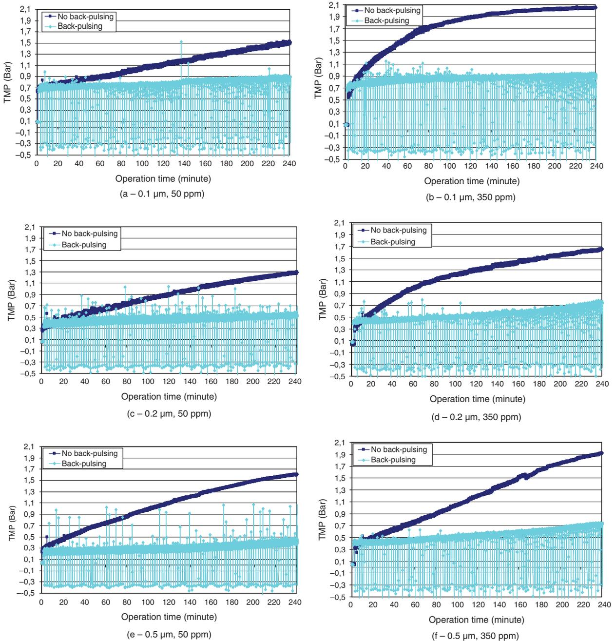
Fig. 5. *a,b,c,d,e,f*: Effect of oil concentration (50, 350 ppm) of oil type-TB on different membrane pore sizes with surfactant (450 ppm), without particles, with and without back-pulsing at flux  $500 \text{ l.m}^{-2}.\text{hr}^{-1}$ .
