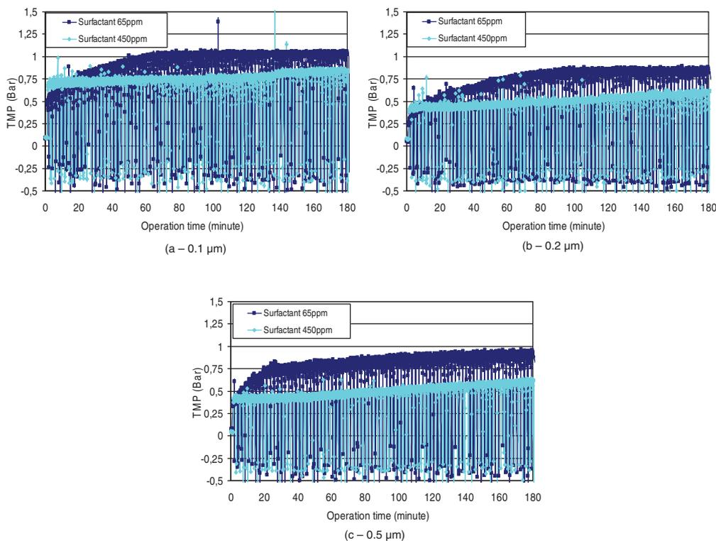
Fig. 4. *a, b, c*: Effect of surfactant concentration (65, 450 ppm) on different membrane pore sizes for oil type-TB (50 ppm), with particles, with back-pulsing at flux  $500 \text{ l.m}^{-2}.\text{hr}^{-1}$ .
