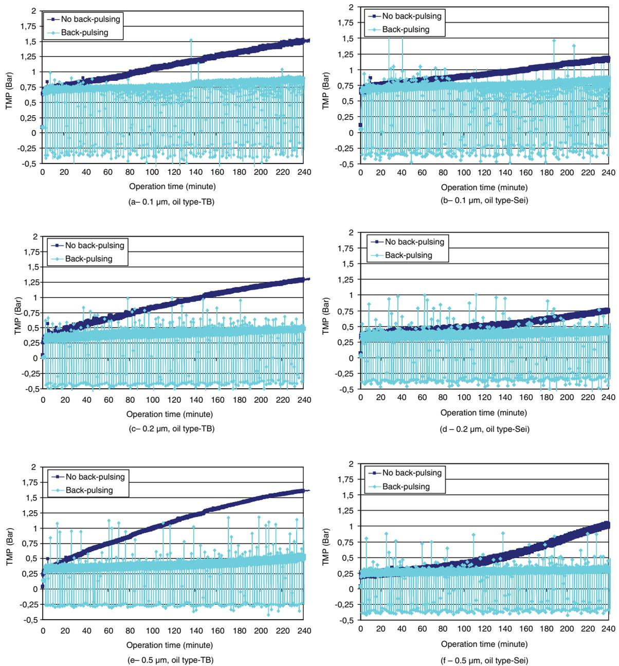
Fig. 2. *a,b,c,d,e,f*: Effect with and without back-pulsing on oil type-TB and oil type-Sei with concentration 50 ppm on different membrane pore sizes, with surfactant (450 ppm), without particles at flux 500 l.m<sup>-2</sup>hr<sup>-1</sup>.
