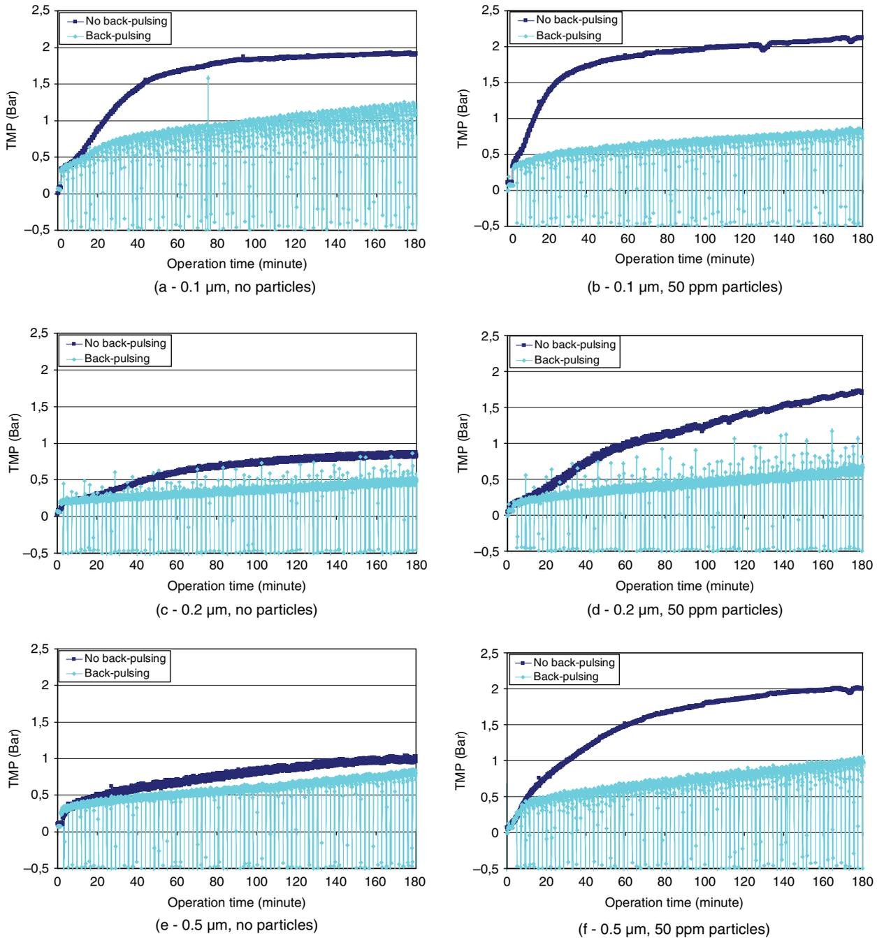
Fig. 7. *a,b,c,d,e,f*: Effect of particles (0, 50 ppm) of oil type-TB (150 ppm) on different membrane pore sizes with surfactant (65 ppm), with and without back-pulsing at flux  $250 \text{ L}\cdot\text{m}^{-2}\cdot\text{hr}^{-1}$ .
