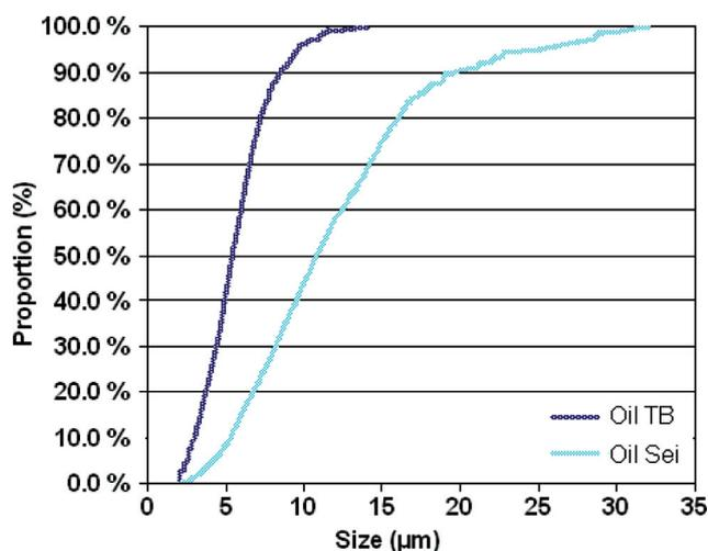
Fig. 3. Droplet size distribution (volume) of oil-TB and oil-Sei at 50 ppm oil in water with 450 ppm of surfactant concentration.
