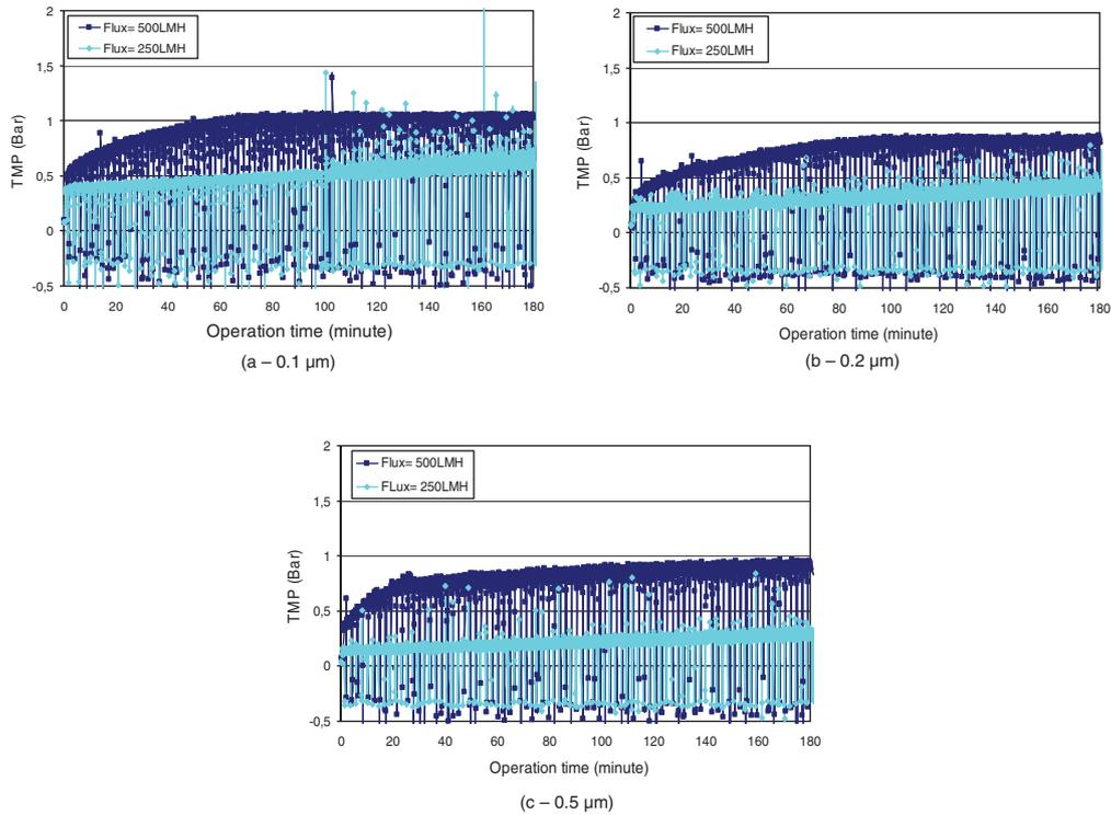
Fig. 8. *a,b,c*: Effect of different fluxes (250, 500  $\text{l.m}^{-2}.\text{hr}^{-1}$ ) on different membrane pore sizes for oil type-TB (50 ppm), with surfactant (65 ppm), without particles, with back-pulsing.
