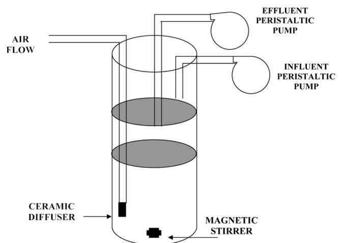
Fig. 1. Schematic diagram of lab-scale sequencing batch reactors (SBR).
