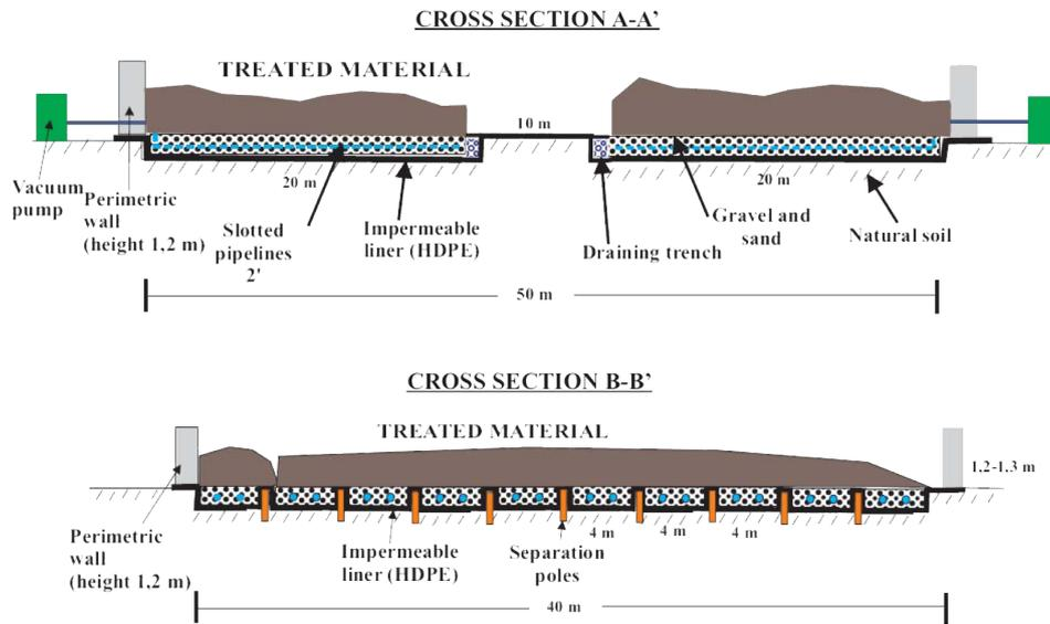
Fig. 1. Cross sections drawings of the bioremediation treatment area.
