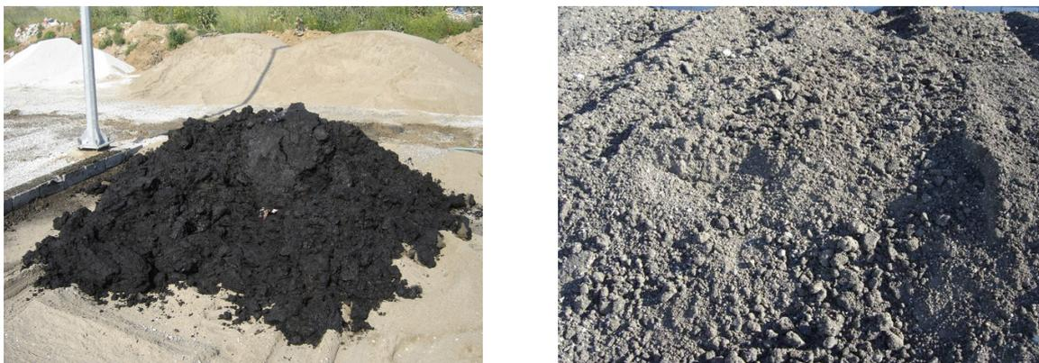
Fig. 2. Solid residual material (SRM) prior (left) and after (right) bioremediation treatment.
