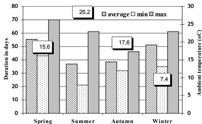
Fig. 3. Duration of bioremediation process vs. year periods (ambient temperature values in labels).
