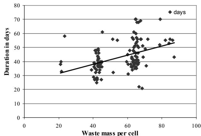
Fig. 4. Duration of bioremediation process vs. waste mass per cell.
