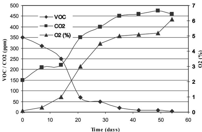
Fig. 6. Monitoring results of biotreatment process – gaseous emissions measurements (biotreatment period 05/01/07–28/2/07).
