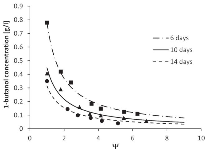
Fig. 9. Influence of  $\Psi$  on 1-butanol concentration in outlet stream. Line – the model calculations, points – experimental data.
