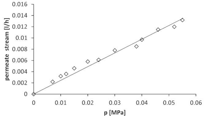
Fig. 7. Characteristic of the membrane module with polysulfone capillaries ( $A = 0.0126 \text{ m}^2$ ).
