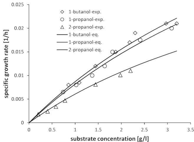
Fig. 5. Kinetics of 1-butanol, 1-propanol and 2-propanol biodegradation (points – experimental data from the continuous processes, line – the curve drawn on the basis of the kinetic constants).
