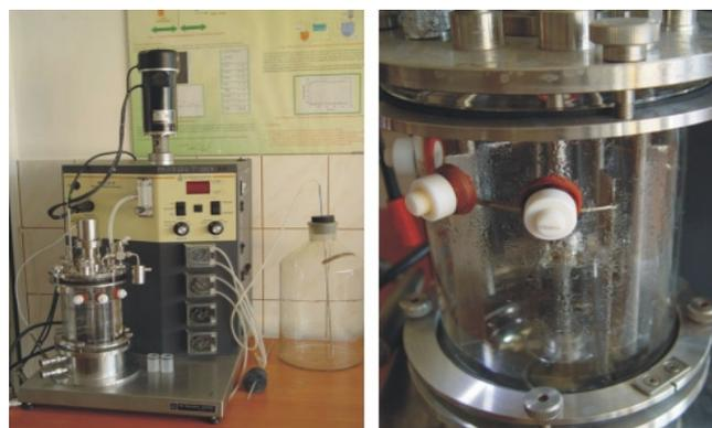
Fig. 1. Bioreactor BioFlo (New Brunswick) used in the experiments.
