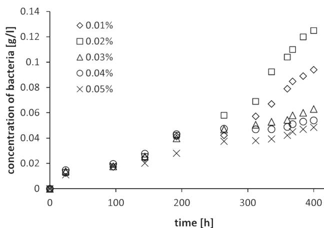
Fig. 3. Influence of concentration of  $H_2O_2$  on *P. fluorescens* growth ( $c_{0(1\text{-butanol})} = 2.2 \text{ g l}^{-1}$ ).
