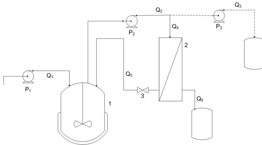
Fig. 2. Scheme of the membrane bioreactor — (1) bioreactor, (2) membrane module, (3) pressure-reducing valve,  $P_1$ ,  $P_2$ ,  $P_3$  — pumps.
