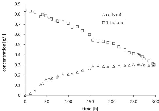
Fig. 4. Run of the batch process at  $c_{0(1-butanol)} = 0.84 \text{ g l}^{-1}$ .
