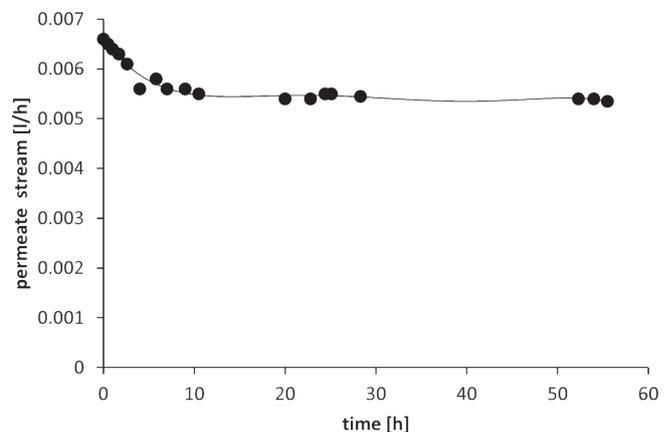
Fig. 8. Change of the permeate stream during circulation of bacteria ( $\Delta P = 0.024 \text{ MPa}$ ,  $V_{reactor} = 2.7 \text{ l}$ ,  $X = 1.14 \text{ g l}^{-1}$ ).
