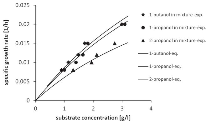
Fig. 6. Kinetics of the mixture alcohols biodegradation (points – experimental data from the continuous processes on alcohol mixtures, line – the curve drawn on the basis of the kinetic constants).
