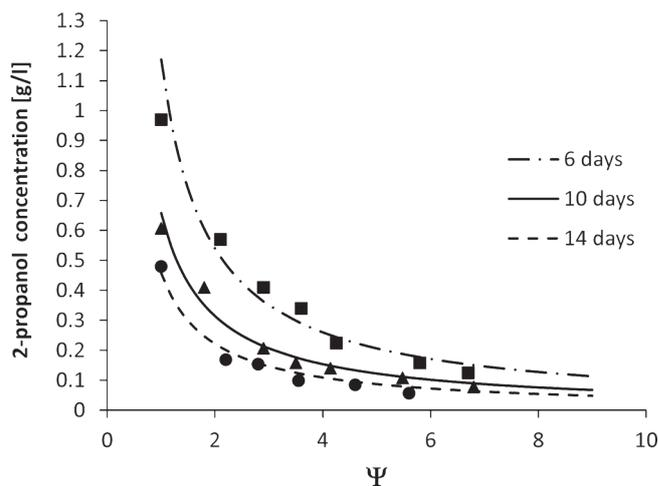
Fig. 10. Influence of  $\Psi$  on 2-propanol concentration in outlet stream. Line – the model calculations, points – experimental data.
