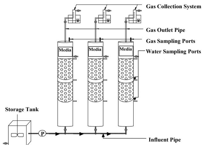
Fig. 1. Experimental set-up of upflow anaerobic floating filter (UAFF).
