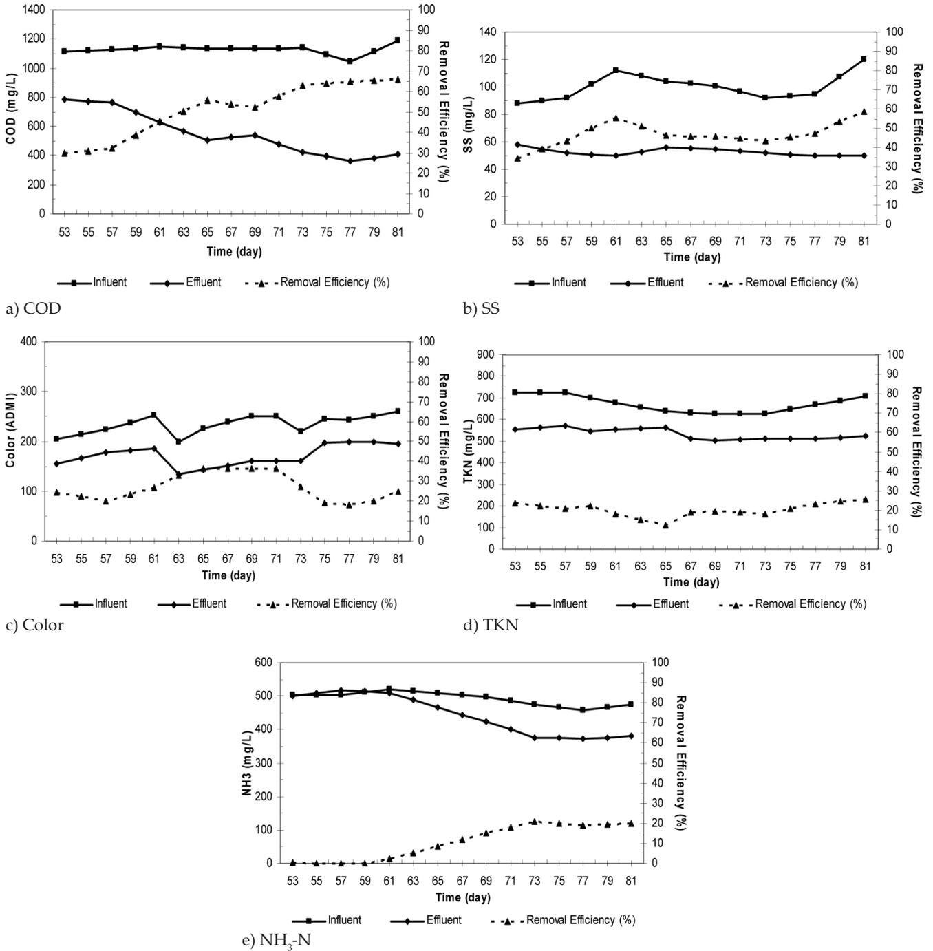
Fig. 2. Performance of CP followed by UAFF process at various water quality parameters.
