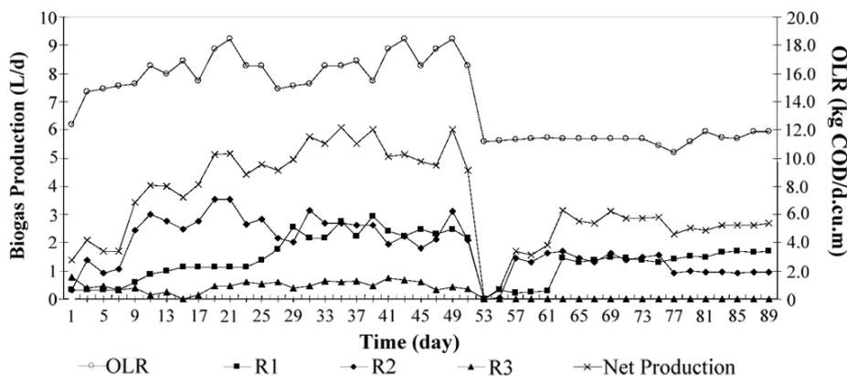
Fig. 4. Variations of OLR and biogas production (R1: the first reactor, R2: the second reactor, R3: the third reactor).
