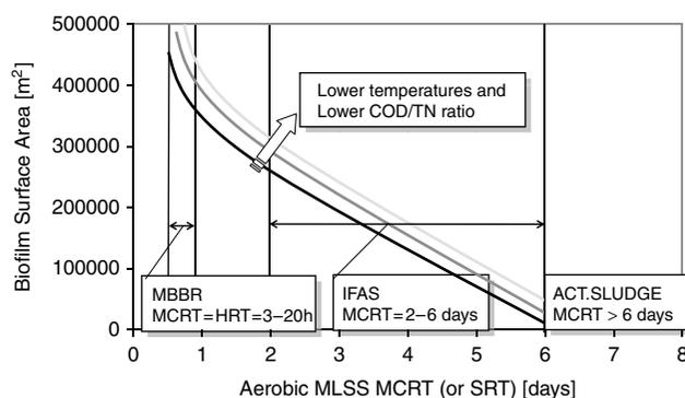
Fig. 1. Threshold of required biofilm surface area for reaching full nitrification for typical municipal wastewater as a function of MCRT (SRT) – adapted from [7].
