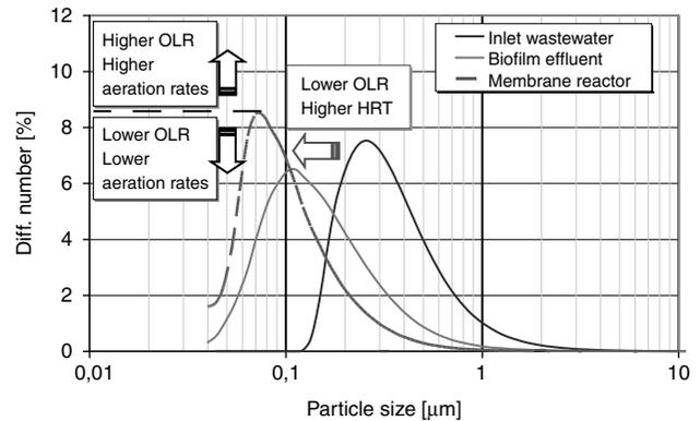
Fig. 3. Fate of submicron particles in pBF-MBR in different stages of process – adapted from [38].
