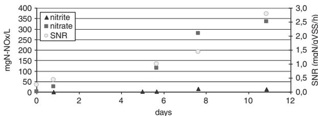
Fig. 3. Lab-scale batch growth of nitrifer species at pH 7.
