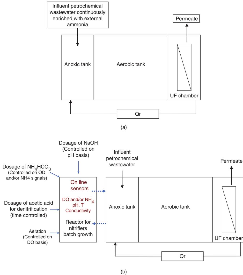
Fig. 1. (a) MBR continuously-fed scenario; (b) MBR with cyclic batch enrichment of nitrifiers scenario.
