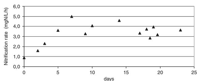
Fig. 6. Pilot scale batch growth of nitrifiers on a substrate of ammonia bicarbonate.
