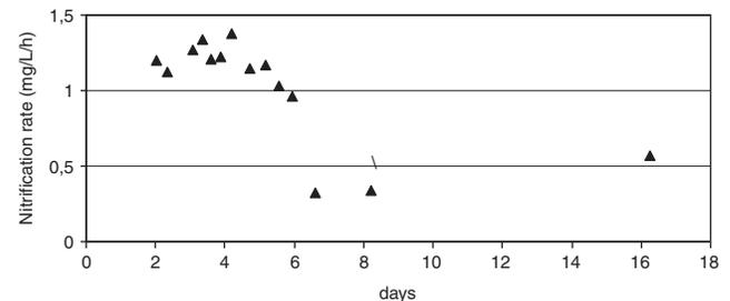
Fig. 5. Pilot scale batch growth of nitrifiers on a substrate of ammonia chloride.
