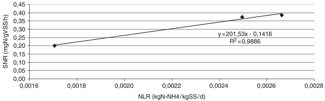
Fig. 2. Linear increase of SNR with NLRs in the conventional continuously-fed MBR.
