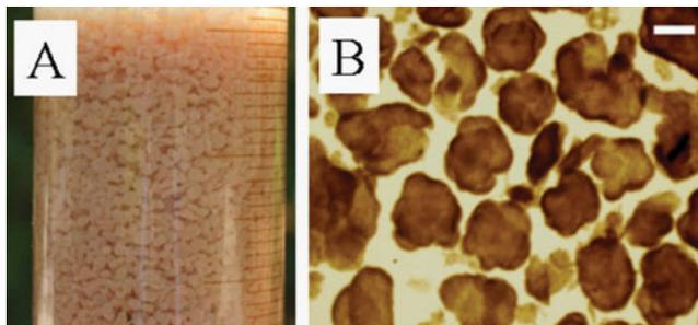
Fig. 1. Morphology of the aerobic microbial granules cultivated in a 3 l sequencing batch reactor. A) Cultivated microbial granules transferred to a measuring cylinder B) stereozoom micrograph. Scale bar in B, 1 mm.
