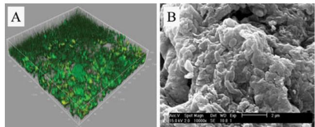
Fig. 2. Microstructure of aerobic microbial granule as shown by confocal microscopy (A) and scanning electron microscopy (B) Confocal image consisted of 28 xy-slices obtained at z-interval of 2  $\mu$ m.
