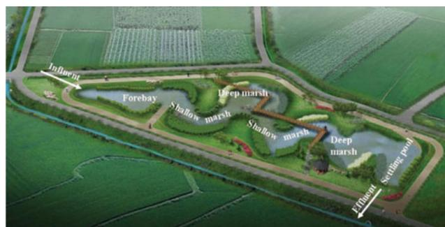
Fig. 2. Schematic diagram of the stormwater wetland in this study.
