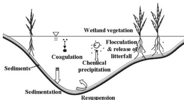
Fig. 1. Schematic diagram of the behavior of particles in a wetland.
