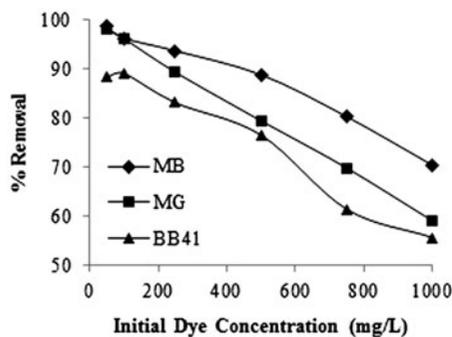
Fig. 5. Effect of initial dye concentration on removal of MB, MG, and BB41.
