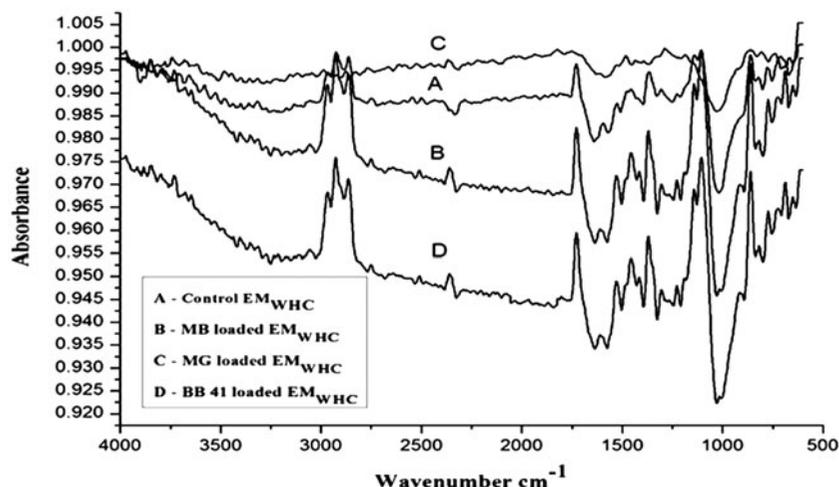
Fig. 1. FTIR spectrum for  $EM_{WHC}$  Control and MB, MG, and BB 41-loaded  $EM_{WHC}$ .
