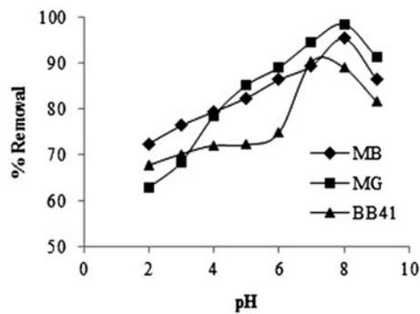
Fig. 3. Effect of pH on removal of MB, MG, and BB41.
