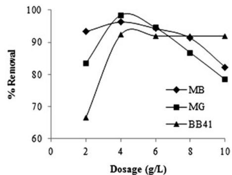
Fig. 4. Effect of adsorbent dosage on removal of MB, MG, and BB41.
