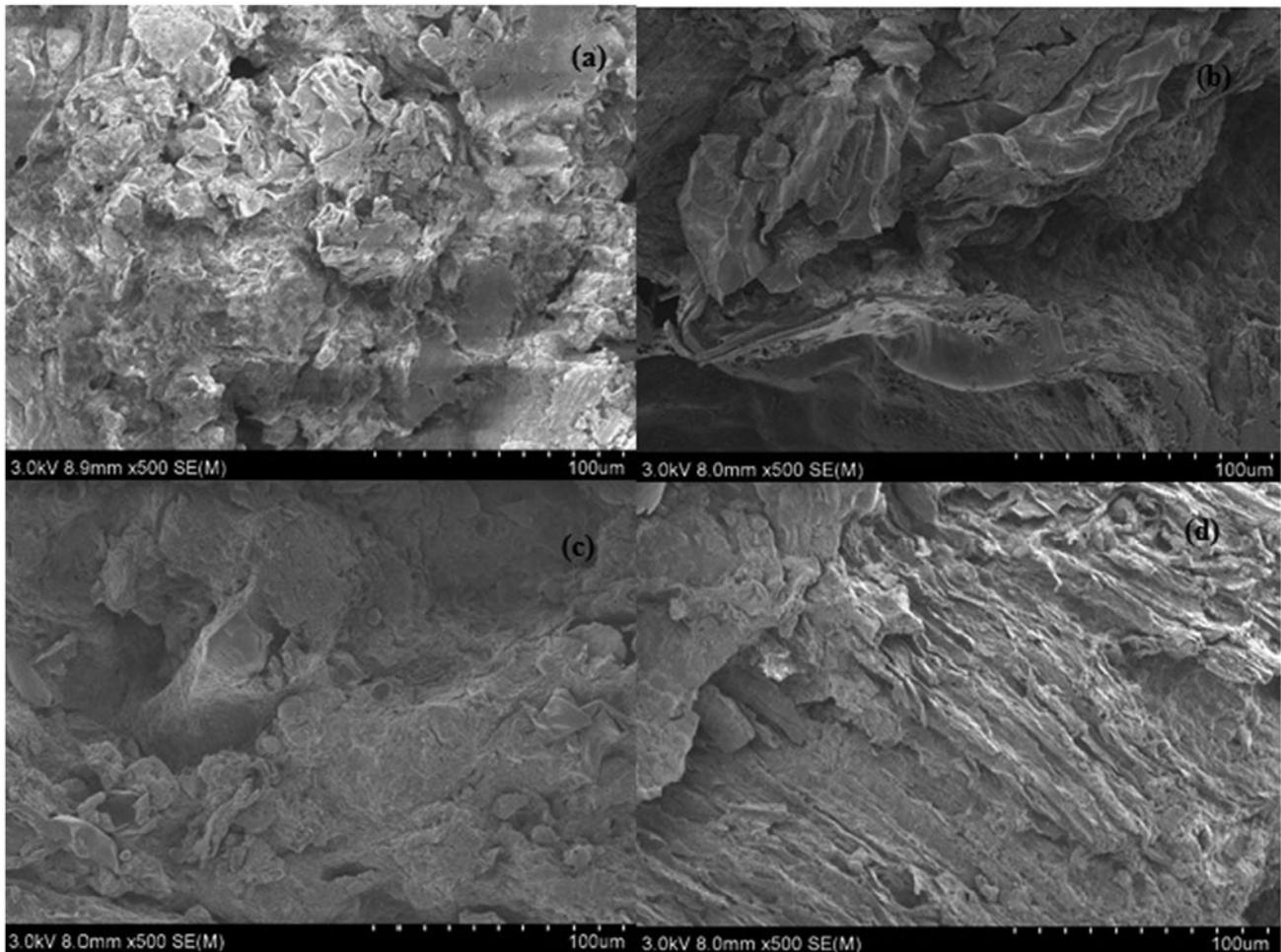
Fig. 2. SEM images of (a) EM<sub>WHC</sub> Control and loaded with (b) MG, (c) MB, and (d) BB41.
