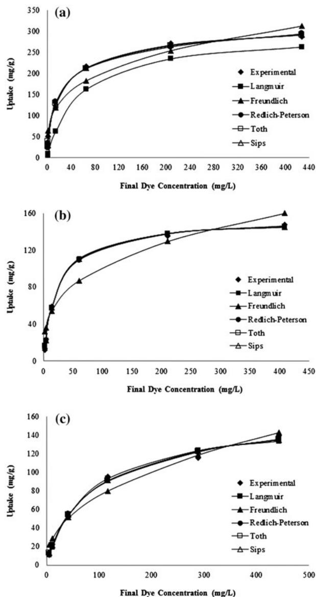
Fig. 7. Biosorption Isotherms for (a) MB, (b) MG, and (c) BB41 onto EM<sub>WHC</sub>.
