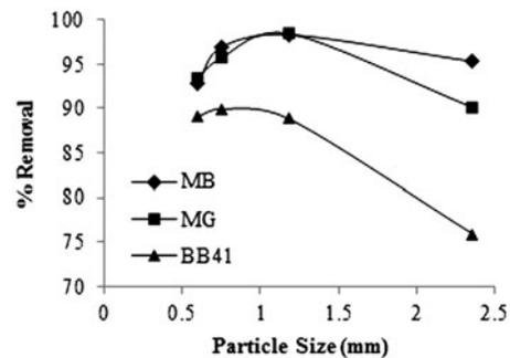
Fig. 6. Effect of adsorbent particle size on removal of MB, MG, and BB41.
