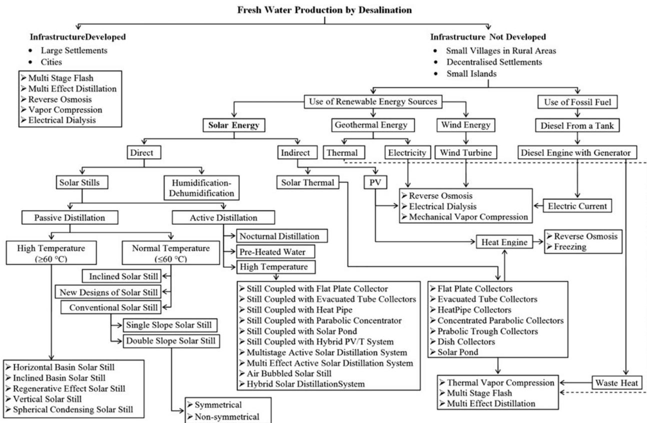
Fig. 1. Desalination techniques used for fresh water production [3,6,7].
