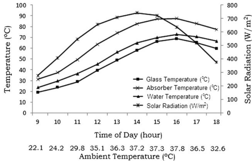
Fig. 3. Hourly variations of temperatures and solar radiation for solar collector-assisted solar still.
