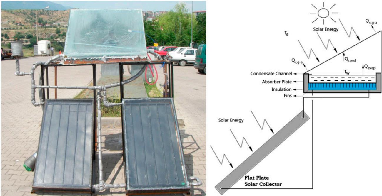
Fig. 2. Basin still coupled with a FPC in the natural circulation and closed cycle mode with its schematic diagram.
