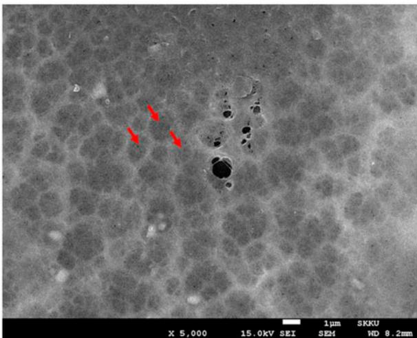
Fig. 9. SEM image of the support layer surface under HA 100 ppm condition.
