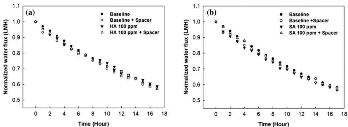
Fig. 2. The water flux decline curve for organic matter. Average values were taken to represent support layer fouling: (a) HA and (b) SA.
