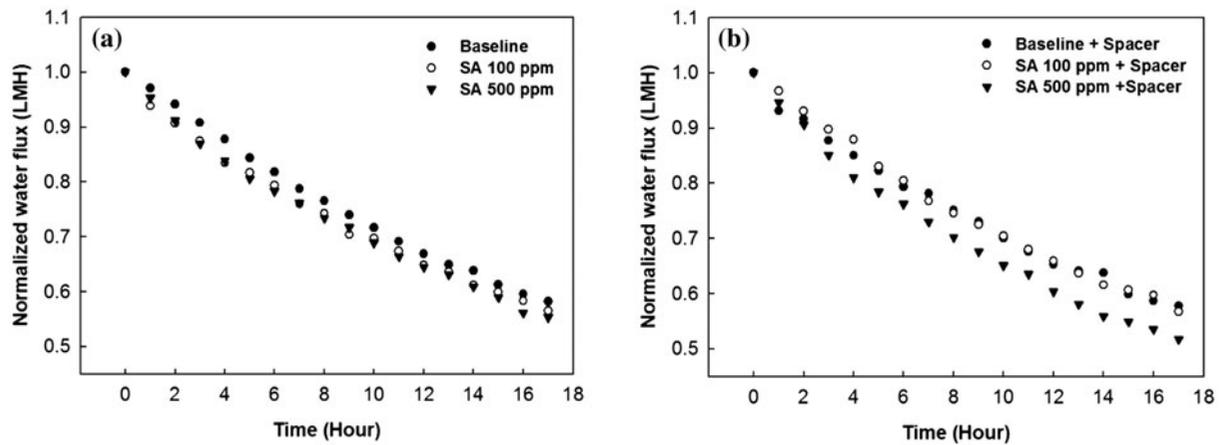
Fig. 4. Water flux decline curve for SA. Values were averaged to represent support layer fouling: (a) Without spacer and (b) With spacer.
