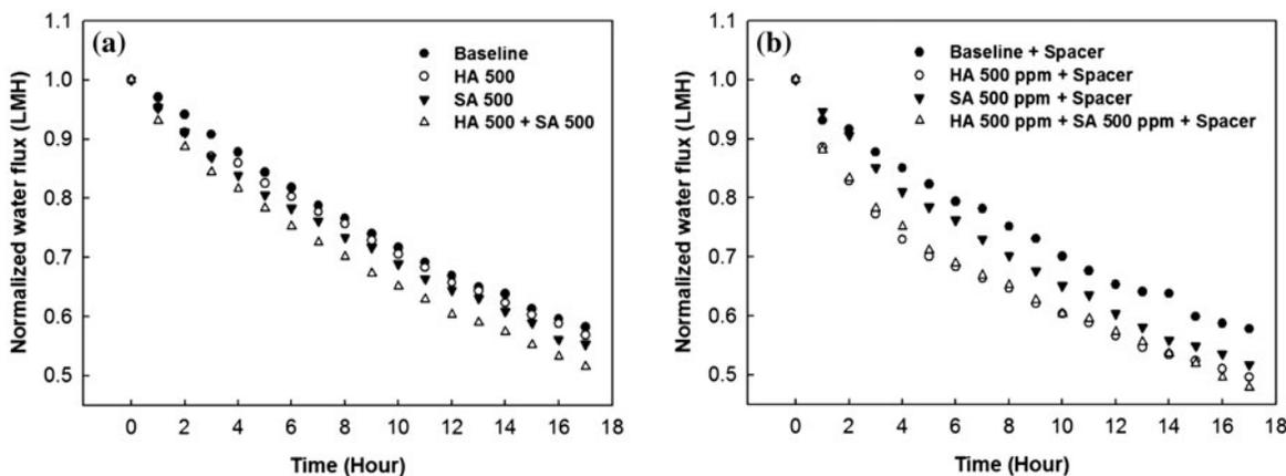
Fig. 5. The water flux decline curve for mixed solution. Values were averaged to represent support layer fouling. (a) Without spacer and (b) With spacer.
