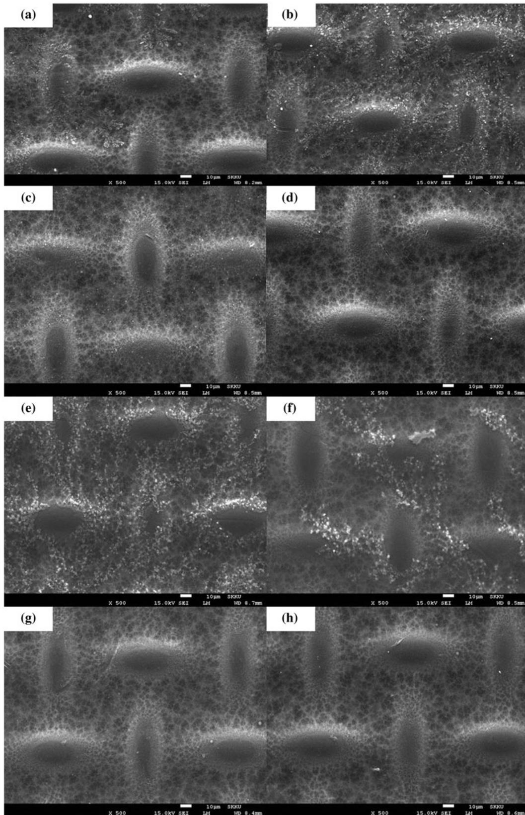
Fig. 7. SEM images on the fouled membrane by organic matter: (a) Baseline, (b) Baseline + spacer, (c) HA 500 ppm, (d) HA 500 ppm + spacer, (e) SA 500 ppm, (f) SA 500 ppm + spacer, (g) Mixing, and (h) Mixing + spacer.
