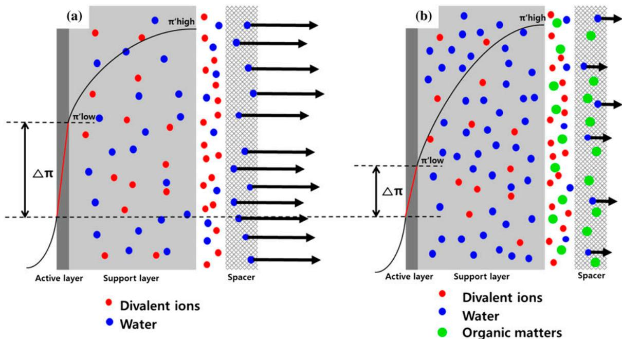
Fig. 10. A conceptual illustration of the permeate water flux on the draw solution side: (a) with spacer and (b) with spacer and organic matter.
