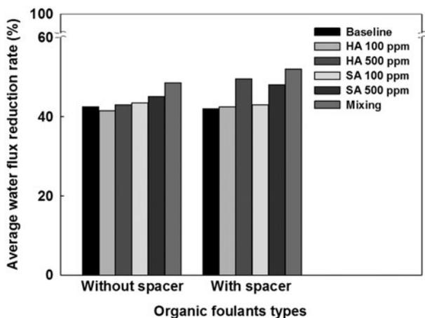
Fig. 6. Average water flux reduction rate comparison (%) without or with spacer.
