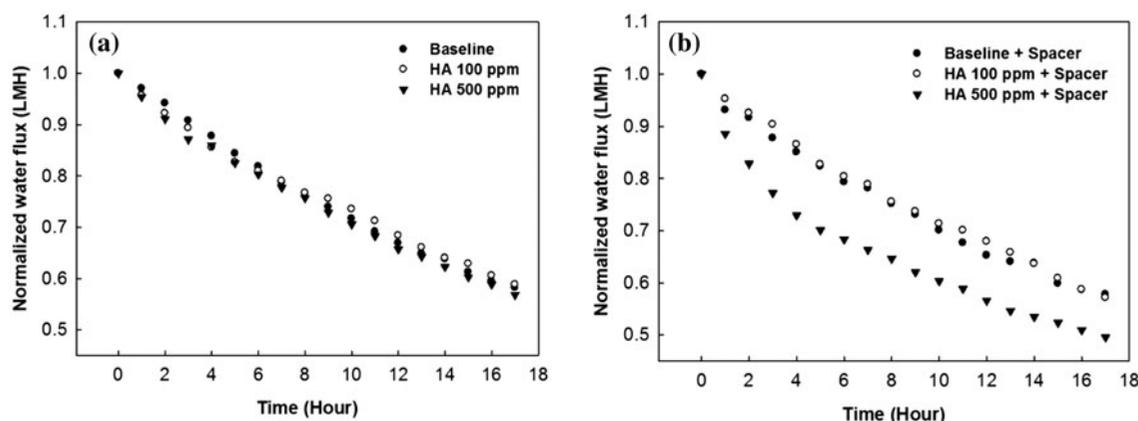
Fig. 3. Water flux decline curve for HA. Values were averaged to represent support layer fouling: (a) Without spacer and (b) With spacer.
