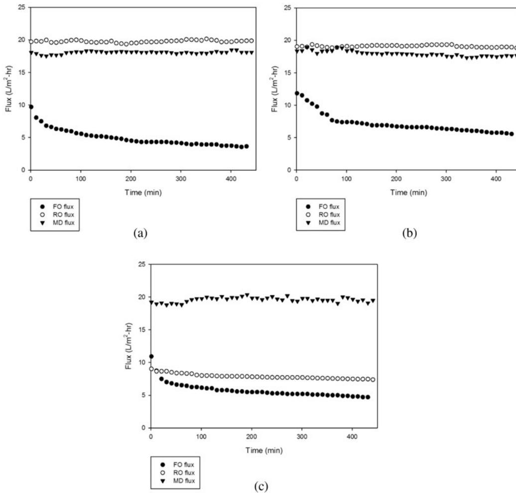
Fig. 6 Comparison of flux behaviors in FO, RO, and MD systems: (a) Feed water containing alginate of 500 mg/L, (b) Feed water containing alginate of 500 mg/L and NaCl of 1,000 mg/L, (c) Feed water containing alginate of 500 mg/L and NaCl of 35,000 mg/L, and (d) Normalized flux after the experiment.
