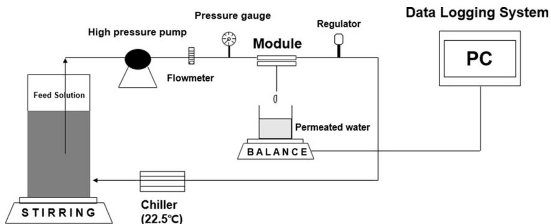
Fig. 2. Schematic diagram of laboratory-scale RO system.
