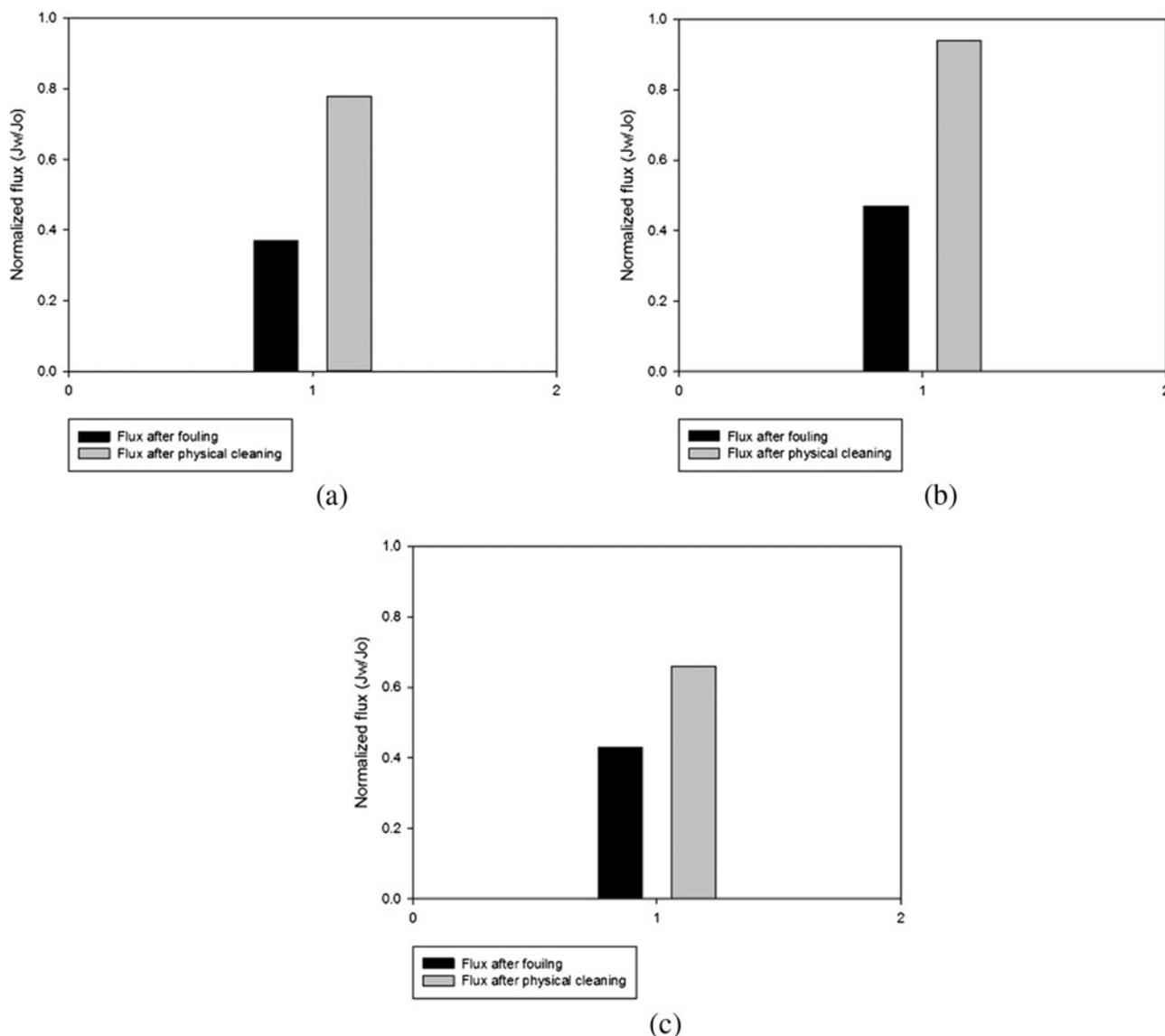
Fig. 9. Comparison of flux recovery for FO membranes fouled by alginate: (a) Feed water containing alginate of 500 mg/L, (b) Feed water containing alginate of 500 mg/L and NaCl of 1,000 mg/L and (c) Feed water containing alginate of 500 mg/L, and NaCl of 35,000 mg/L.
