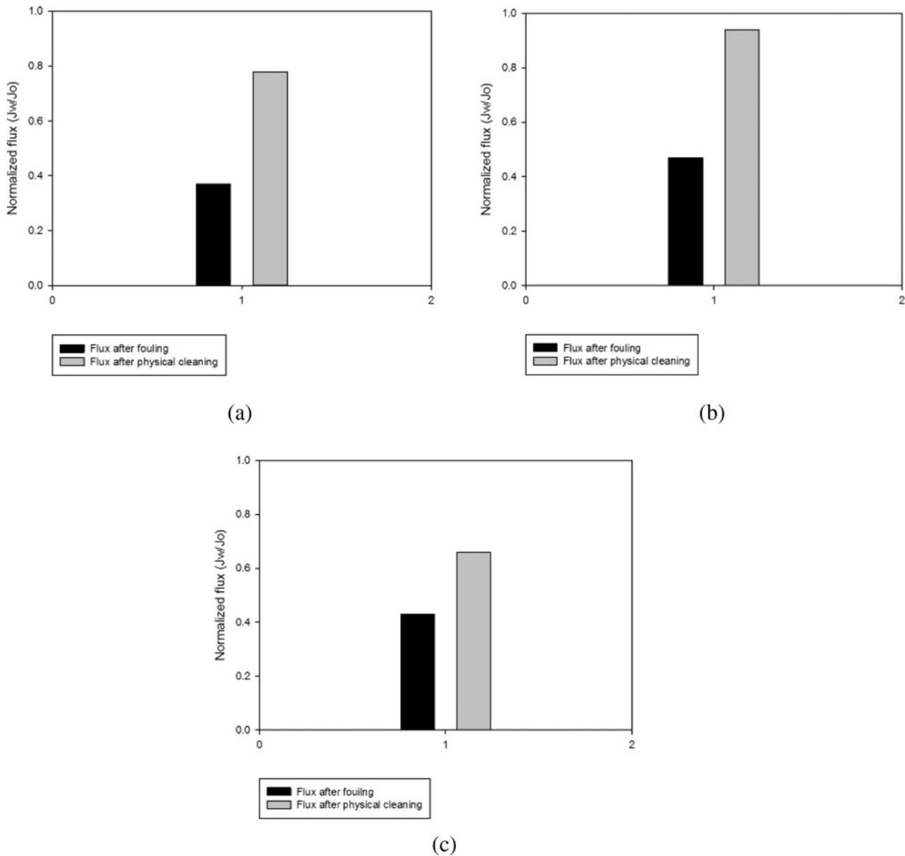
Fig. 8. Comparison of flux recovery for FO membranes fouled by colloidal silica: (a) Feed water containing colloidal silica of 5,000 mg/L, (b) Feed water containing colloidal silica of 5,000 mg/L and NaCl of 1,000 mg/L, and (c) Feed water containing colloidal silica of 5,000 mg/L and NaCl of 35,000 mg/L.
