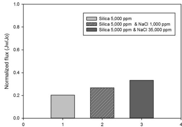
Fig. 5. Effect of NaCl concentration on flux decline by colloidal silica in FO system.
