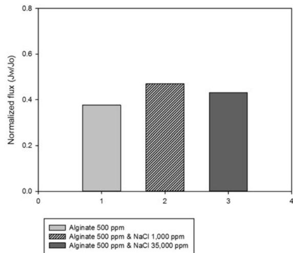
Fig. 7. Effect of NaCl concentration on flux decline by alginate in FO system.
