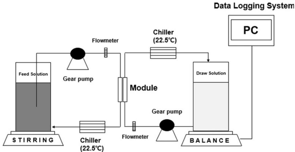
Fig. 1. Schematic diagram of laboratory-scale FO system.
