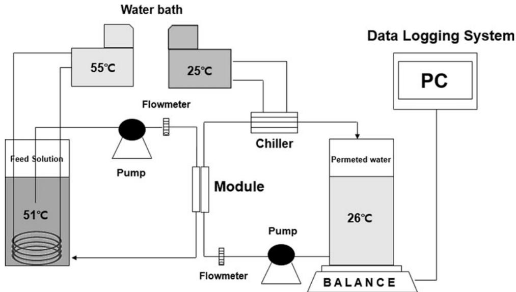
Fig. 3. Schematic diagram of laboratory-scale DCMD system.
