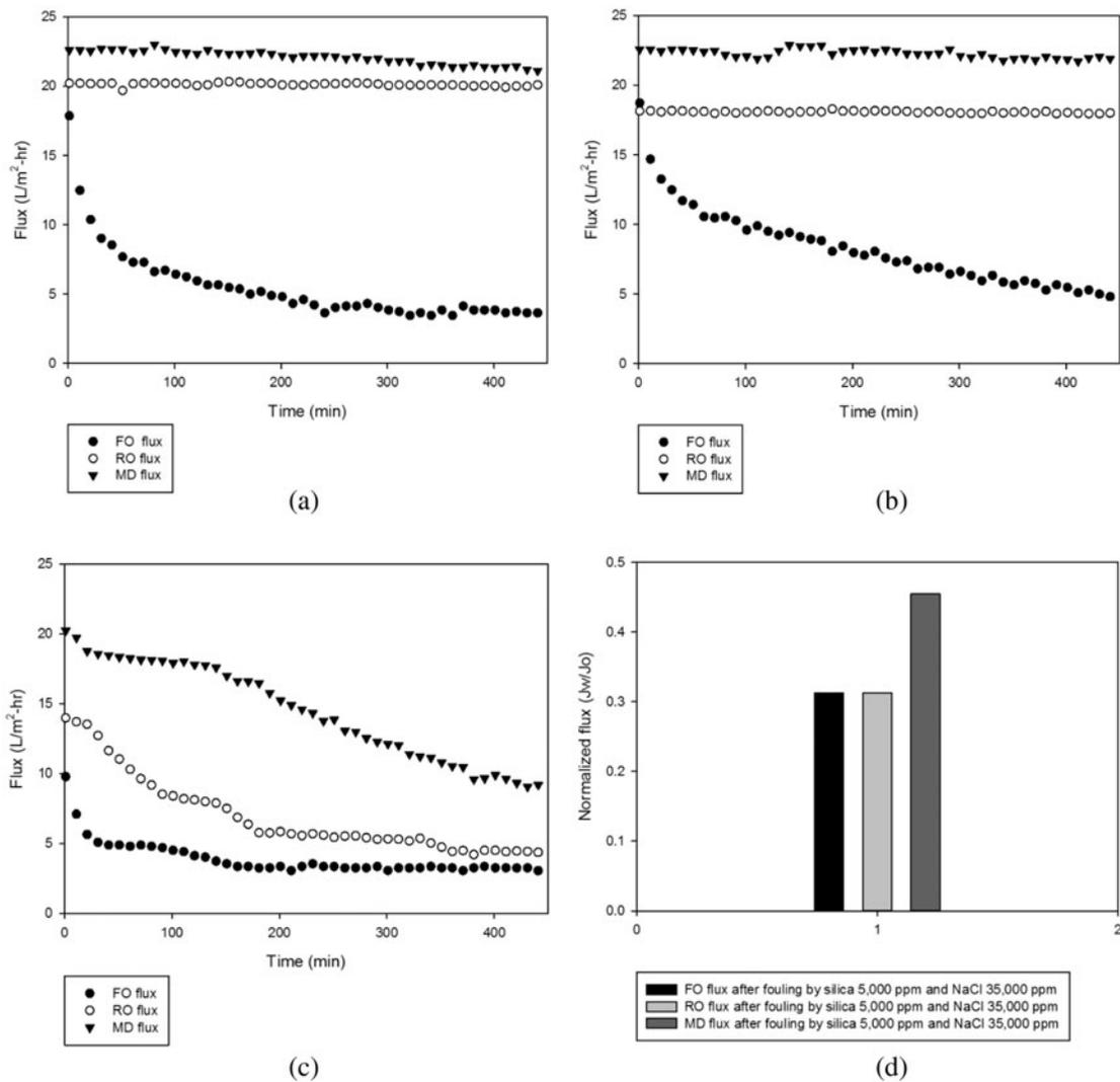
Fig. 4. Comparison of flux behaviors in FO, RO, and MD systems: (a) Feed water containing colloidal silica of 5,000 mg/L, (b) Feed water containing colloidal silica of 5,000 mg/L and NaCl of 1,000 mg/L, (c) Feed water containing colloidal silica of 5,000 mg/L and NaCl of 35,000 mg/L, and (d) Normalized flux after the experiment.
