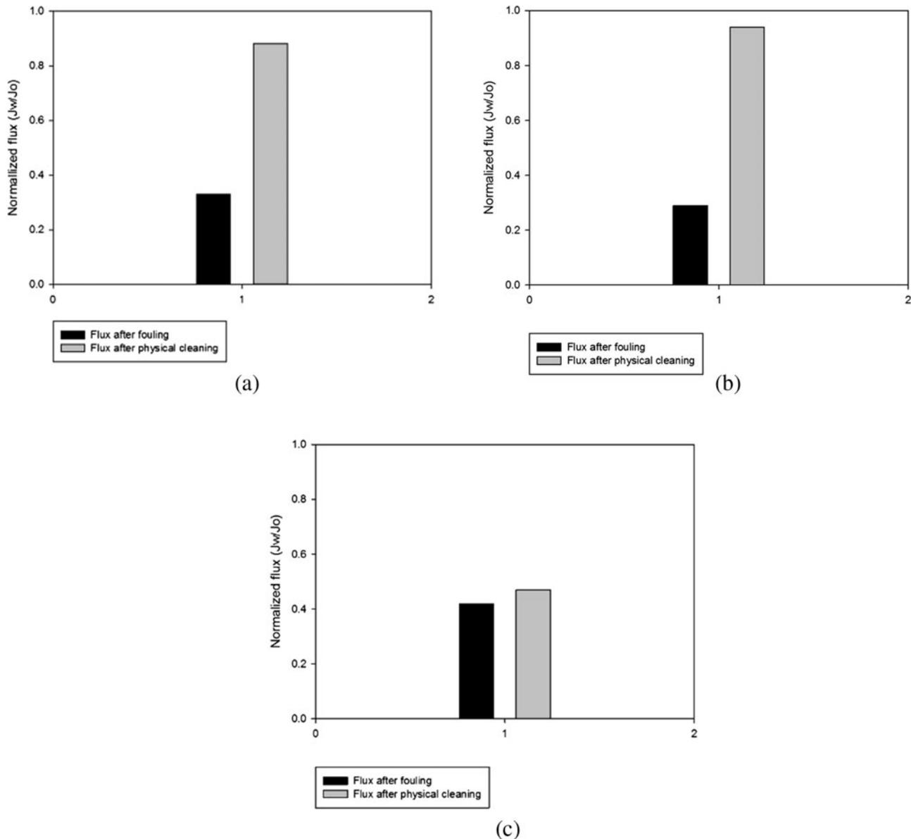
Fig. 10. Comparison of flux recovery for FO, RO, and MD membranes fouled by colloidal silica in NaCl solution of 35,000 mg/L: (a) FO membrane, (b) RO membrane, and (c) MD membrane.
