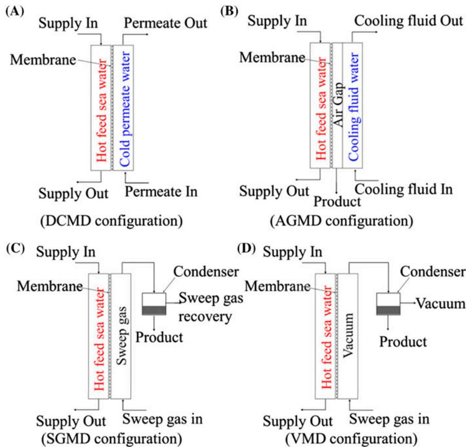
Fig. 1. Different types of membrane distillation: (A) DCMD, (B) AGMD, (C) SGMD, and (D) VMD.
