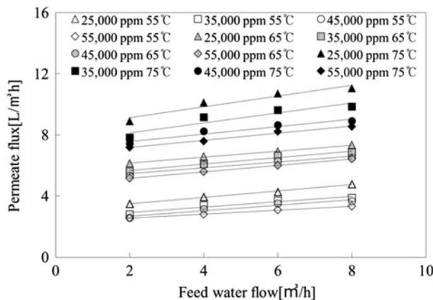
Fig. 6. LMH per feedwater flow rate conditions.
