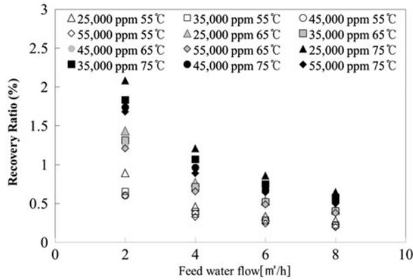
Fig. 8. RR of VMD module per feedwater conditions.
