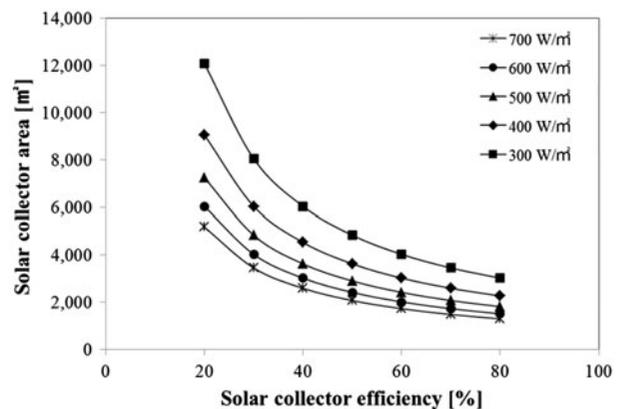
Fig. 10. Solar collector areas required for 10 m<sup>3</sup>/d solar thermal VMD seawater desalination plant with respect to solar thermal collector efficiency and insolation.
