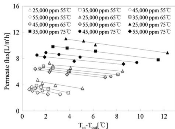
Fig. 7. Temperature difference between VMD module inlet and outlet with respect to feedwater salinity and temperature conditions.
