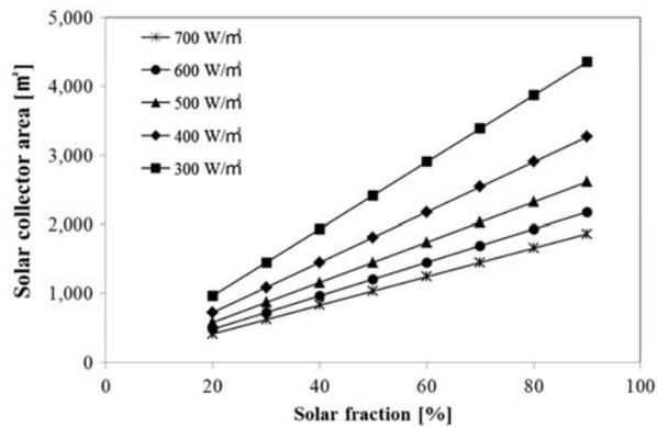
Fig. 11. Solar collector areas required for 10 m<sup>3</sup>/d solar thermal VMD seawater.
