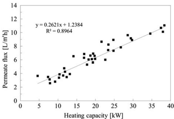
Fig. 9. LMH values of VMD module with respect to feed heat capacity.
