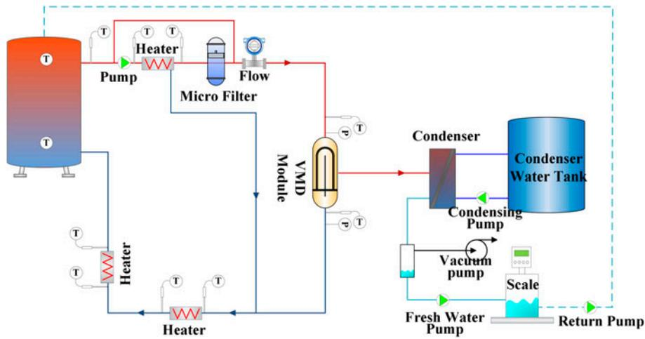
Fig. 4. Experimental equipment to test VMD performance.
