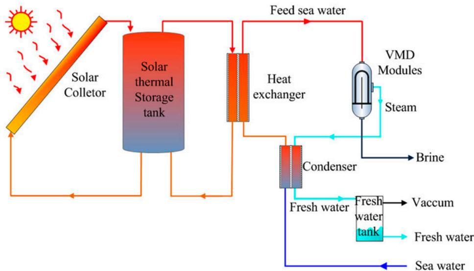
Fig. 2. Diagram for solar thermal system used VMD system.
