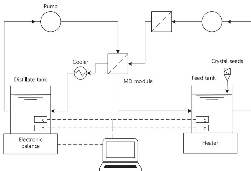
Fig. 1. Schematic diagram of experimental setup for MD.
