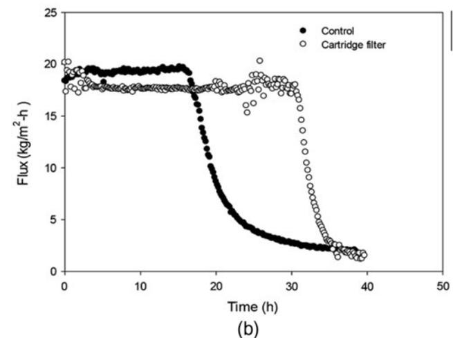
Fig. 4. Effect of in-line filtration on MD flux decline due to scale formation: (a) flux vs. VCF and (b) flux vs. time.
