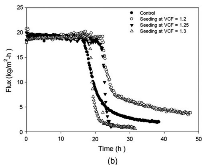
Fig. 3. Effect of crystal seeding on MD flux declines due to scale formation: (a) flux vs. VCF and (b) flux vs. time.
