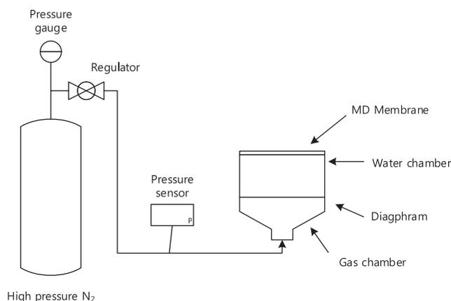
Fig. 2. Schematic diagram of experimental setup for liquid entry pressure measurement (LEP).
