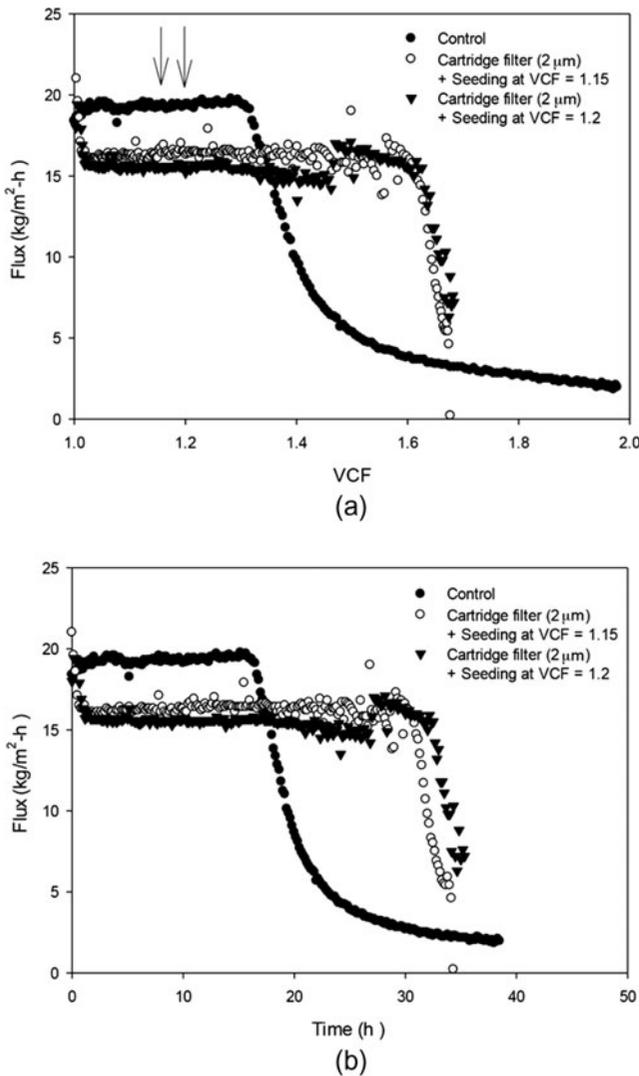
Fig. 5. Effect of crystal seeding followed by in-line filtration on MD flux decline due to scale formation: (a) flux vs. VCF and (b) flux vs. time.
