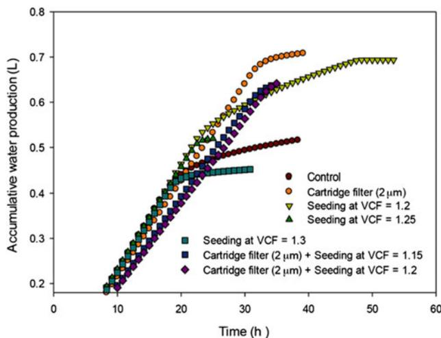
Fig. 6. Comparison of accumulative water production in MD operation for different antiscaling methods.
