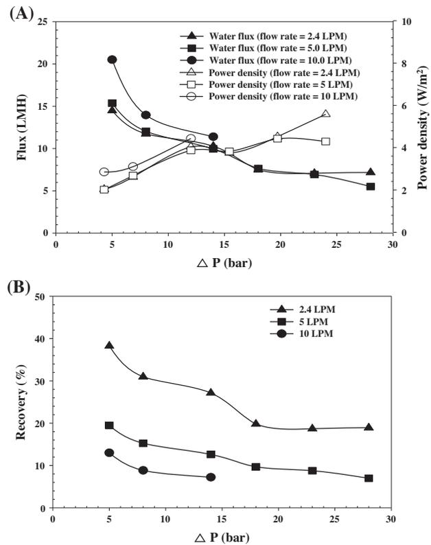
Fig. 3. Effect of draw and feed solutions flow rate on the PRO performance. Water flux and PD (A) and recovery of feed solution (B).
