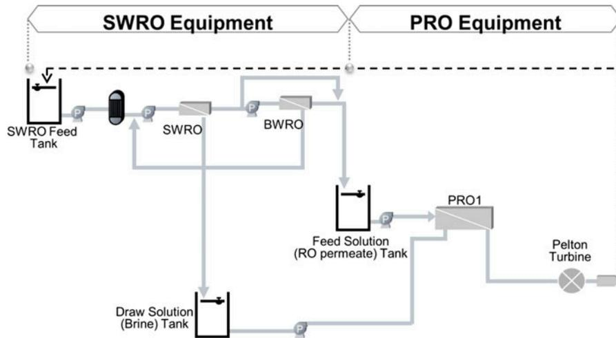
Fig. 1. Schematic diagram of the SWRO-PRO semi-pilot (capacity, 20 m<sup>3</sup>/d).
