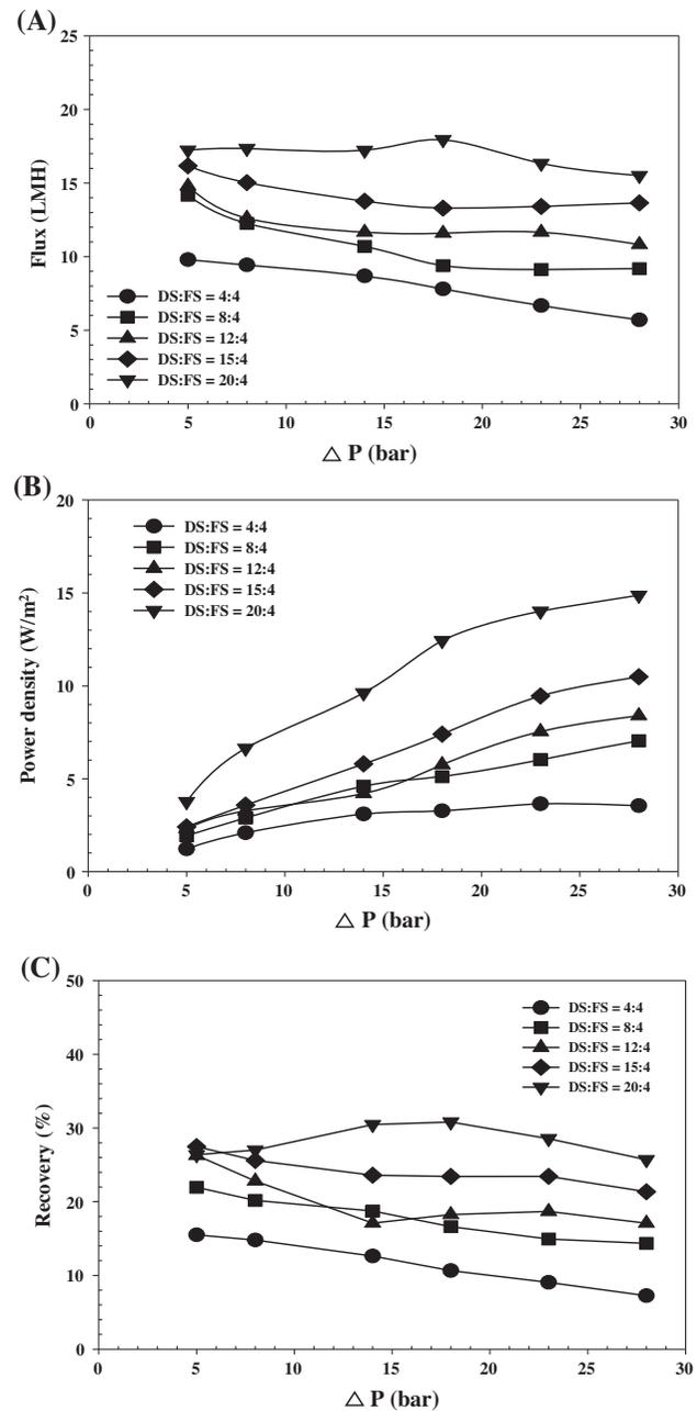
Fig. 5. Impact of various draw solution ratios on PRO performance. Feed solution was fixed as 4 L/min and draw solution was changed from 4 to 20 L/min. Ratio is 1:1, 2:1, 3:1, 3.75:1, 5:1, respectively. Water flux (A), PD (B), and recovery (C).
