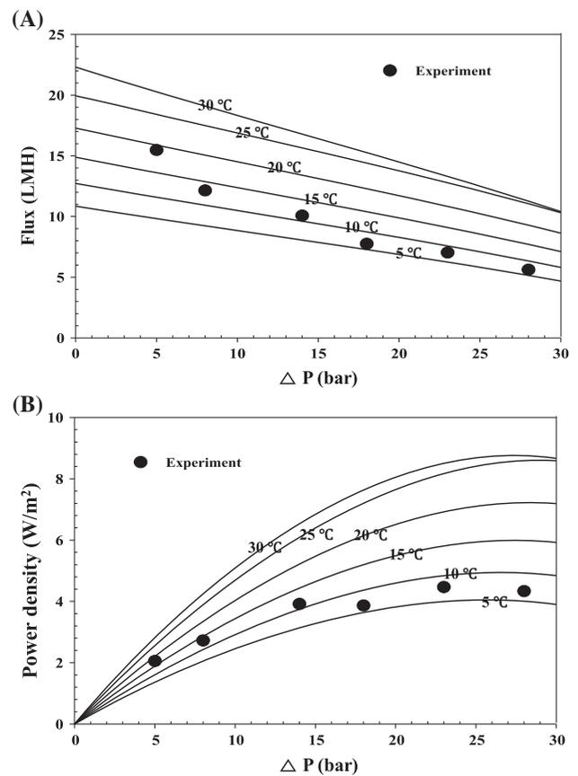
Fig. 6. Experimental and simulated water flux (A) and PD (B) for the PRO module. Simulation results were obtained from Eq. (5). Experimental conditions: The draw and feed solutions were 70,000 mg/L NaCl and 400 mg/L RO permeate, respectively. The inlet flow rates of draw and feed solutions were maintained 5 LPM at 25°C.
