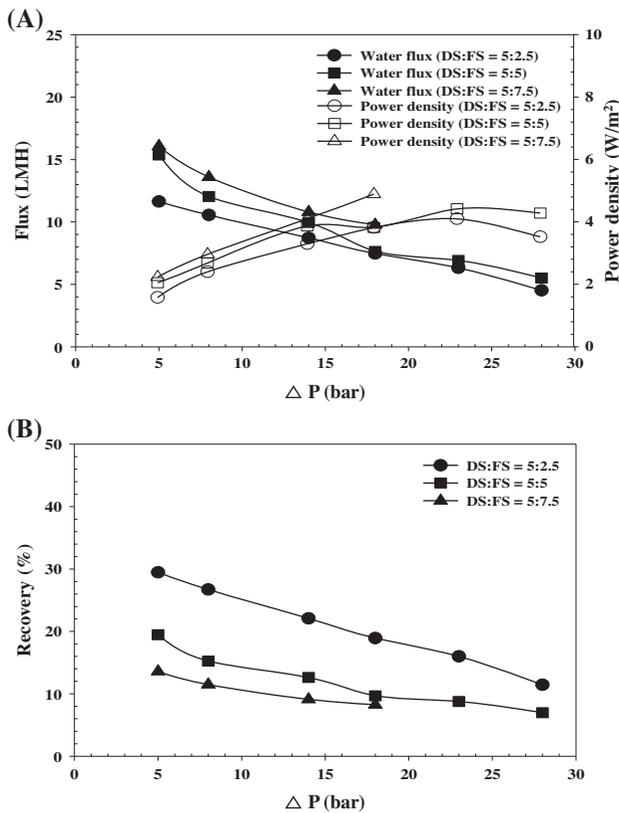
Fig. 4. Impact of various feed solution ratios on PRO performance. Draw solution was fixed as 5 L/min and feed solution was changed from 2.5 to 7.5 L/min. Ratio is 1:0.5, 1:1, 1:1.5, respectively. Water flux and PD (A) and recovery (B).
