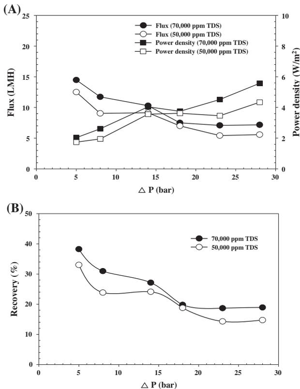
Fig. 2. Effect of applied pressure on water flux and PD (A) and recovery (B) in the PRO system at different draw solution concentrations.
