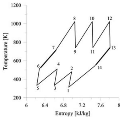
Fig. 5. T-s diagram of reference cycle for the conversion section.
