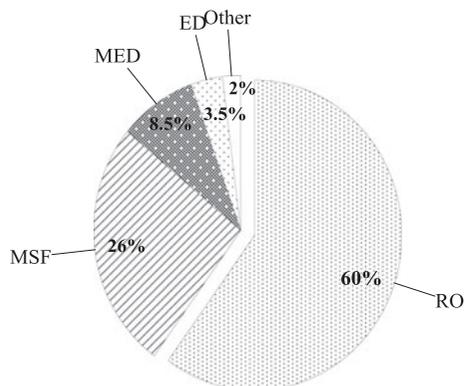
Fig. 2. Worldwide installed desalination capacities by technology for a total of 66.5 million m<sup>3</sup>/d, 2011 [27].
