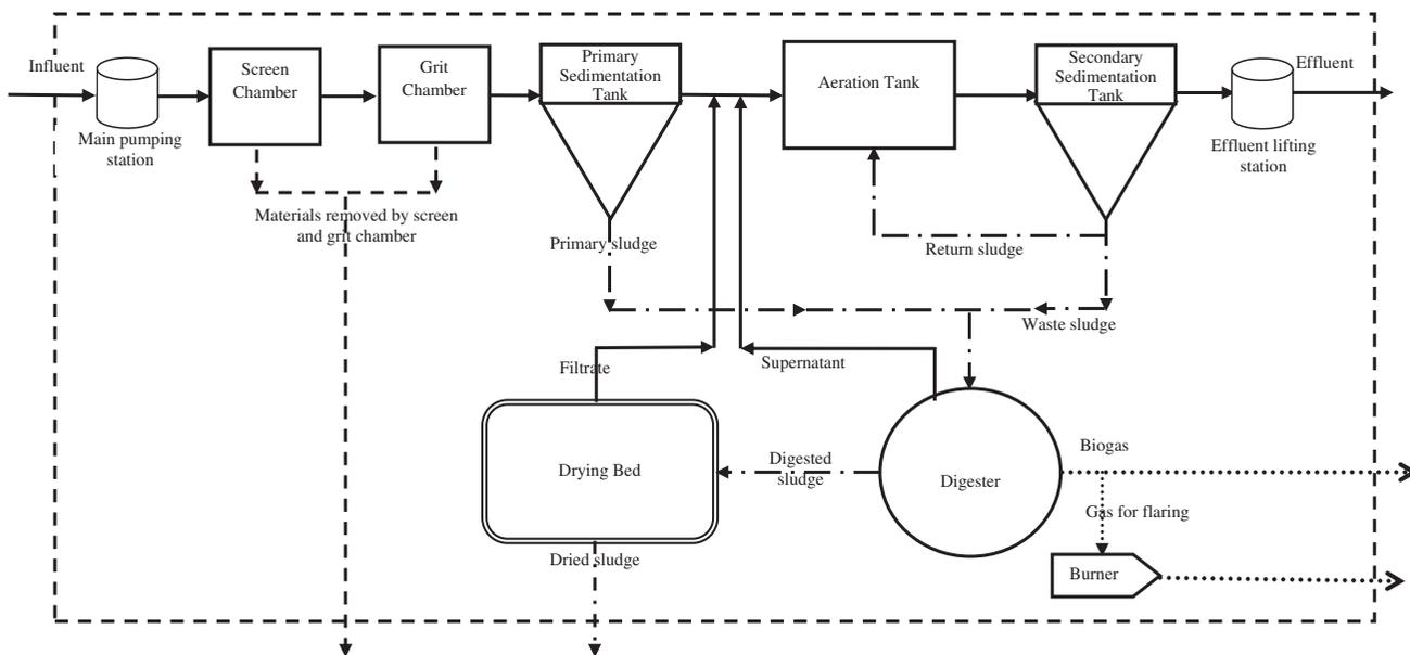
Fig. 1. Flow diagram of Beur Municipal Wastewater Treatment Plant Unit-I (BMWTP-I).
