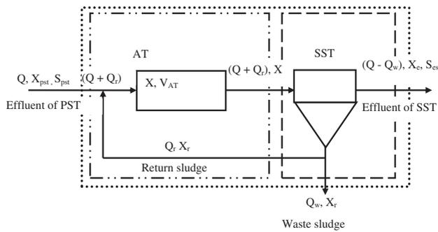
Fig. 2. Mass balance around AT and SST.
