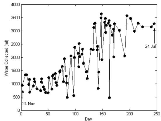
Fig. 4. The amount of distilled water produced by the still over the entire experiment.
