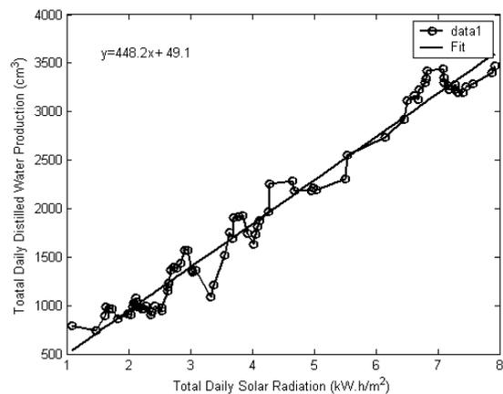
Fig. 7. The amount of water collected plotted vs. total solar radiation for daylight time.
