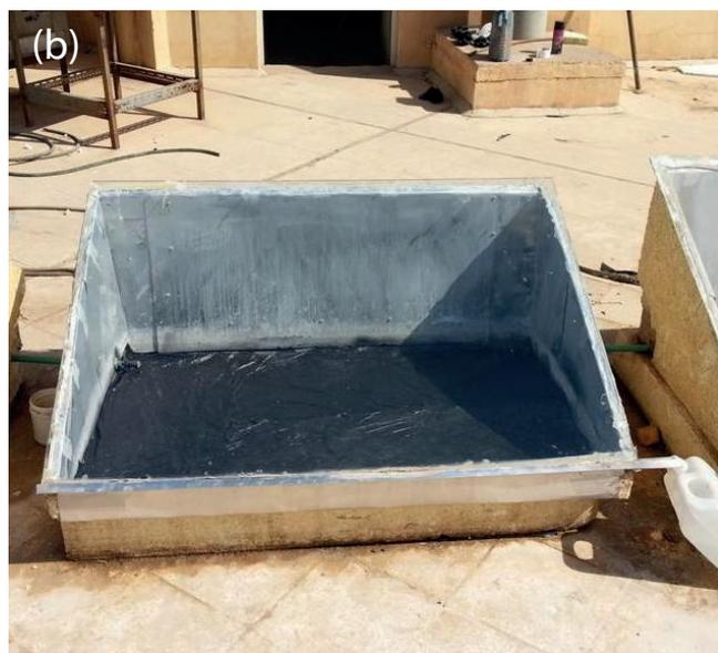
Fig. 1. Experimental solar still: (a) sketch diagram (lateral view) and (b) actual basin.
