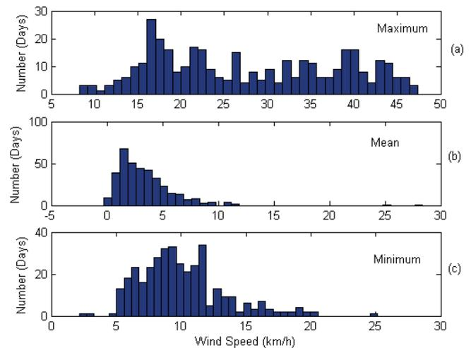
Fig. 3. (a) Maximum, (b) mean, and (c) minimum daily wind speed distribution in Mosul for between first of November 2014 and end of September 2015.
