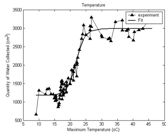
Fig. 8. The amount of collected water plotted against maximum daylight temperature.
