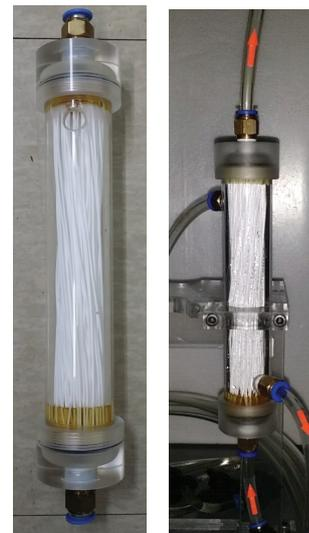
Fig. 1. Photo images of (a) a detached module of 180 PVDF hollow fibers and (b) the same module connected to a feed tank and a vacuum pump in the VMD system.
