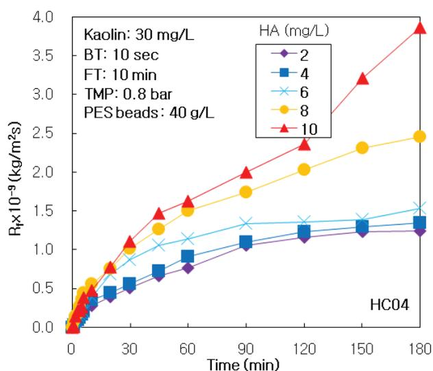
Fig. 2. Effect of HA on resistance of membrane fouling in hybrid water treatment process of multi-channel ceramic MF and photocatalyst-loaded PES beads.
