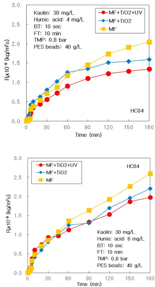
Fig. 4. Role of membrane filtration, adsorption and photo-oxidation on resistance of membrane fouling in hybrid process of multi-channel ceramic MF and photocatalyst-loaded PES beads; (a) HA 4 mg/L, (b) HA 6 mg/L.
