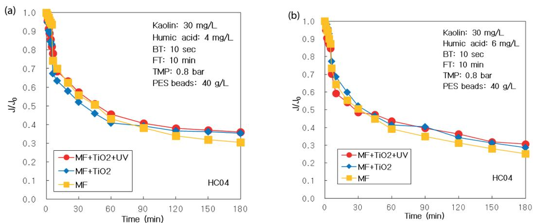
Fig. 5. Role of membrane filtration, adsorption and photo-oxidation on dimensionless permeate flux in hybrid process of multi-channel ceramic MF and photocatalyst-loaded PES beads; (a) HA 4 mg/L, (b) HA 6 mg/L.
