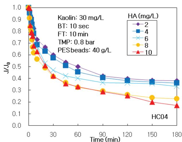
Fig. 3. Effect of HA on dimensionless permeate flux in hybrid water treatment process of multi-channel ceramic MF and photocatalyst-loaded PES beads.
