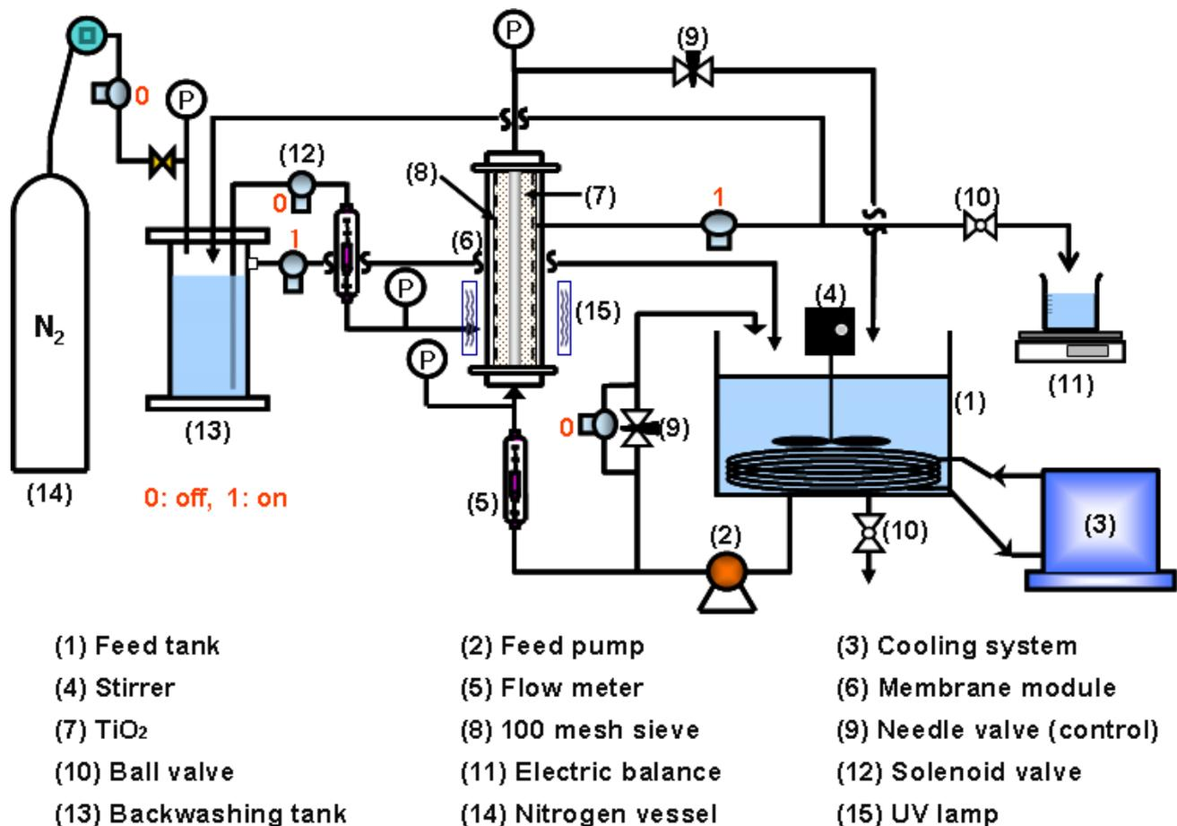
Fig. 1. Apparatus of hybrid water treatment process of multi-channel ceramic microfiltration and the photocatalyst-loaded PES beads with periodic water back-flushing [23].
