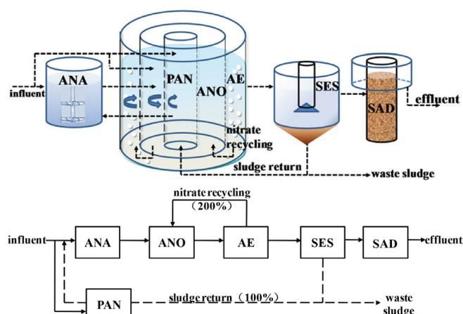
Fig. 1. Layout (a) and schematic diagram (b) of the JHB-SAD system. PAN: pre-anoxic zone; ANA: anaerobic zone; ANO: anoxic zone; AE: aerobic zone; SES: secondary settler; SAD: sulfur autotrophic denitrification reactor.
