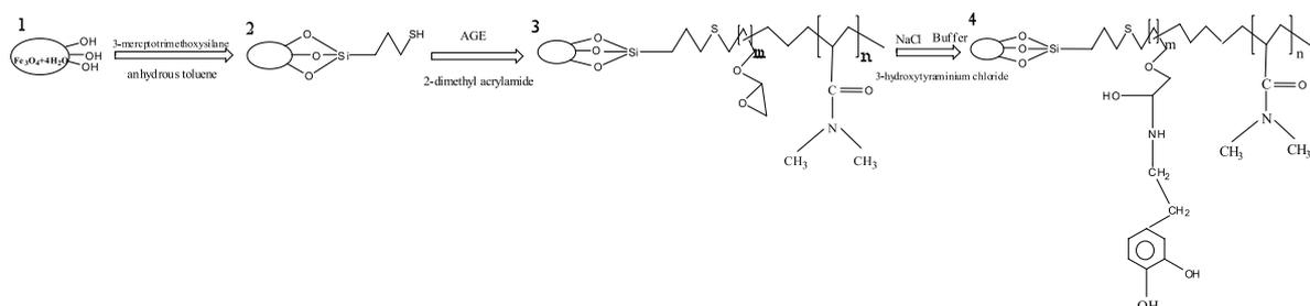
Fig. 1. Schematic presentation of four stages of iron magnetic nanoparticles synthesis.
