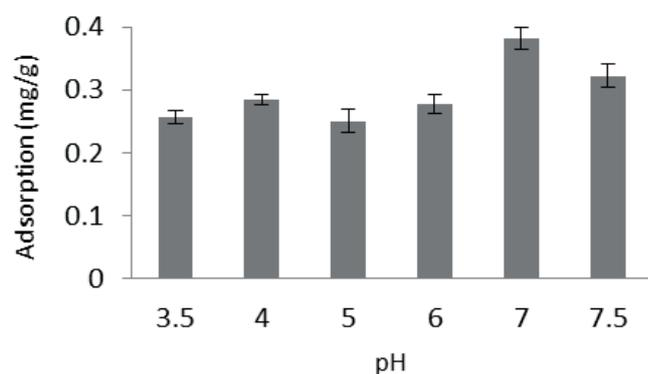
Fig. 3. Effect of pH on uptake of deltamethrin (20 mg/L) by PCH-MNP (0.05 g) at 20°C (results are represented as mean  $\pm$  SD;  $n = 4$ ).
