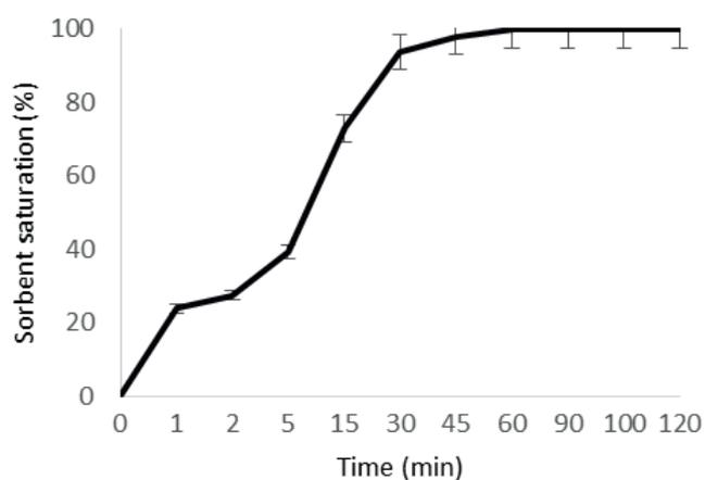
Fig. 4. Effect of contact time on the uptake of deltamethrin (20 mg/L) by PCH-MNP (0.05 g) at pH 7 and 20°C (results are represented as mean  $\pm$  SD;  $n = 4$ ).
