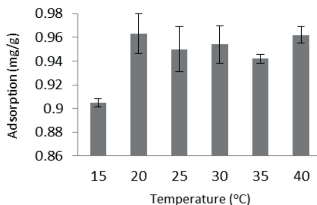
Fig. 5. Effect of temperature on the uptake of deltamethrin (20 mg/L) by PCH-MNP (0.05 g) at pH 7 (results are represented as mean  $\pm$  SD;  $n = 4$ ).
