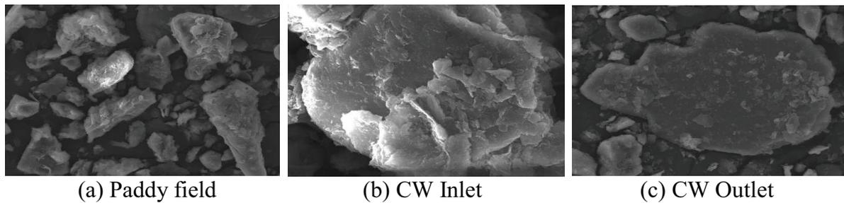
Fig. 7. SEM photographs of the sediment collected at respective sampling locations; (a) Paddy field, (b) CW Inlet, (c) CW Outlet.
