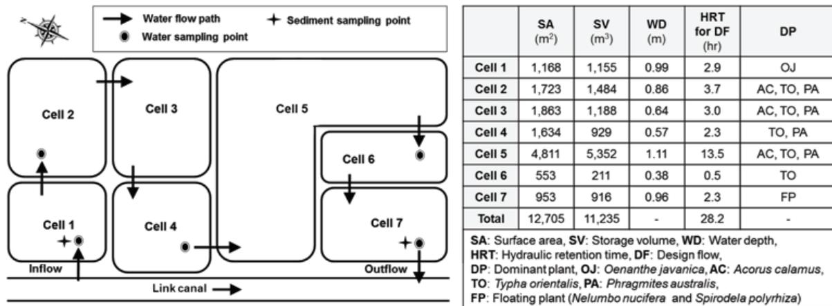
Fig. 1. Schematic diagram and design information of the CW (Cell 1 and 7: sedimentation zone, Cell 2 and 5: deep marsh, Cell 3 and 4: shallow and deep marsh, Cell 6: shallow marsh).
