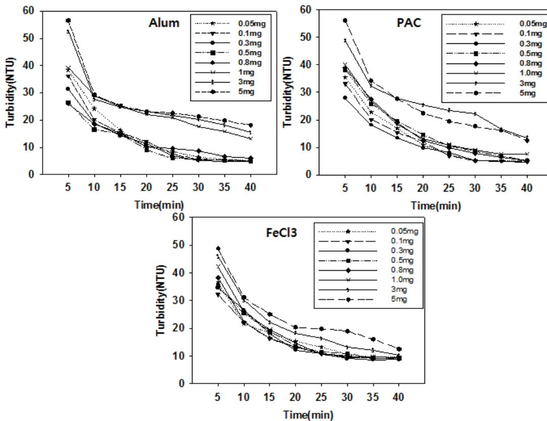
Fig. 6. Sedimentation rate of flocs by weighted coagulant dose.
