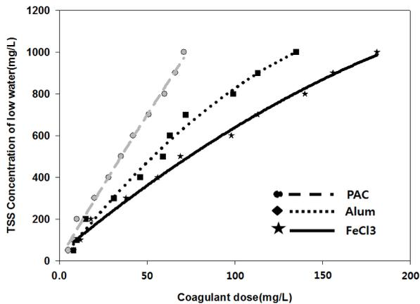
Fig. 8. Coagulant dose curve obtained by TSS concentration in raw water.
