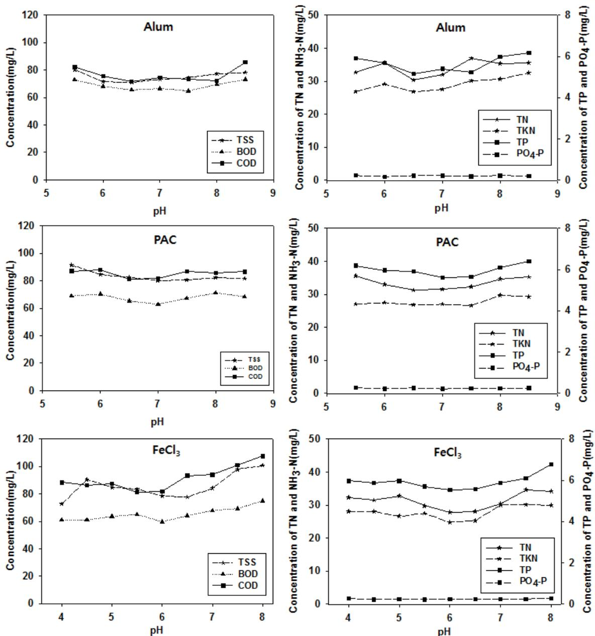
Fig. 3. Experiment result to determine optimum pH.
