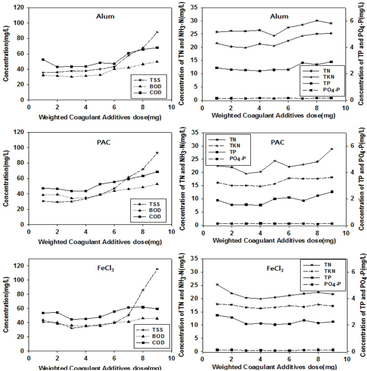
Fig. 5. Experiment result to determine optimum WCA dose.
