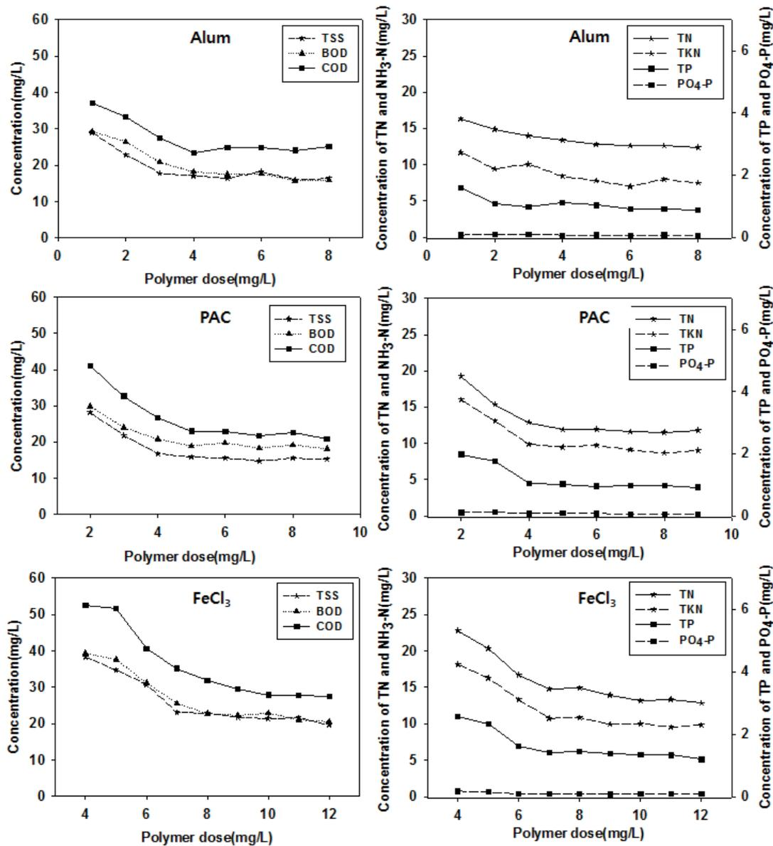
Fig. 7. Experiment result to determine optimum polymer dose.
