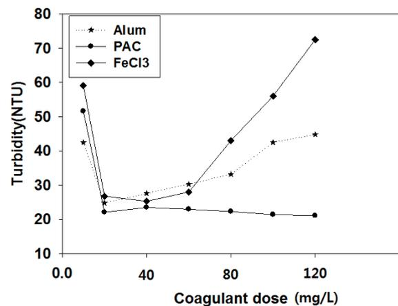
Fig. 2. Result of the preceding research to determine the optimum coagulant dose.
