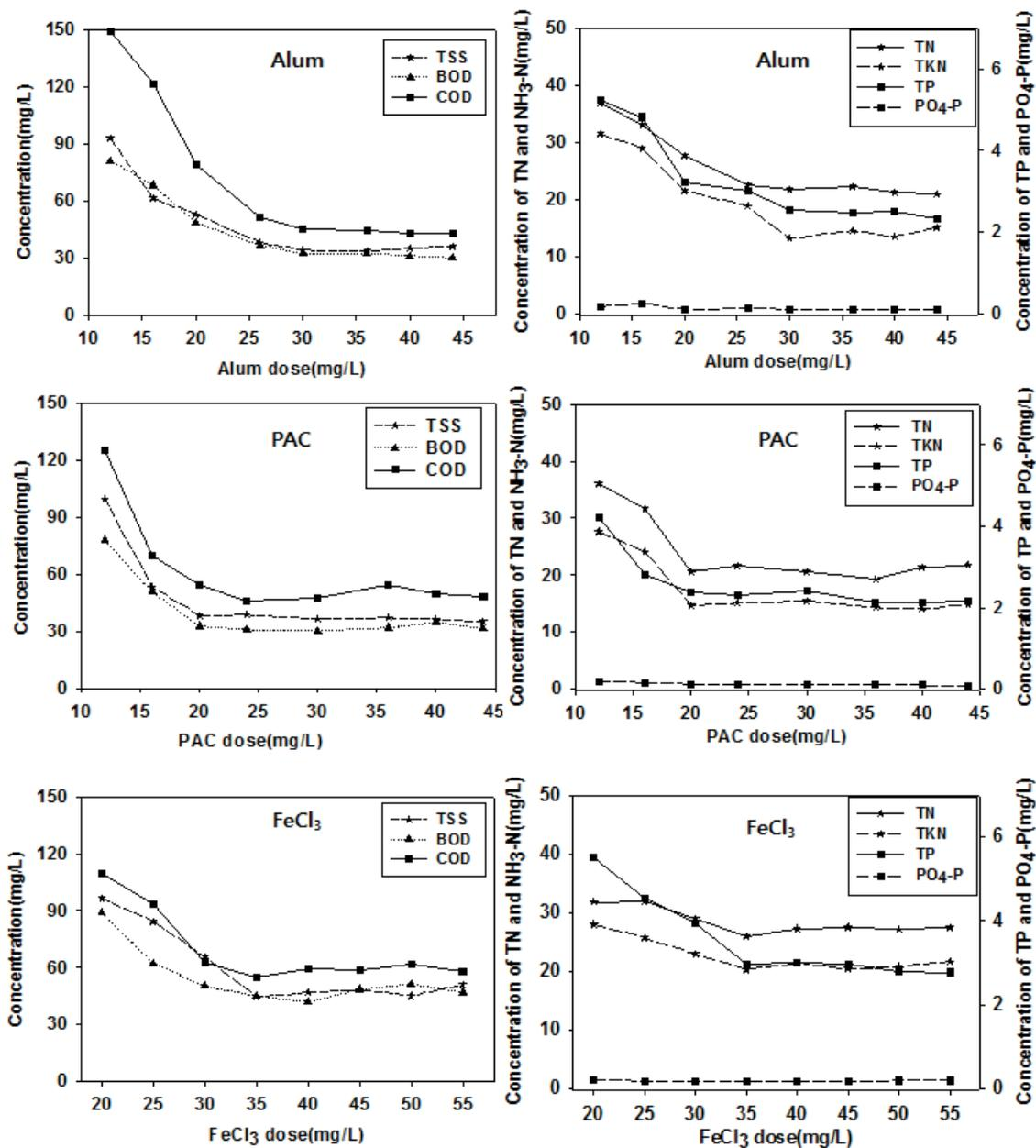
Fig. 4. Experiment result to determine optimum coagulants dose.
