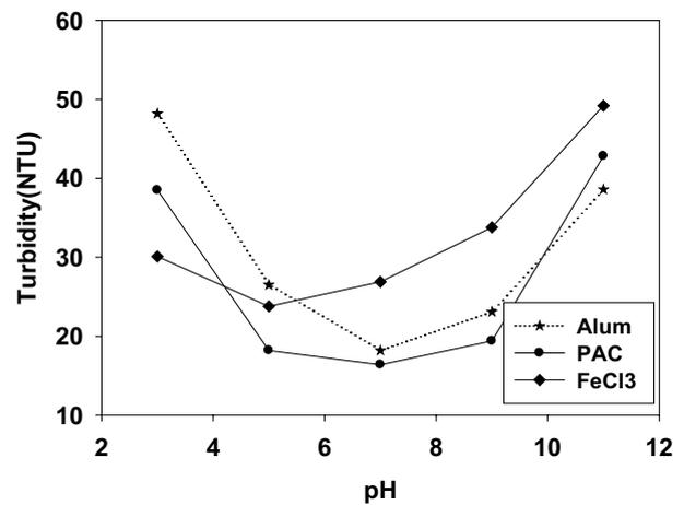
Fig. 1. Result of preceding research to determine optimum pH value.
