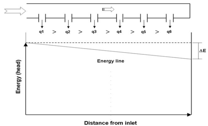
Fig. 2. Energy line grade of an open-type distribution channel (top view).
