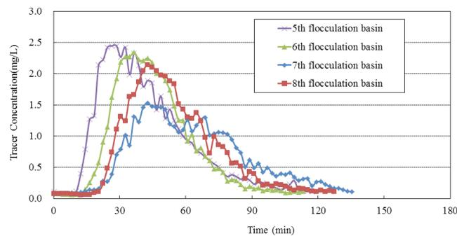
Fig. 7. Results of the tracer tests for the 5th to 8th flocculation basins.
