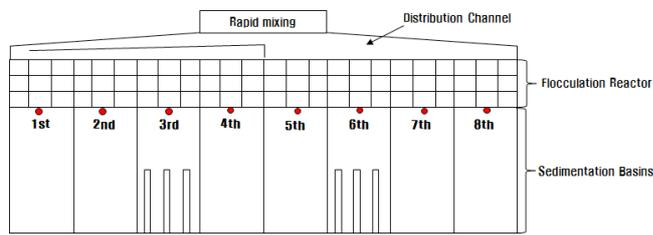
Fig. 1. Rapid mixing, distribution channel, and flocculation and sedimentation basins (top view).
