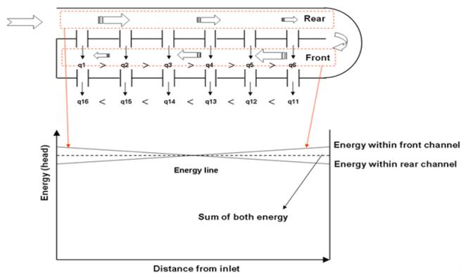
Fig. 3. Energy line grade of a double-baffled-type distribution channel (top view).
