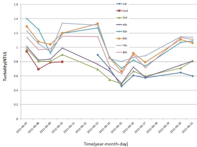
Fig. 8. Results of the turbidity measurements from the eight sedimentation basins.
