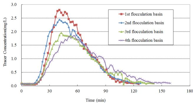
Fig. 6. Results of the tracer tests for the 1st to 4th flocculation basins.
