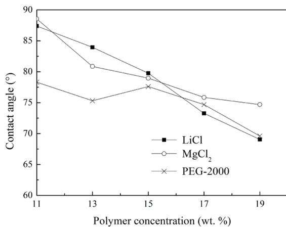
Fig. 8. Effects of polymer concentration on contact flux with different additive.
