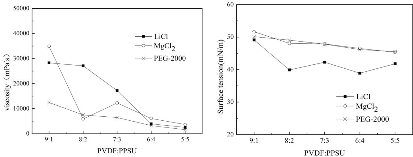
Fig. 3. Effects of PVDF/PPSU blend ratio on viscosity and surface tension with different additive.
