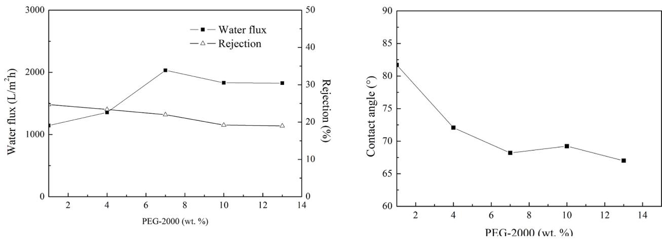
Fig. 10. Effects of additive concentration on water flux and rejection (PEG-2000).
