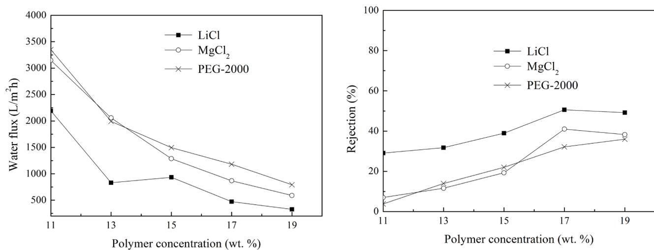
Fig. 7. Effects of polymer concentration on water flux and rejection with different additive.
