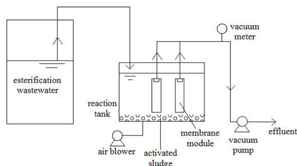
Fig. 1. Schematic drawing of MBR.
