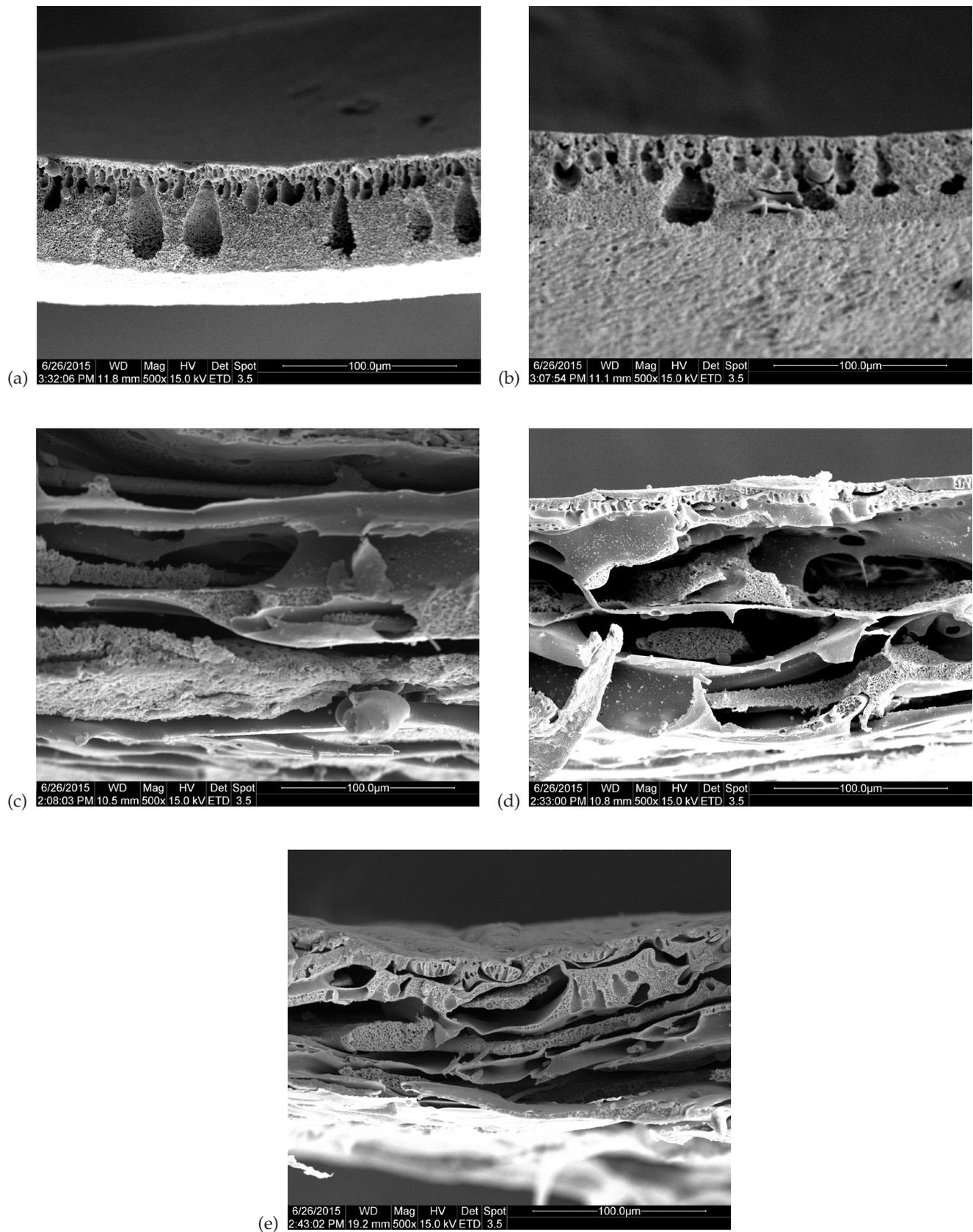
Fig. 2. Morphologies of PVDF/PPSU blending membrane.
