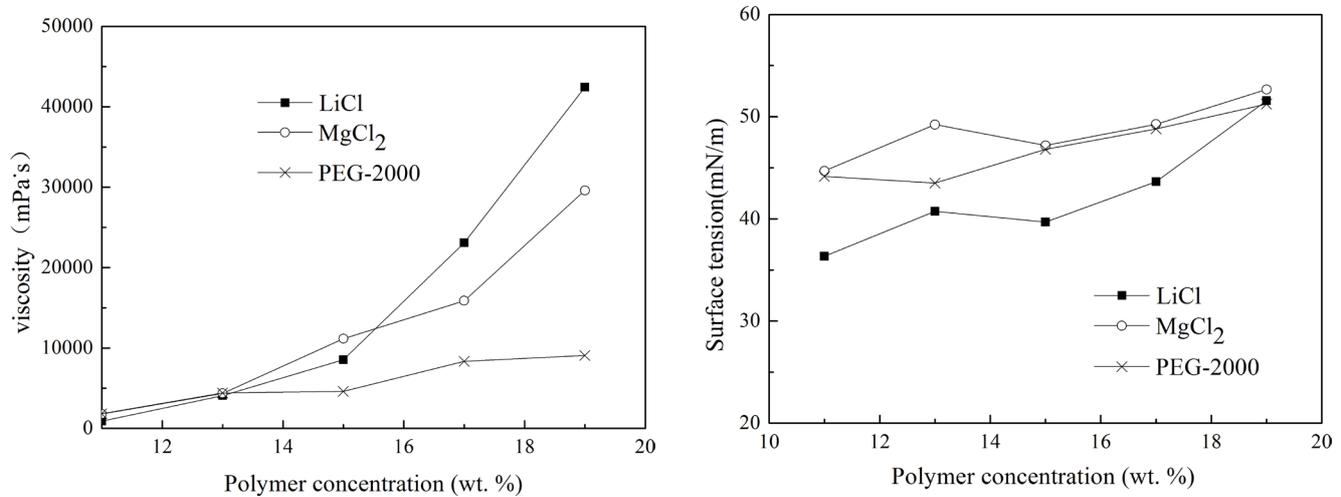
Fig. 6. Effects of polymer concentration on viscosity and surface tension with different additive.
