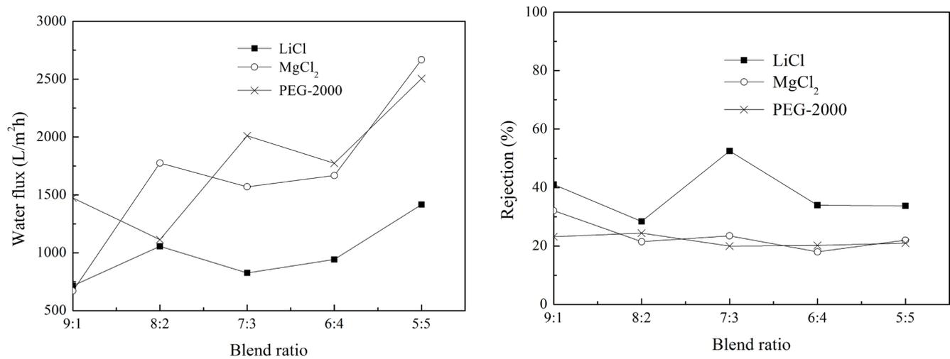
Fig. 4. Effects of PVDF/PPSU blend ratio on water flux and rejection with different additive.
