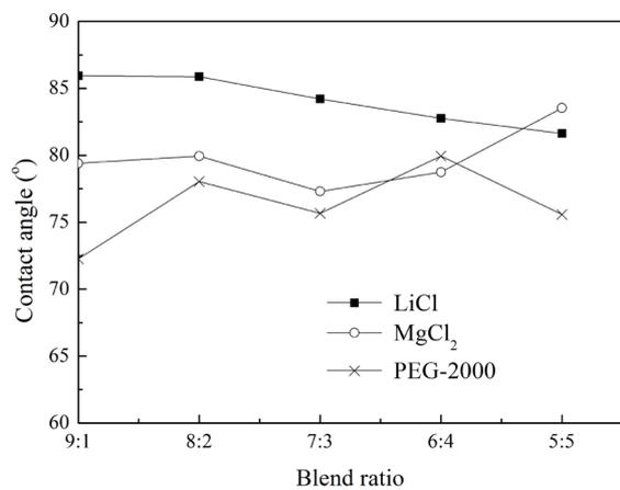
Fig. 5. Effects of PVDF/PPSU blend ratio on contact angle with different additive.
