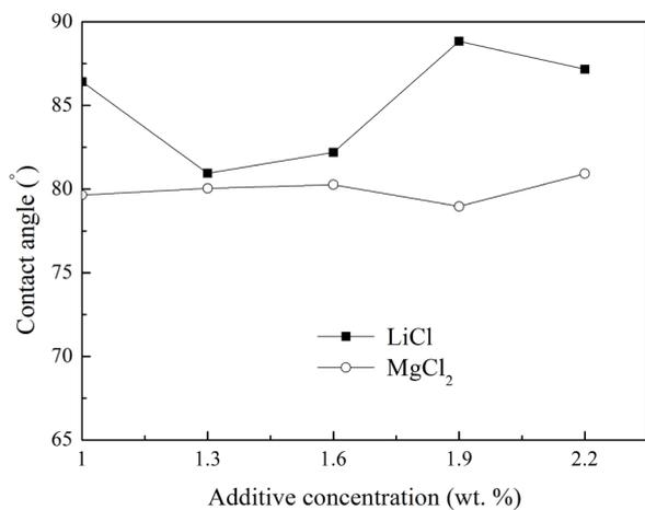
Fig. 11. Effects of additive concentration on contact angle with different additive.
