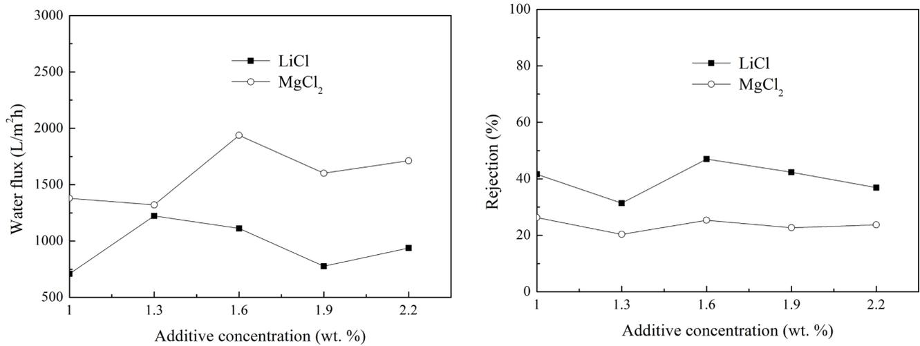
Fig. 9. Effects of additive concentration on water flux and rejection with different additive (LiCl and MgCl<sub>2</sub>).
