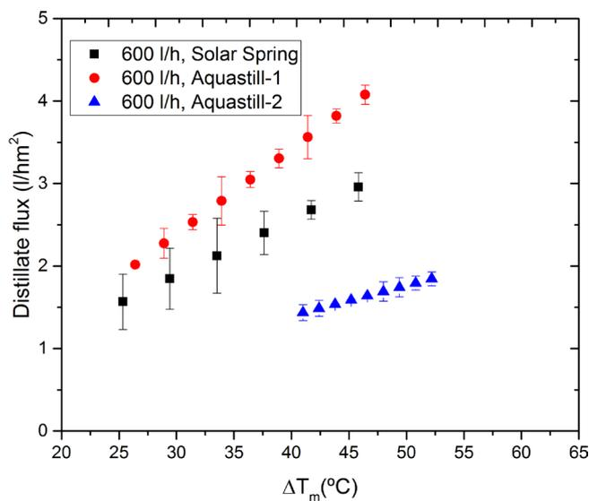
Fig. 6. Distillate flux (l h<sup>-1</sup>·m<sup>-2</sup>) as a function of the logarithmic mean temperature difference for the three modules for feed flow rate of 600 l h<sup>-1</sup>.
