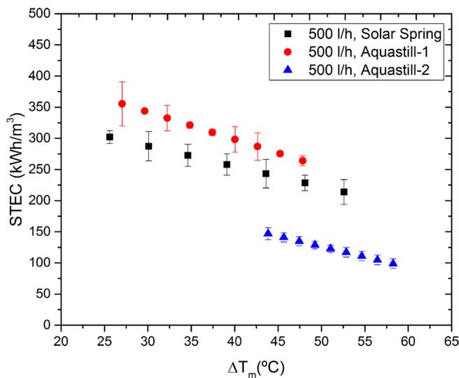
Fig. 8. Specific thermal energy consumption as a function of the logarithmic mean temperature difference for the three modules for feed flow rate of 500 l h<sup>-1</sup>.
