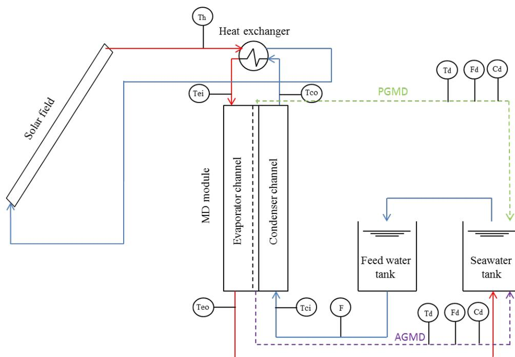
Fig. 3. Schematic diagram of the experimental set up.
