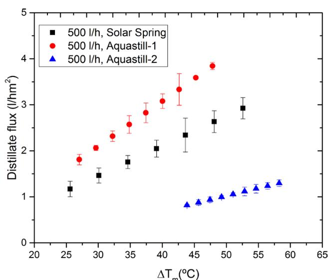
Fig. 5. Distillate flux as a function of the logarithmic mean temperature difference for the three modules for feed flow rate of 500 l h<sup>-1</sup>.
