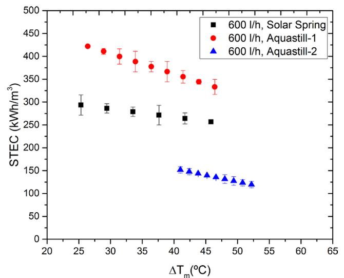
Fig. 9. Specific thermal energy consumption as a function of the logarithmic mean temperature difference for the three modules for feed flow rate of 600 l h<sup>-1</sup>.
