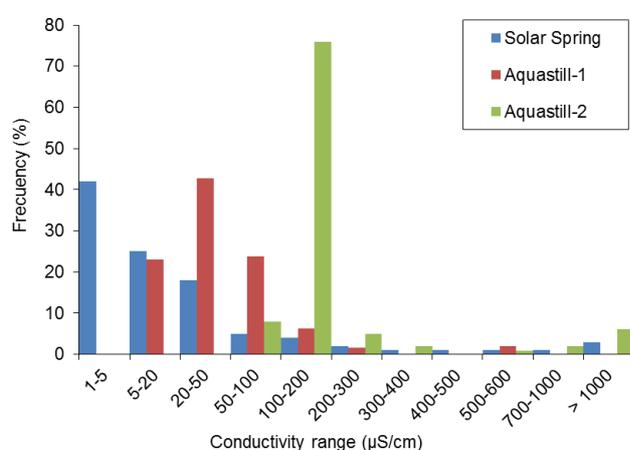
Fig. 10. Frequency distribution of the values of distillate conductivity measured for the Solar Spring, Aquastill-1 and Aquastill-2 modules.
