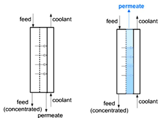
Fig. 2. AGMD (left) and PGMD (right) configurations.
