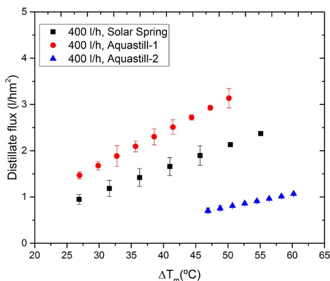
Fig. 4. Distillate flux as a function of the logarithmic mean temperature difference for the three modules for feed flow rate of 400 l h<sup>-1</sup>.
