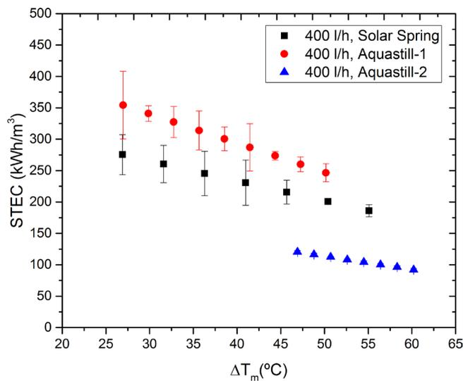
Fig. 7. Specific thermal energy consumption as a function of the logarithmic mean temperature difference for the three modules for feed flow rate of 400 l h<sup>-1</sup>.
