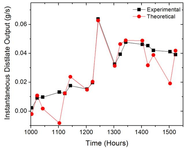
Fig. 6. The experimentally measured (squares) and theoretically predicted (circles) instantaneous distillate output.
