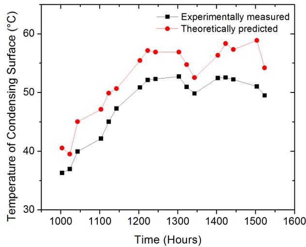
Fig. 5. The experimentally measured (squares) and theoretically predicted (circles) condensing surface temperature of the double exposure single basin solar still.
