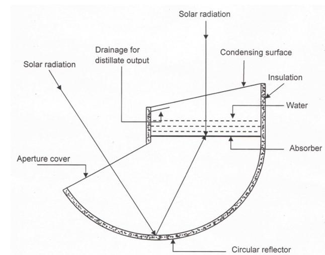
Fig. 2. Schematic diagram of a double exposure basin solar still showing solar radiation reaching the absorber from top and the bottom.
