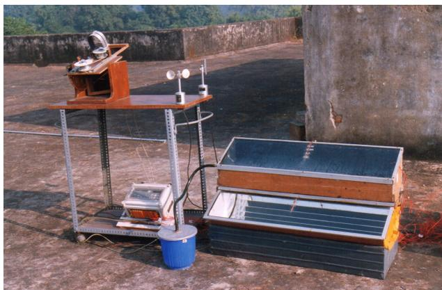
Fig. 1. A double exposure single basin solar still put on experiment.
