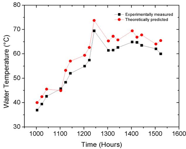
Fig. 4. Experimentally measured (squares) and theoretically predicted (circles) water temperatures of the double exposure single basin solar still.
