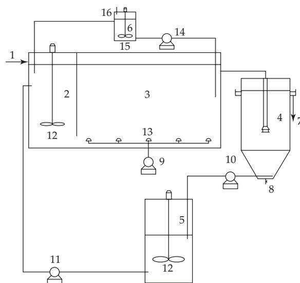
Fig. 2. Experimental device of the A-OSA process.
