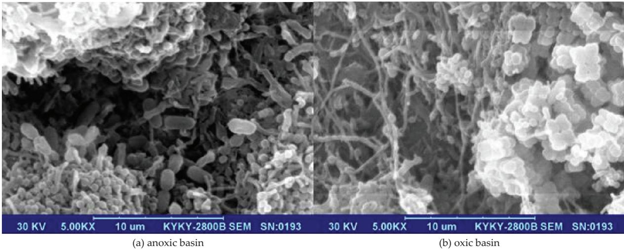
Fig. 7. SEM observations of the microorganism morphologies in HS-A-OSA process.
