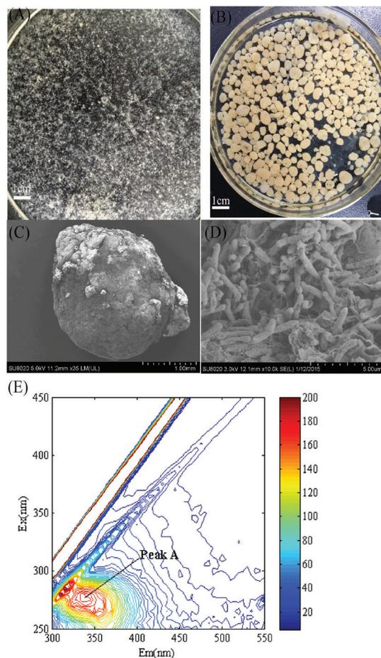
Fig. 2. Images illustrating the reaction components: (A) Seed sludge, (B) Mature aerobic granular sludge, (C) Low-magnification SEM image of AGS, (D) SEM image of a granule, and (E) EEM fluorescence spectrum for AGS-EPS.
