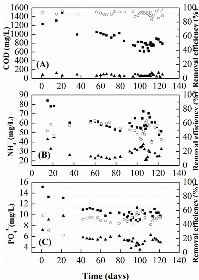
Fig. 1. Operating profiles of the SBR: (A) COD, (B) NH<sub>4</sub><sup>+</sup>-N, and (C) PO<sub>4</sub><sup>3--P</sup> concentrations. Influent (■), effluent (▲), and removal efficiency (○) are shown.
