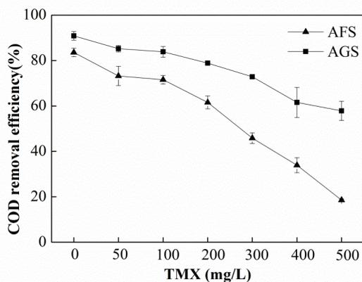
Fig. 3. COD removal efficiency of AFS and AGS during the treatment of synthetic wastewater in the presence of TMX.
