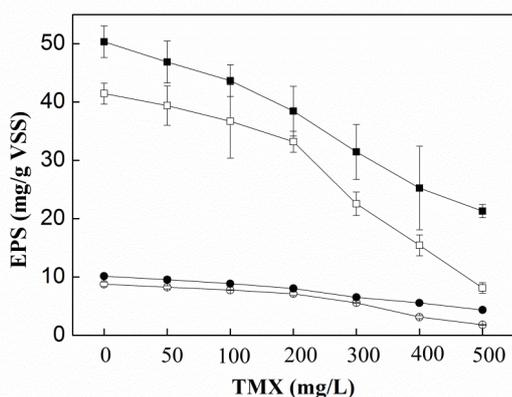
Fig. 4. Variations in EPS content during the experimental process. Profiles of PN and PS are shown as follows: PN of AGS (■) and AFS (□), PS of AGS (●) and AFS (○).
