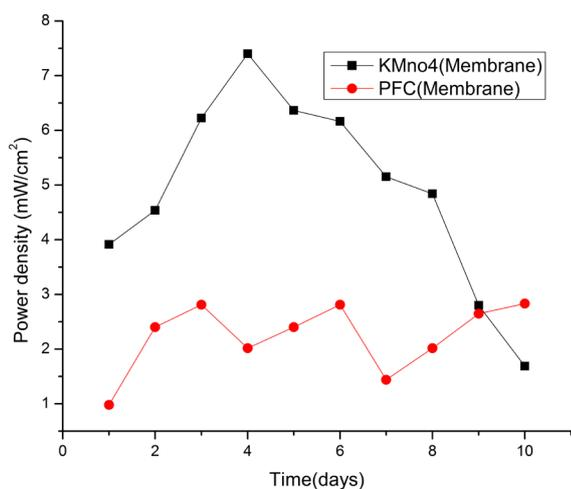
Fig. 4. Comparison of Power density production with potassium permanganate and potassium ferricyanide in PEM-MFC.
