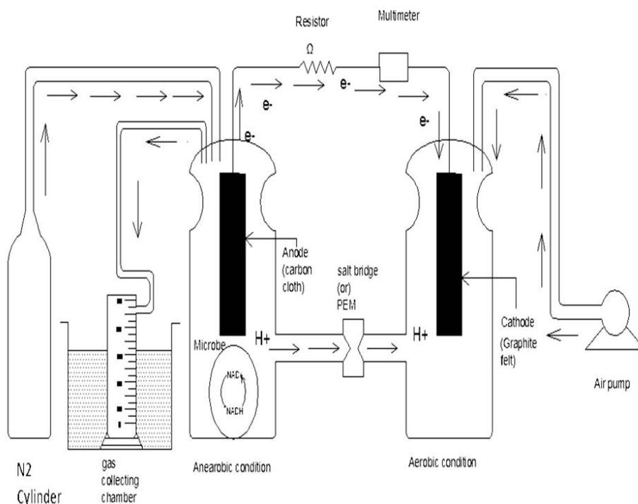
Fig. 1. Schematic of double chambered microbial fuel cell reactor.
