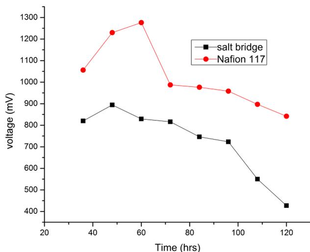
Fig. 2. Comparison of voltage production in PEM-MFC and salt bridge.
