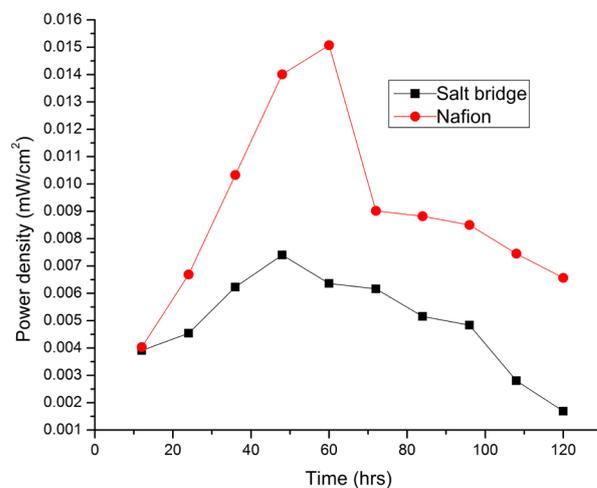
Fig. 3. Comparison of Power density production in PEM-MFC and salt bridge-MFC.
