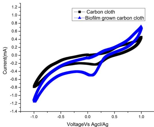
Fig. 10. Cyclic voltammetry of bare carbon electrode compared with biofilm formed electrode.
