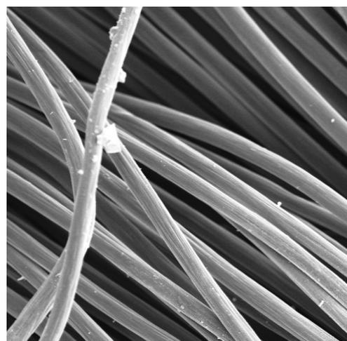
Fig. 6. SEM image of bare carbon cloth.
