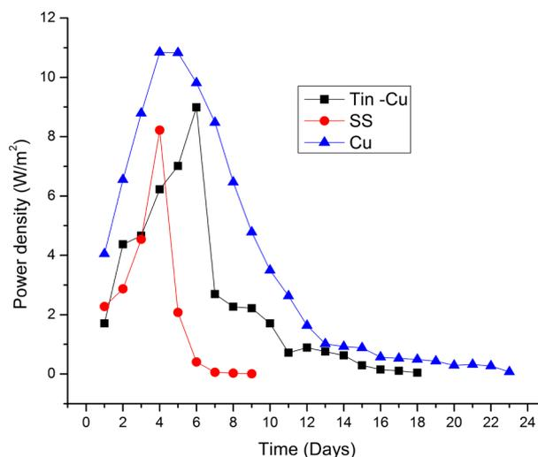
Fig. 5. Comparison chart between stainless steel, copper and tin coated copper wire.
