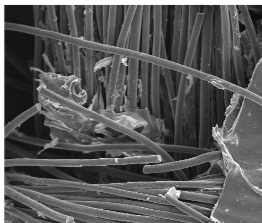
Fig. 7. SEM image of biofilm formed carbon cloth.
