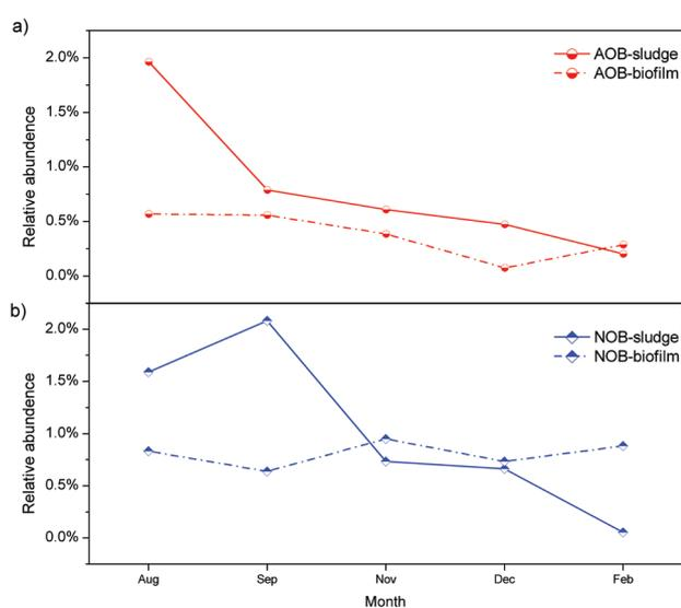
Fig. 4. Shift of nitrifying bacteria abundance in sludge and biofilm: (a) AOB and (b) NOB.
