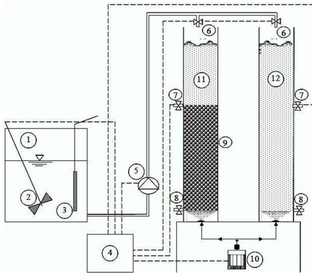
Fig. 1. Schematics of SBR and FBSBR.
