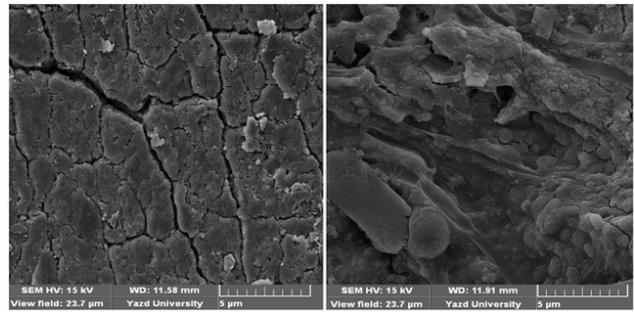
Fig. 9. SEM images of a sample of virgin surfaces of WTCs (left) and WTCs after biofilm formation (right).
