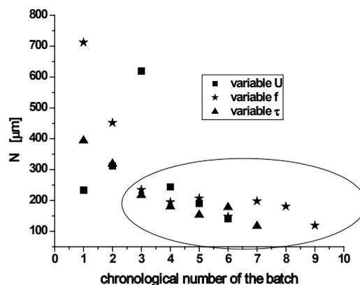
Fig. 9. Changes in polymer bulge size in microcapsule batches obtained with variable  $U$ ,  $f$  and  $\tau$ .
