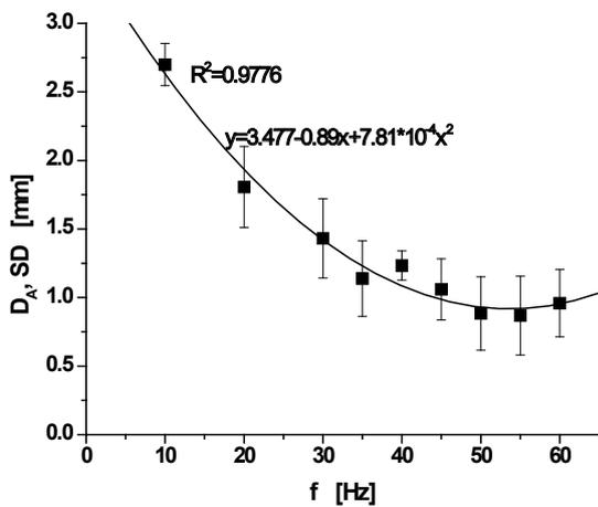
Fig. 3. Relation between electric impulse frequency  $f$  and average microcapsule diameter  $D_A$ .
