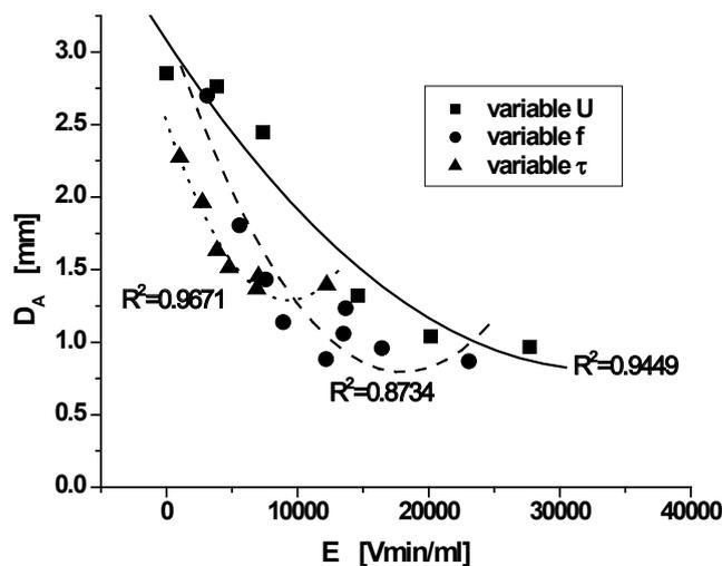
Fig. 7. Changes in average AGP microcapsule diameter  $D_A$  in the series with variable voltage U (continuous line), electric impulse frequency  $f$  (dashed line) and impulse duration  $\tau$  (dotted line).
