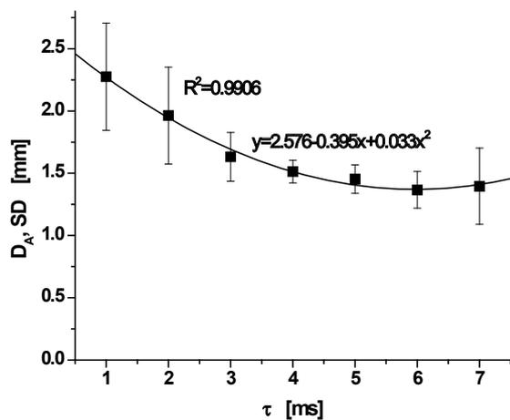
Fig. 5. Changes in average microcapsule diameter  $D_A$  as a function of changes in electric impulse duration  $\tau$ .
