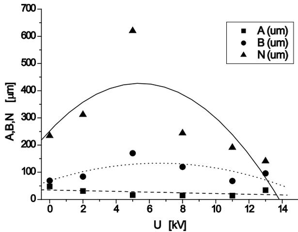
Fig. 2. Changes in microcapsule structural parameters: A, B and N as a function of increasing electric voltage  $U$ .
