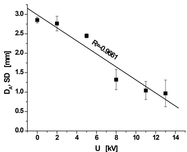
Fig. 1. Change in average microcapsule diameter  $D_A$  as a function of voltage  $U$  change.
