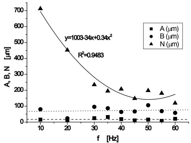
Fig. 4. Changes in membrane thickness of microcapsules obtained at different values of electric impulse frequency  $f$ .
