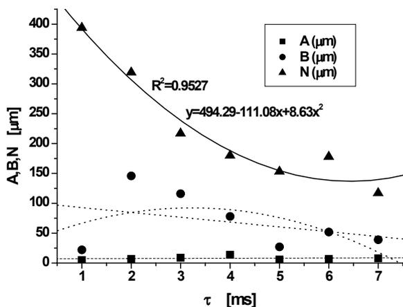
Fig. 6. Changes in membrane thickness of third-series microcapsules as a function of the duration of electric impulses  $\tau$ .
