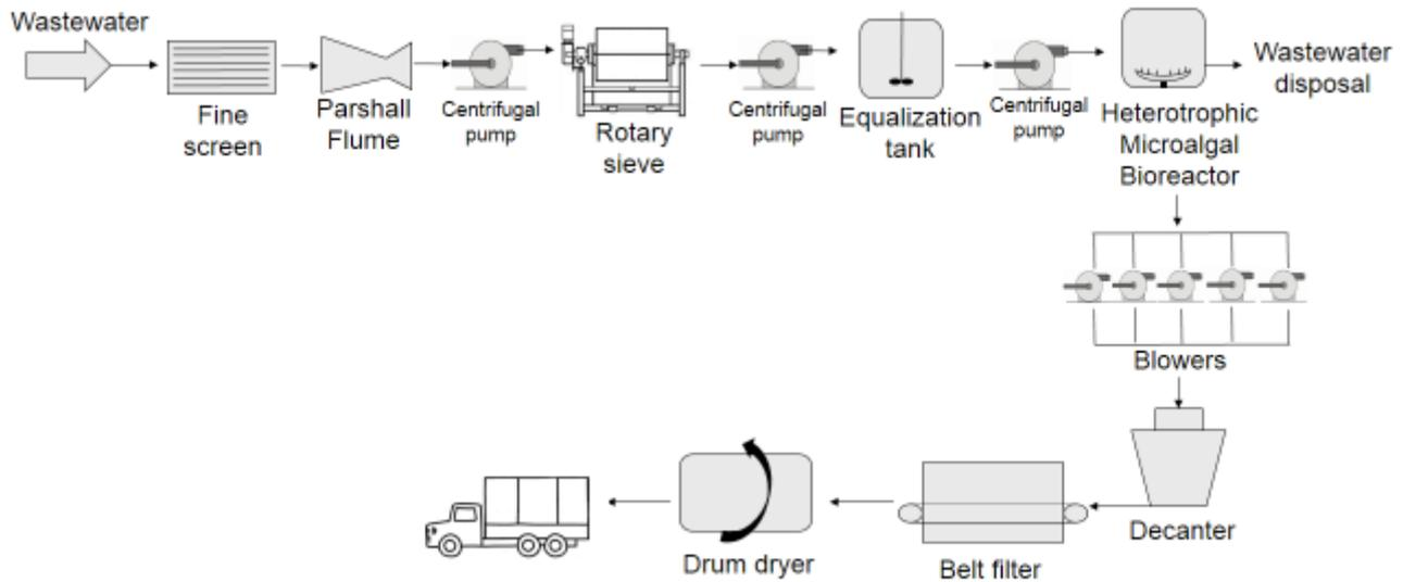
Fig. 1. Process flow diagram of the agroindustrial wastewater treatment.
