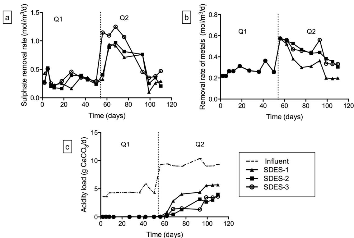
Fig. 4. Removal rates of (a) sulphate, (b) metals, and (c) specific acidity.
