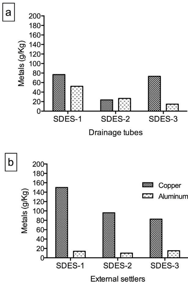
Fig. 6. Content of metals accumulated at the bottom of (a) the drainage tubes and in (b) the external settlers of SDES.
