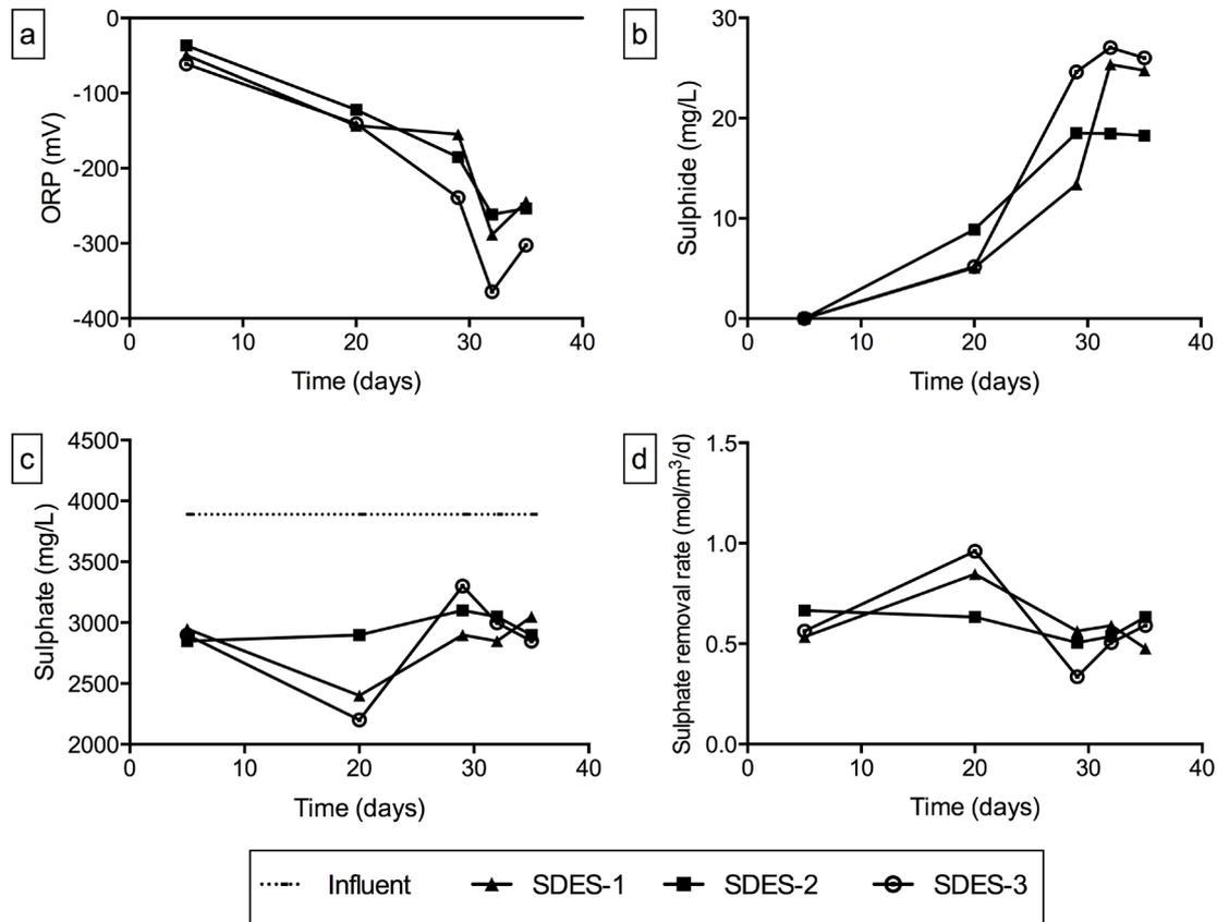
Fig. 2. Variations in (a) the ORP (mV); (b) the sulphide and (c) sulphate concentrations; and (d) the sulphate removal rate of three diffusive systems during feeding with sulphate solution (flow rate = 7.5 L/d).
