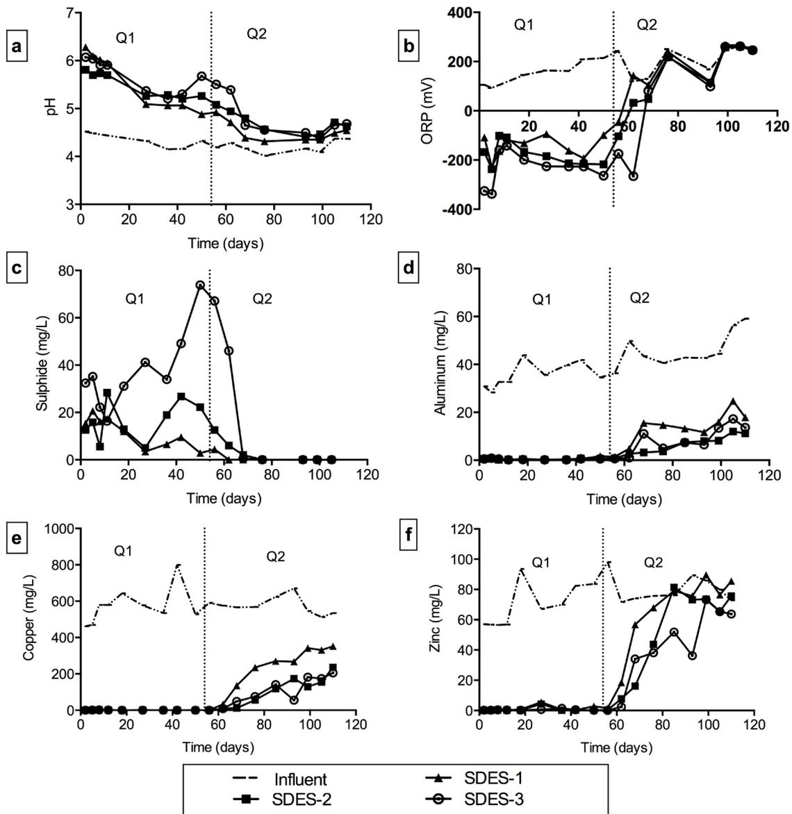
Fig. 3. Results of (a) pH; (b) ORP; (c) sulphide, (d) aluminium, (e) copper and (f) zinc concentrations in the effluent of three diffusive systems during operation with a synthetic AMD solution at two flow rates.
