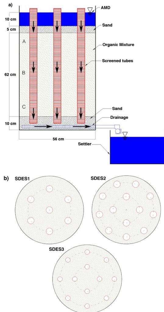
Fig. 1. (a) Side view of the diffusive exchange systems, (b) Representation of the characteristics of the diffusive systems (SDES). The vertical drainage tubes (conductive space) are represented as circles.
