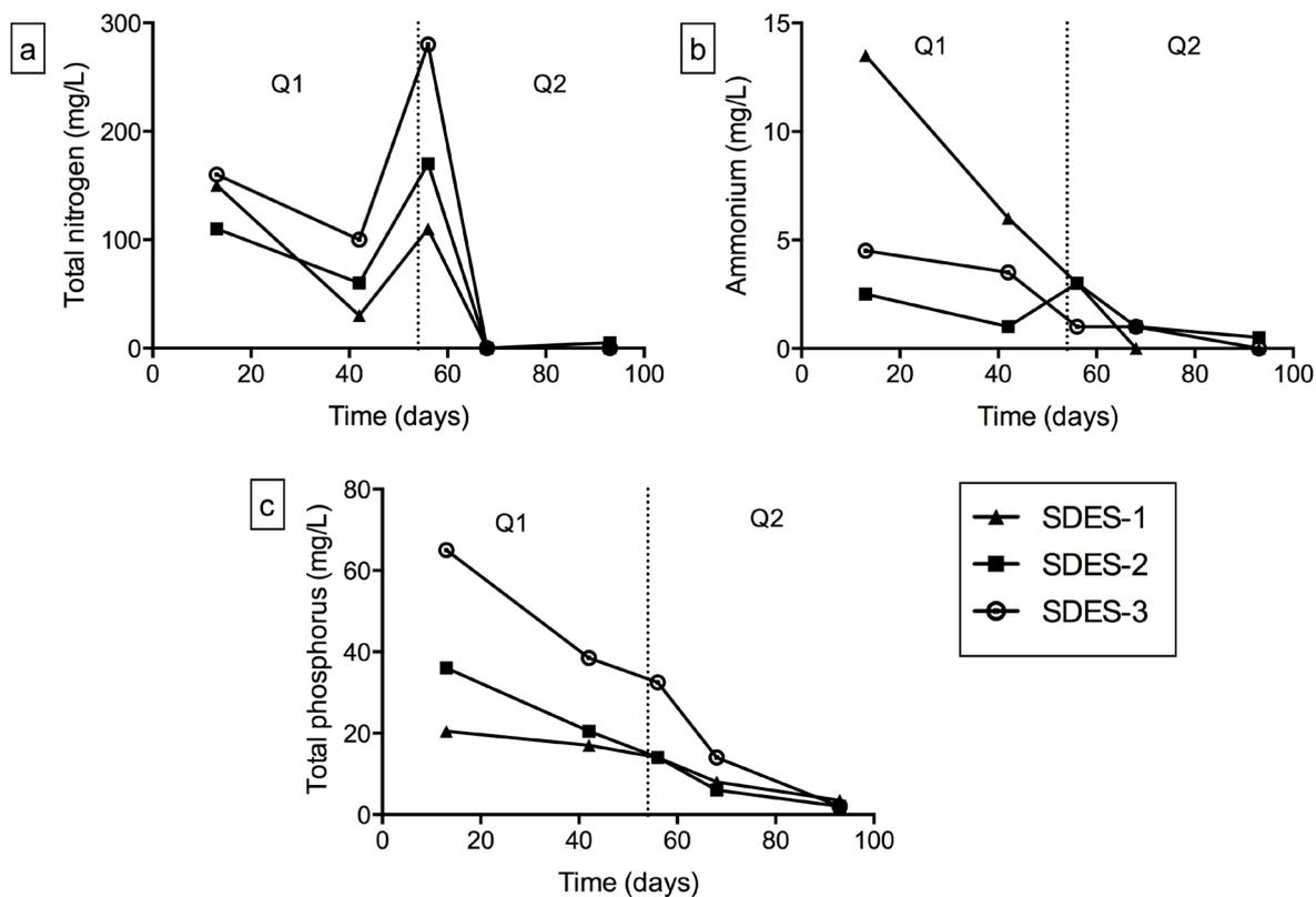
Fig. 5. Contents of (a) total N, (b) ammonium and (c) total P in the effluents of the diffusive systems.
