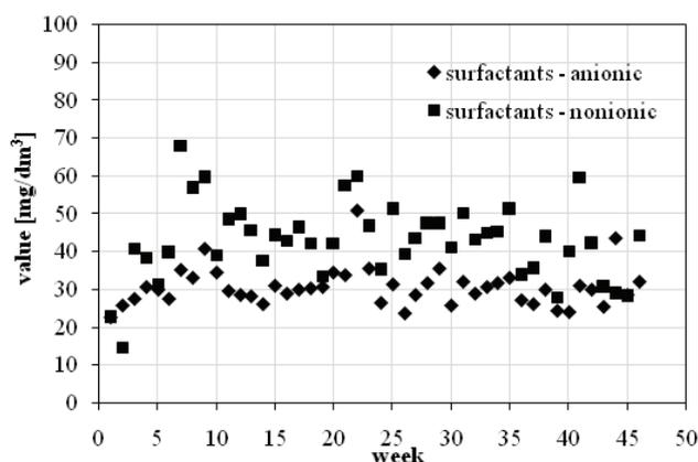
Fig. 2. Concentration of anionic and non-ionic surfactants in the raw laundry wastewater.
