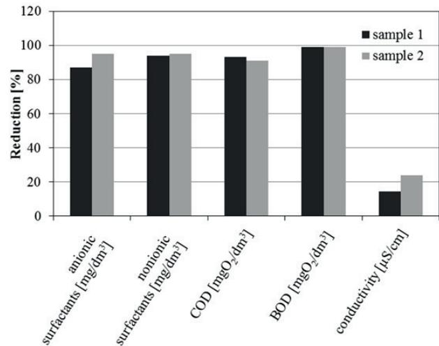
Fig. 7. Total efficiency of removal of organic and inorganic contaminants from laundry wastewater treated in pilot-scale MBR at 218 h (Sample 1) and 510 h (Sample 2).
