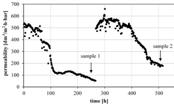
Fig. 6. Changes of the membrane permeability during 3 weeks of MBR operation.
