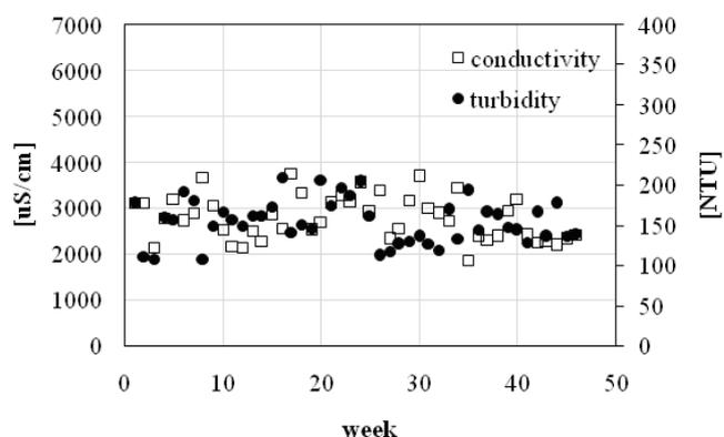
Fig. 4. Changes of conductivity and turbidity of raw laundry wastewater in time.
