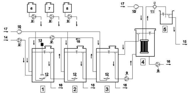
Fig. 1. A schematic diagram of the pilot scale MBR installation. Note: 1 – anoxic/oxic reactor, 2 – oxic reactor, 3 – oxic reactor, 4 – membrane unit, 5 – permeate tank, 6 – acid container, 7 – anti-foam container, 8 – nutrient container, 9 – peristaltic pump, 10 – blower, 11 – permeate pump, 12 – membrane diffuser, 13 – mixer, 14 – raw wastewater inflow, 15 – permeate outflow, 16 – excess sludge, 17 – air, 18 – recirculation of activated sludge.
