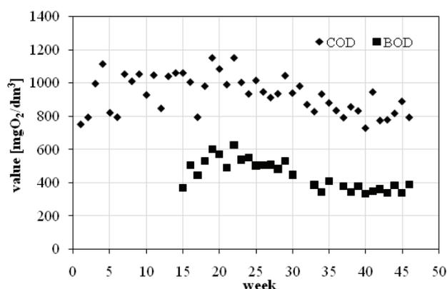
Fig. 3. Changes of COD and BOD of raw laundry wastewater with time.
