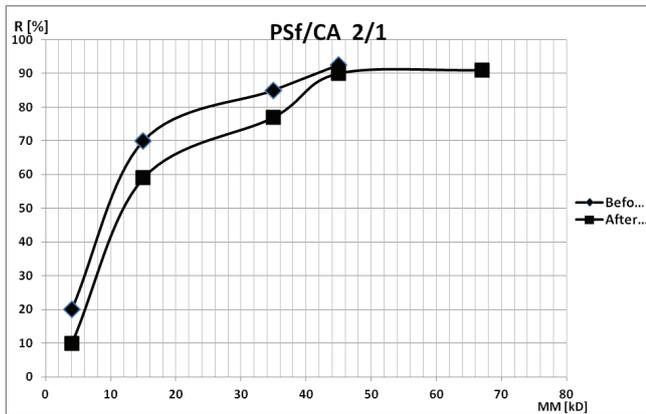
Fig. 2. Retention coefficients of different markers for PSf, PSf/CA-2/1 membranes before and after hydrolysis.
