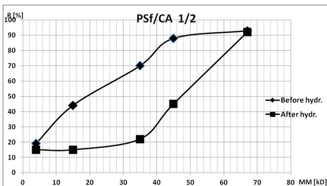
Fig. 4. Retention coefficients of different markers for PSf, PSf/CA-1/2 membranes before and after hydrolysis.
