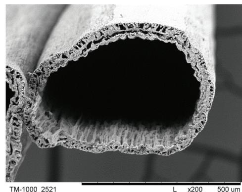
Fig. 19. Cross section of PSf/CA-1/3 membranes after hydrolysis.
