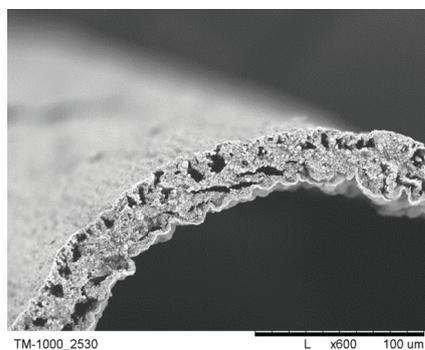
Fig. 21. Part of cross section of PSf/CA-1/3 membranes after hydrolysis.
