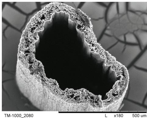
Fig. 15. Cross section of PSf/CA-1/2 membranes after hydrolysis.
