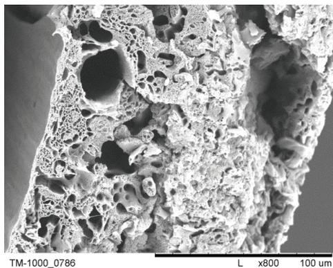
Fig. 16. Part of cross section of PSf/CA-1/2 membranes before hydrolysis.
