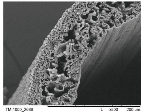
Fig. 17. Part of cross section of PSf/CA-1/2 membranes after hydrolysis.
