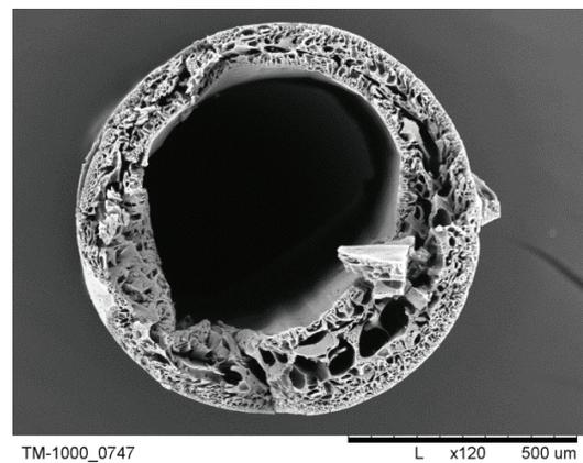
Fig. 6. Cross section of PSf/CA-2/1 membranes before hydrolysis.
