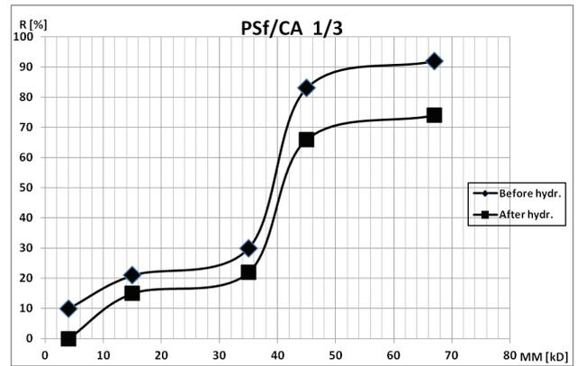
Fig. 5. Retention coefficients for different markers for PSf, PSf/CA-1/3 membranes before and after hydrolysis.
