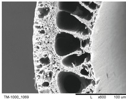
Fig. 20. Part of cross section of PSf/CA-1/3 membranes before hydrolysis.
