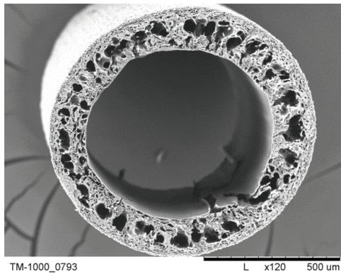
Fig. 14. Cross section of PSf/CA-1/2 membranes before hydrolysis.
