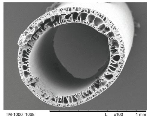
Fig. 18. Cross section of PSf/CA-1/3 membranes before hydrolysis.
