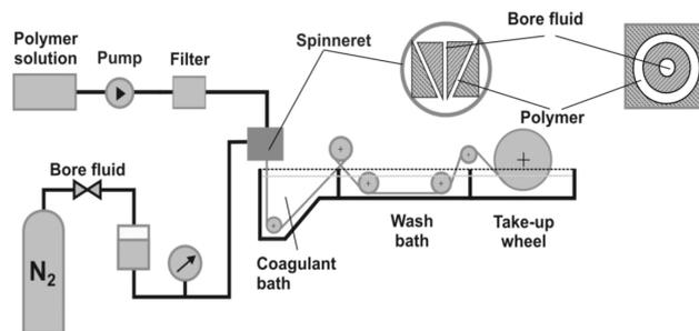
Fig. 1. Schematic diagram of the spinning process for capillary membranes preparation.
