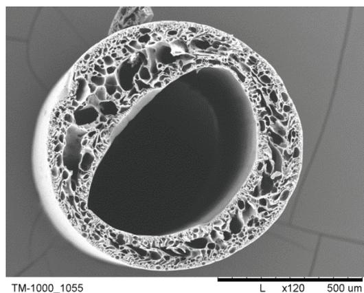
Fig. 7. Cross section of PSf/CA-2/1 membranes after hydrolysis.
