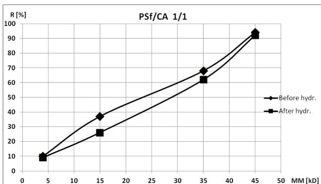
Fig. 3. Retention coefficients of different markers for PSf, PSf/CA-1/1 membranes before and after hydrolysis.
