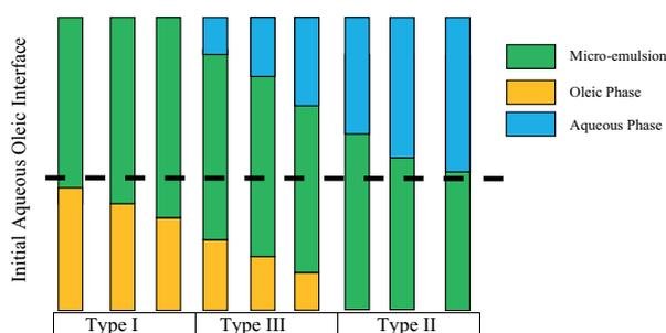
Fig. 1. Phase behaviour of equal volumes of surfactant solution and oil mixed in test tubes (after allowing time for equilibrium). At low salinity (Type I), a micro-emulsion and excess oil phase exist. At high salinity (Type II), a micro-emulsion and excess water form. All three phases (Type III) exist at intermediate salinities (Kostarelos et al. [6]).
