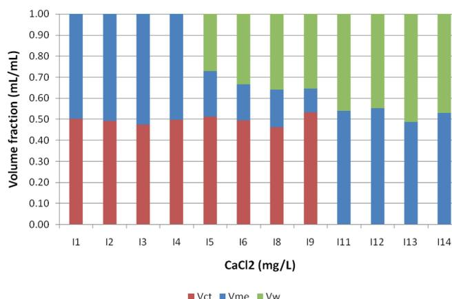
Fig. 3. Surfactant phase behaviour diagram for CaCl<sub>2</sub> (Winsor Type I 0–600 mg/L, II 2,500–10,000 mg/L, III 1,000–1,900 mg/L system) (Vct: coal tar volume, Vme: micro-emulsion volume, Vw: water volume).
