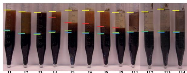
Fig. 2. Final results for the phase behaviour test (60°C ± 1°C) using as surfactant (2 mL): Alf 123 (3%) and MA 80-I (1%) (blue line indicates the initial interface, yellow line indicates the phase C, red line indicates the phase B and green line indicates the phase A).
