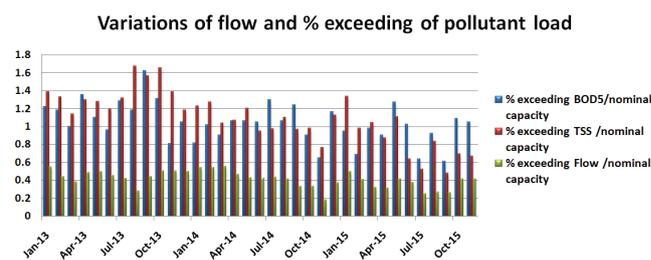
Fig. 3. Variations of flow and % exceeding of BOD<sub>5</sub> and TSS relative to the nominal capacity.
