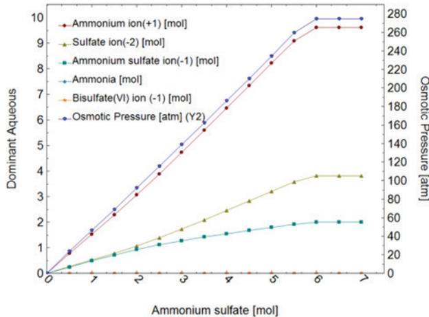
Fig. 6. Species generated and osmotic pressure of ammonium sulphate. Analysis carried out using OLI stream Analyzer 9.1 at 25°C temperature and 1 atm pressure [37].
