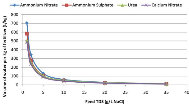
Fig. 10. Variation of water extraction capacities of the draw solutes by FO process at different feed TDS using different draw solutes.
