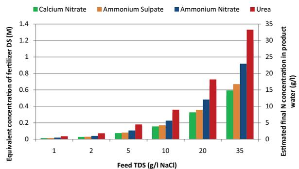
Fig. 11. Equivalent concentration of fertilizer DS and estimated final N concentration in product water for different feed TDS concentrations.
