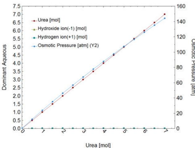
Fig. 7. Species formed and osmotic pressure of urea. Analysis carried out using OLI stream Analyzer 9.1 at 25°C temperature and 1 atm pressure [37].
