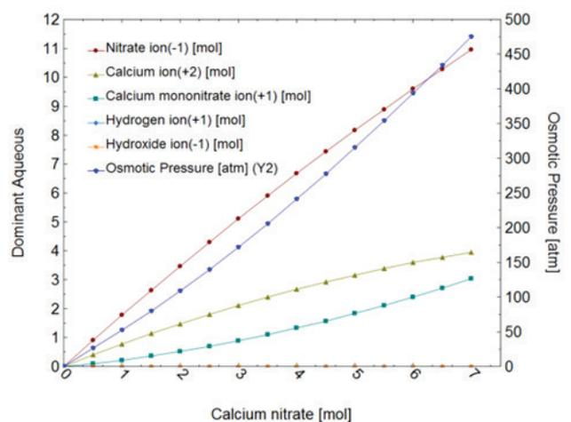
Fig. 9. Species formed and osmotic pressure of calcium nitrate. Analysis carried out using OLI Stream Analyzer 9.1 at 25°C temperature and 1 atm pressure [37].
