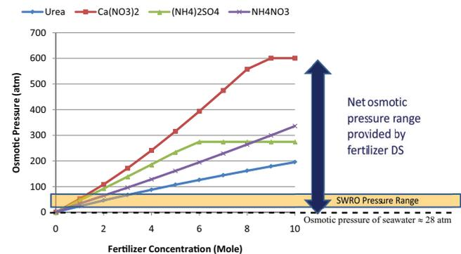
Fig. 5. Osmotic pressure of different nitrogenous fertilizers DS at 25°C analyzed using OLI Stream Analyzer 9.1.
