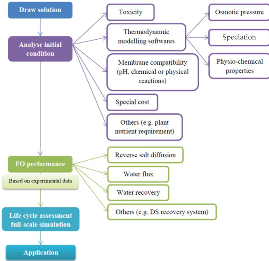
Fig. 1. Flow diagram for selecting a suitable DS in FO process [30].
