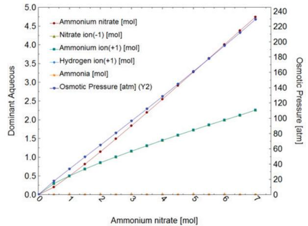
Fig. 8. Species formed and osmotic pressure of ammonium nitrate. Analysis carried out using OLI stream Analyzer 9.1 at 25°C temperature and 1 atm pressure [37].
