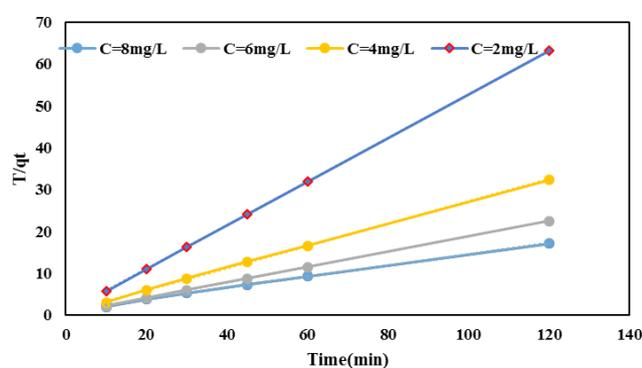
Fig. 9. Modeling the pseudo-second-order kinetic for fluoride adsorption using alumina nanoparticle/MWCNTs.
