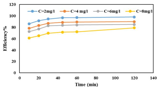
Fig. 4. The effect of contact time on fluoride adsorption by alumina nanoparticle/MWCNTs (adsorbent dose = 0.5 g/L, pH = 3).
