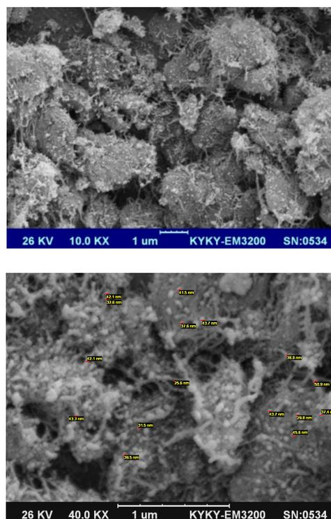
Fig. 2. SEM photograph of alumina nanoparticle on MWCNTs from a different angle.
