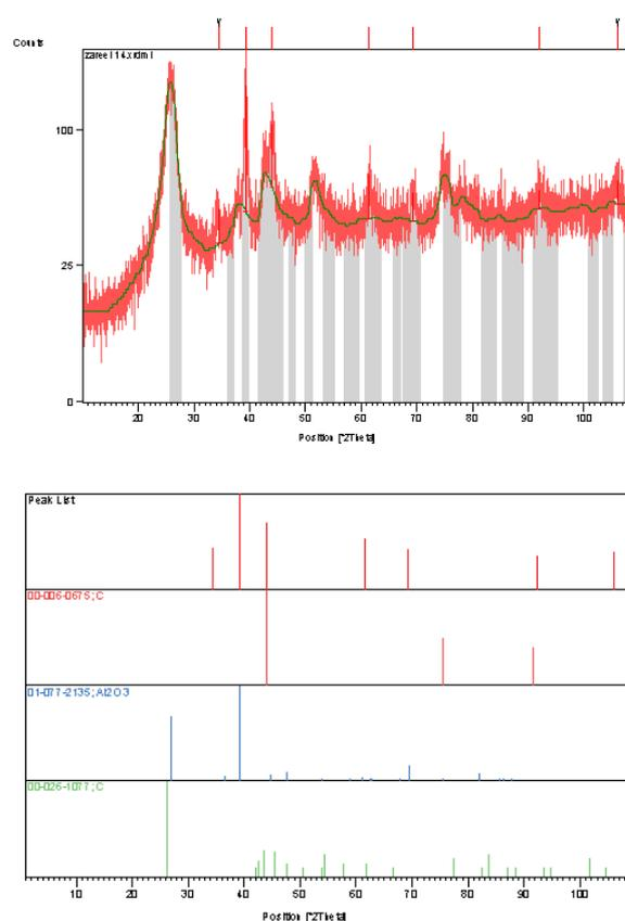
Fig. 3. XRD pattern of the alumina nanoparticle/MWCNTs.
