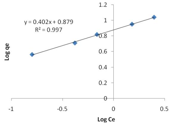
Fig. 8. Modeling the Freundlich adsorption isotherm for fluoride adsorption using alumina nanoparticle/MWCNTs.
