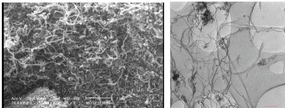
Fig. 1. (a) SEM and (b) TEM of a (MWCNTs).
