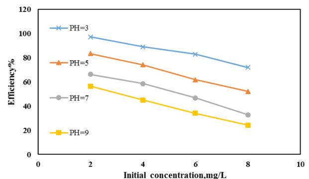
Fig. 6. Effect of pH on fluoride sorption by alumina nanoparticle/MWCNTs (sorbent dose = 0.5 g L<sup>-1</sup>; contact time = 60 min and different fluoride concentration).
