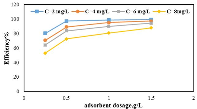
Fig. 7. Effect of adsorbent dose on fluoride sorption by alumina nanoparticle/MWCNTs (pH = 3 dose = 0.5 g/L, contact time = 60 min and different fluoride concentration).
