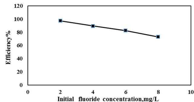
Fig. 5. Effect of initial concentration on fluoride adsorption by alumina nanoparticle/MWCNTs (adsorbent dose = 0.5 g/L, pH = 3).
