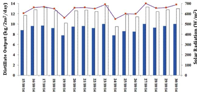
Fig. 10. Distillate outputs of 2 m<sup>2</sup> Carocell solar still, with versus without a heat exchanger.
