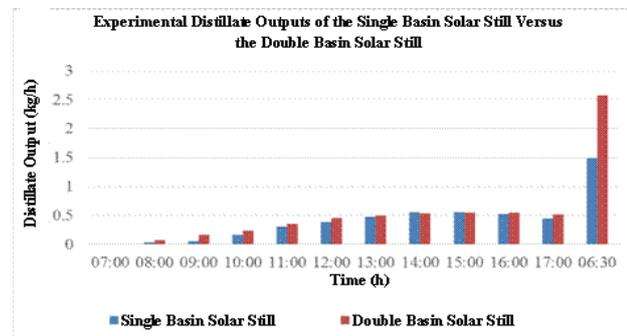
Fig. 9. Experimental distillate outputs of the single basin solar still versus the double basin solar still.
