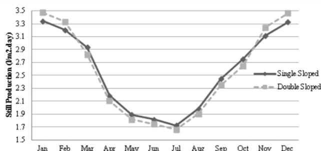
Fig. 3. The output of distilled water per month single roof and roof type double [12].
