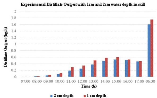
Fig. 4. Experimental distillate output with 1 cm and 2 cm water depth in the single basin solar still coupled with evacuated glass tubes [18].
