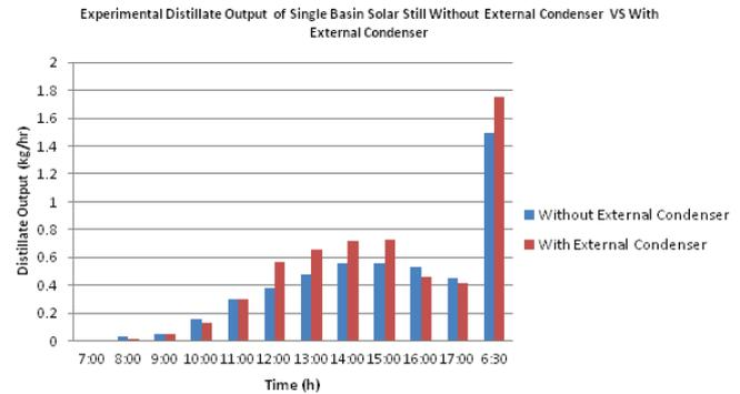
Fig. 13. Experimental distillate output of single basin solar still without external condenser versus with external condenser.
