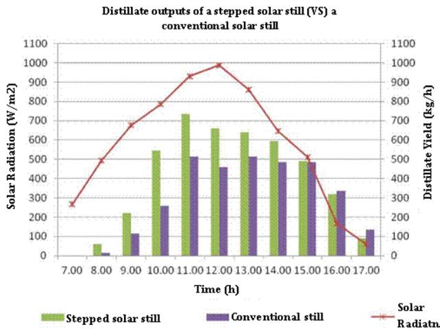
Fig. 11. Distillate outputs of a stepped solar still versus a conventional solar still.
