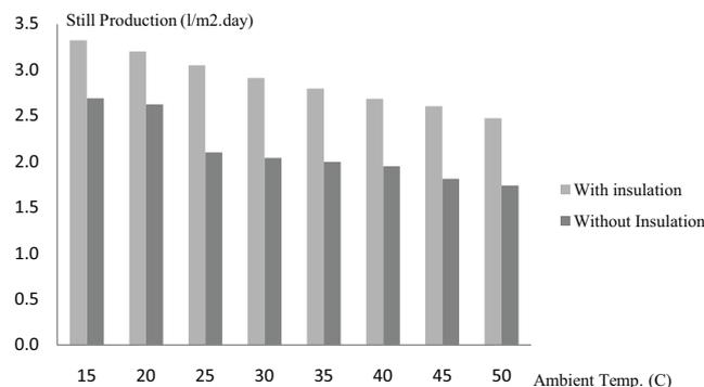
Fig. 2. Effect of temperature on the output of solar stills [12].
