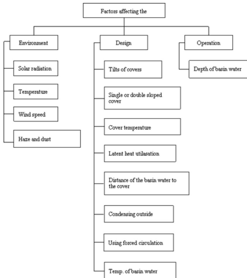
Fig. 1. Factors affecting the outputs of solar distillation systems.
