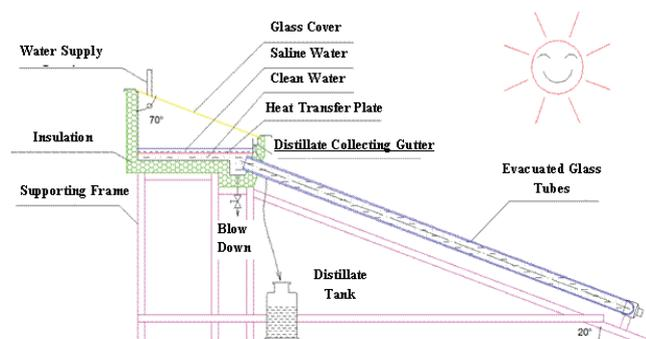
Fig. 7. Single basin solar still coupled with evacuated glass tubes.
