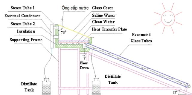
Fig. 12. Single basin solar still coupled with evacuated glass tubes and external condenser.
