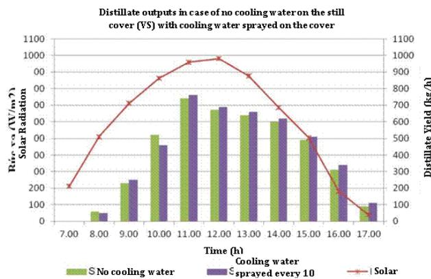
Fig. 6. Distillate outputs in case of no cooling water on the still cover (VS) with cooling water sprayed on the cover.
