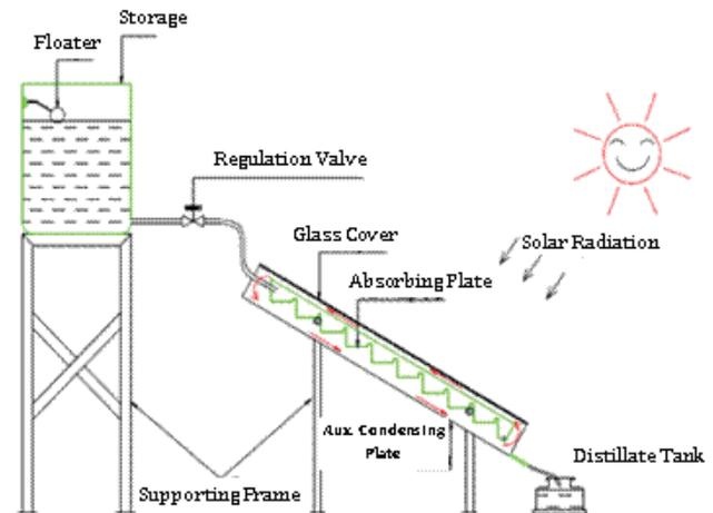
Fig. 5. The schematic diagram of the experimented stepped solar still [19].
