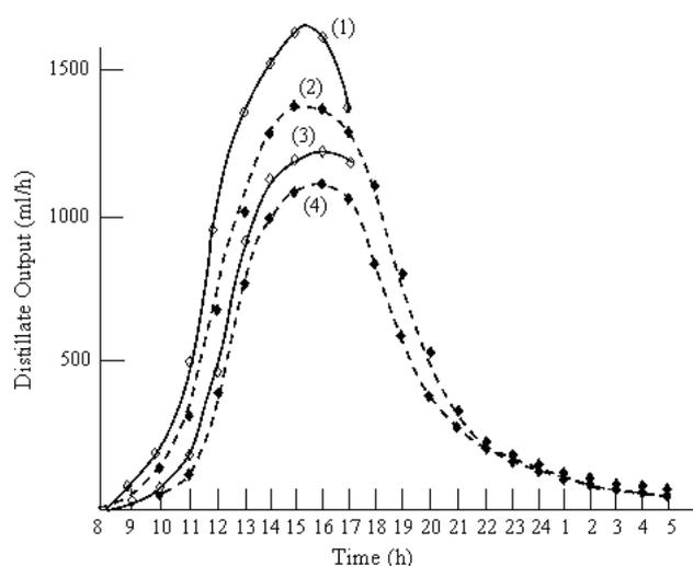
Fig. 15. The effect of forced convection in the device to produce distilled water. (1) Data empirical forced convection; (2) The data forced convection theory. (3) Data empirical natural convection; (4) Data natural convection theory.
