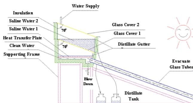
Fig. 8. Double basin solar still coupled with evacuated glass tubes.
