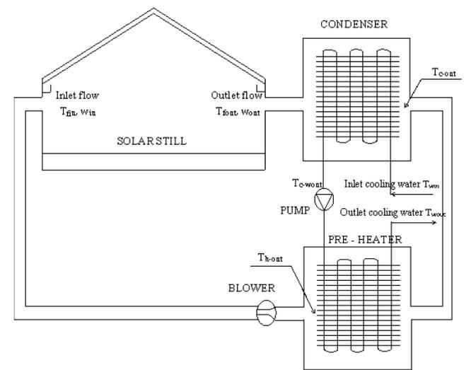
Fig. 14. Schematic diagram of a forced circulation solar still with enhanced water recovery.
