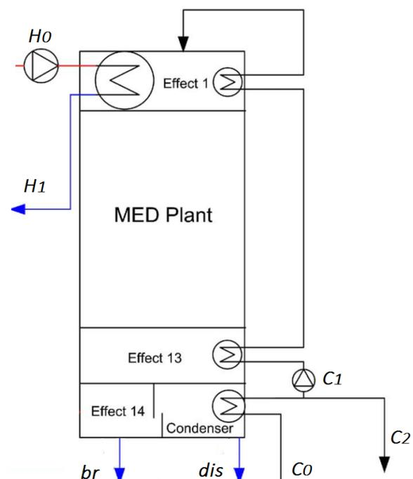
Fig. 1. MED plant unit scheme.
