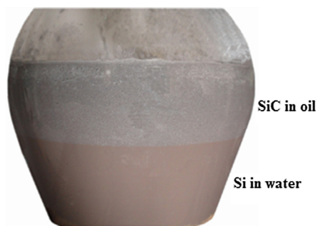
Fig. 1. A picture of phases in the separating funnel after settling for 10 min during recovering Si from wire saw slurry by liquid–liquid extraction, with kerosene as the oil. Slurry is wet oxidized, and {O} content is 1.7% by weight.
