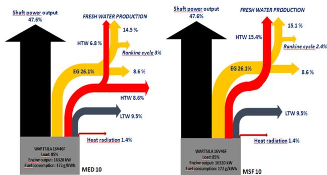
Fig. 7. Sankey Diagram of the dual purpose water/energy plant in case of MED and MSF.
