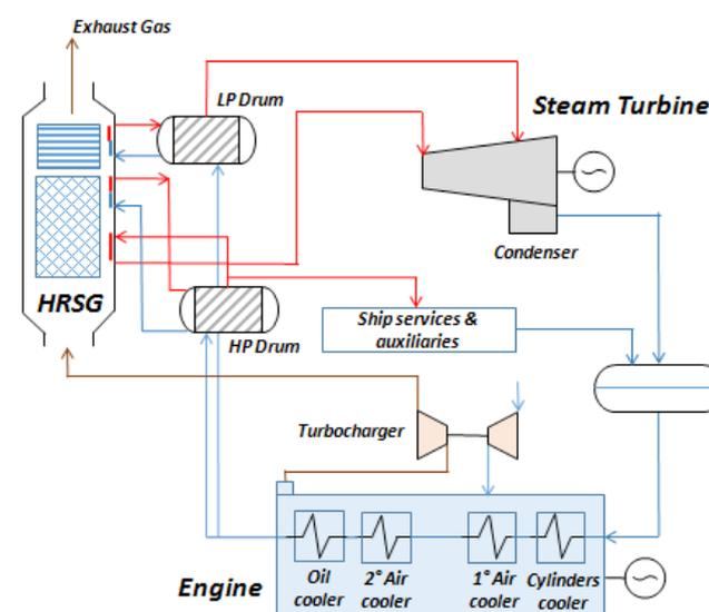
Fig. 1. Diesel Engine with HRSG and Steam Turbine for additional power generation.
