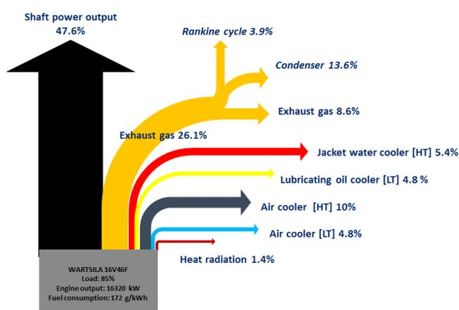
Fig. 2. Sankey diagram of the diesel engine with HRSG and additional power generation in steam cycle (see Fig. 1) (1.3 MW,  $\eta = 0.22$ ).
