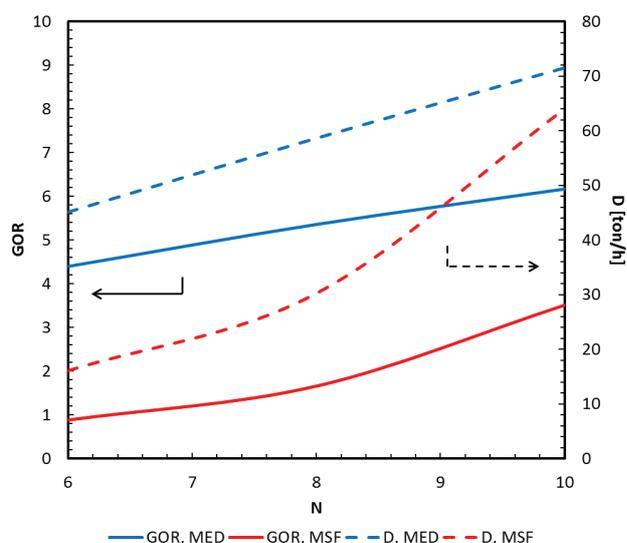
Fig. 6. GOR and Distillate for MED and MSF on-board application.
