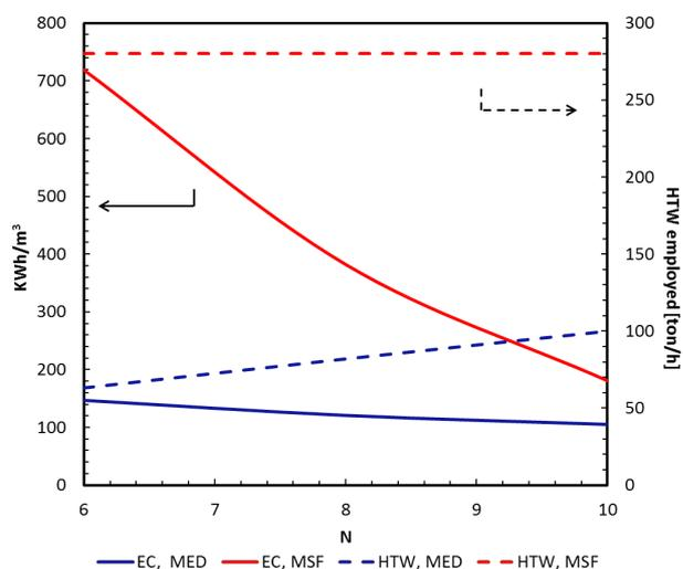
Fig. 5. Energy consumption (EC) and HTW reclaimed in MED and MSF application.
