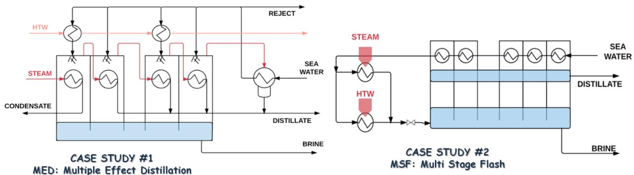
Fig. 4. Process schemes of the two thermal desalination plants analysed in the case studies.
