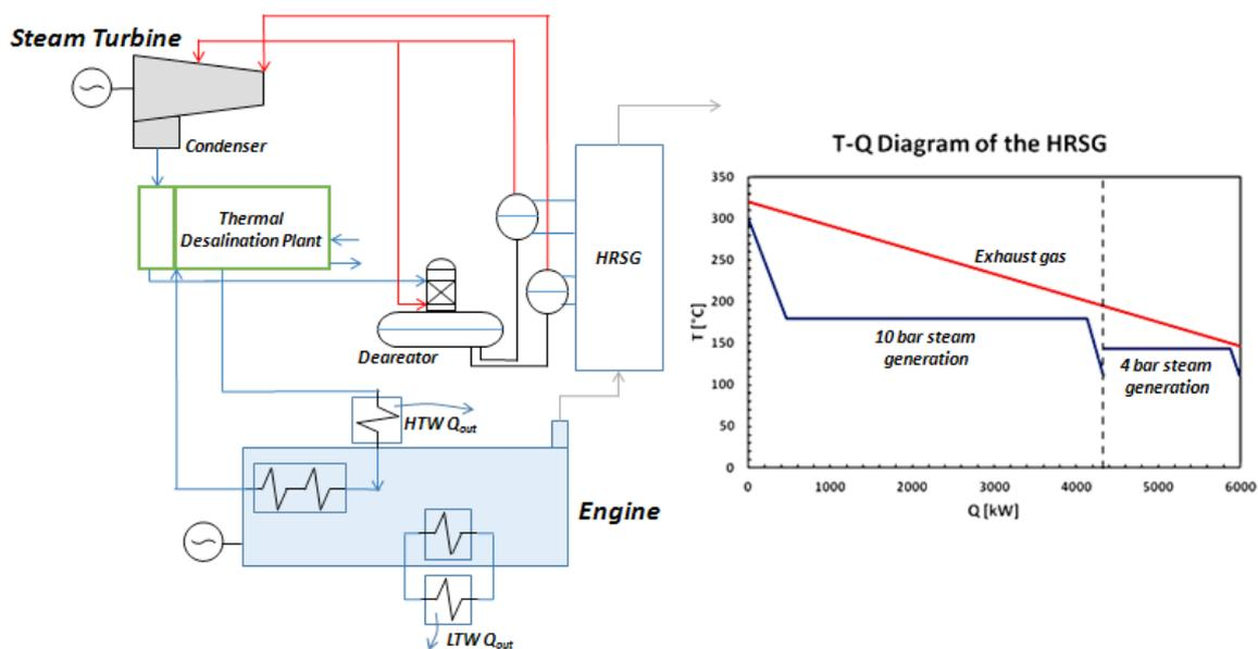
Fig. 3. Dual Purpose plant for on-ship desalination and electrical power production with temperature-duty diagram of the HRSG.
